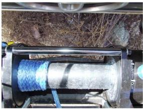
The Test - Winching a Land Rover Defender up a moderate slope. Testing involved a cycle of 90second pull time with a 60 second recovery period until the Defender had been pulled 30m up the hill. All stops and start times were
