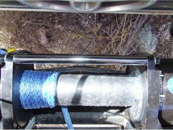
The Test - Winching a Land Rover Defender up a moderate slope. Testing involved a cycle of 90second pull time with a 60 second recovery period until the Defender had been pulled 30m up the hill. All stops and start times were accurately followed to ensure fair comparison and repeatability. Winching was started with 10 turns of rope on the winch drum. Winch and batteries were given a 10minute (timed) break before the test was repeated.
