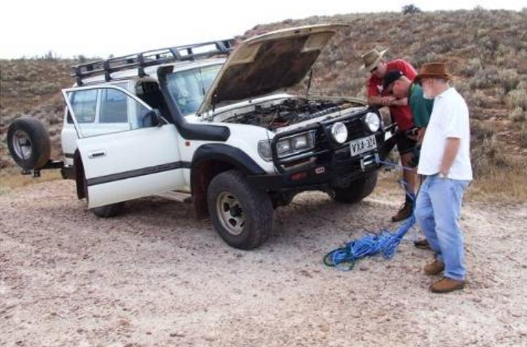
**Ironman 4x4 9500lb electric winch - installed in an 80series Landcruiser**
