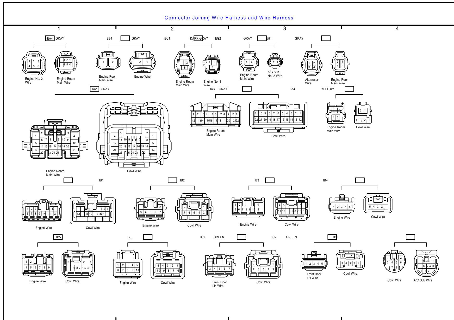
**HILUX****Connector Joining Wire Harness and Wire Harness**
