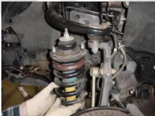
12. Position the new coilover onto the vehicle, sliding the top into the shock tower first. Install the top three nuts which hold the coilover to the shock tower finger tight. Install the lower shock bolt and nut. **You may need to pry down on the upper control arm in order to get the lower shock bolt installed.** Torque upper nuts and lower bolt/nut to manufacture specs.
