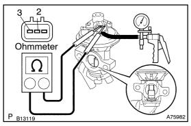
(2) Apply vacuum to the diaphragm chamber and then check each resistance between terminals of 3 (VOUT) and 2 (E2) of the lift sensor when the valve is fully opened and also when fully closed.
