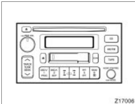
Type 4: AM/FM ETR radio/cassette player/ compact disc player/compact disc auto changer controller
