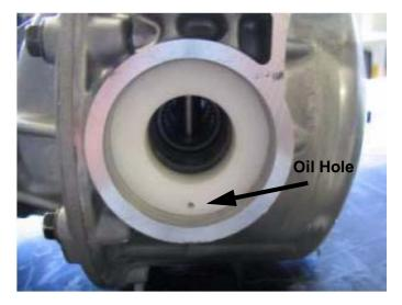
4. There should be a depth of ten millimeters between the support and the edge of the differential.
