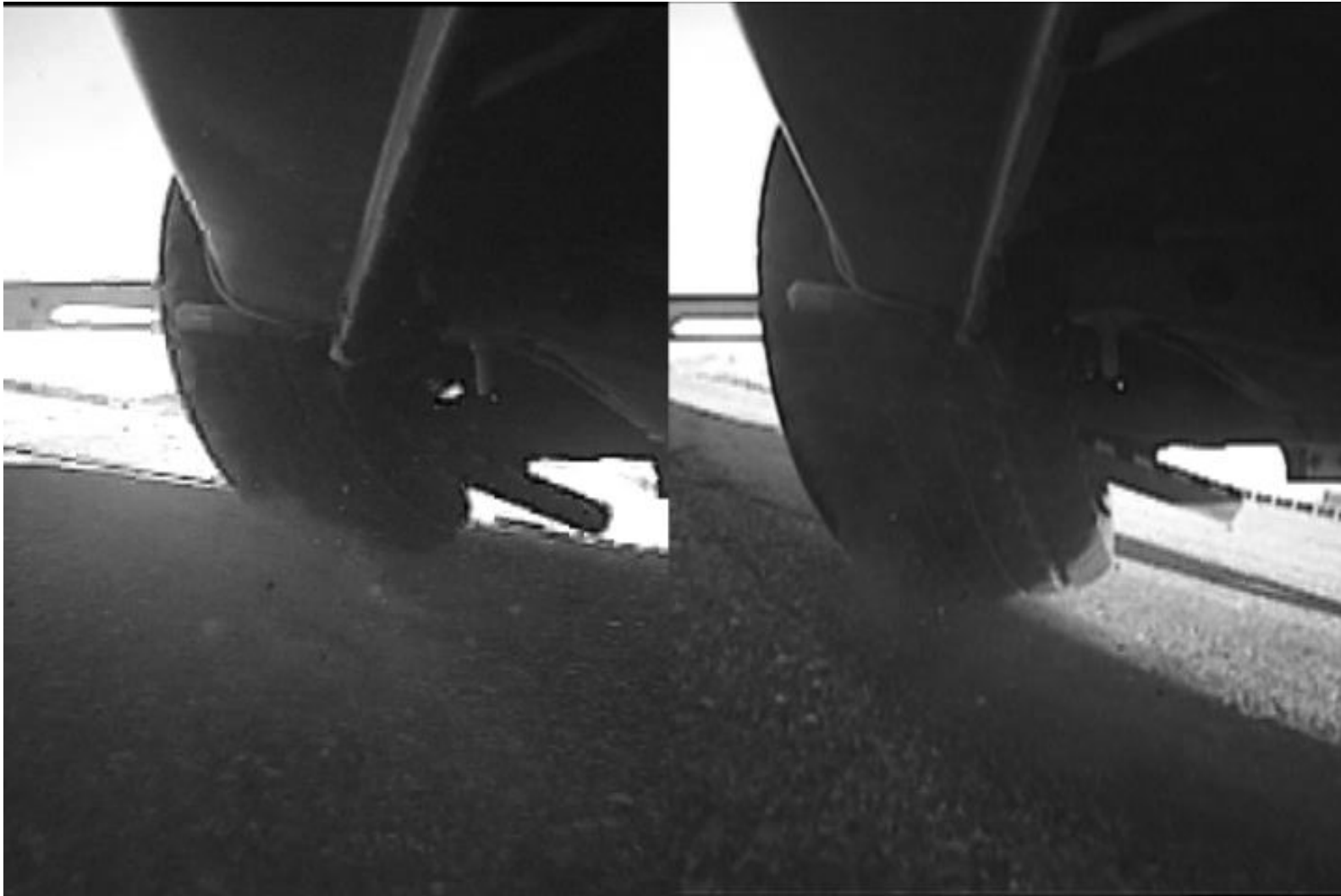
FIGURE 5. Comparison of front tire deformation of P225/75R15 (left) and 285/50R20 (right) at maximum tip-up. Wheels are zero offset on left and -2 mm offset on right.
