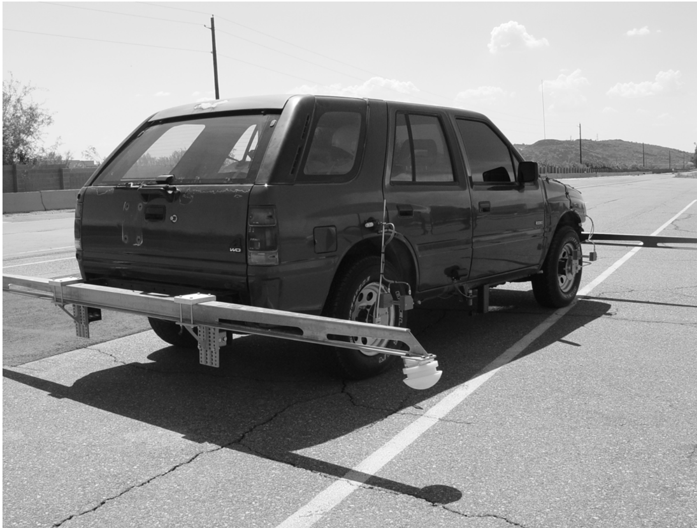
FIGURE 3. Test Vehicle with NHTSA-style outriggers and wheel lift sensors. The steering controller and tire video equipment are specific to the specific test center.
