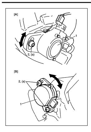
7) If ignition timing is out of specification, loosen flange bolt(s) (2), adjust timing by turning CMP sensor (1) while engine is running, and then tighten bolt(s) (2).
