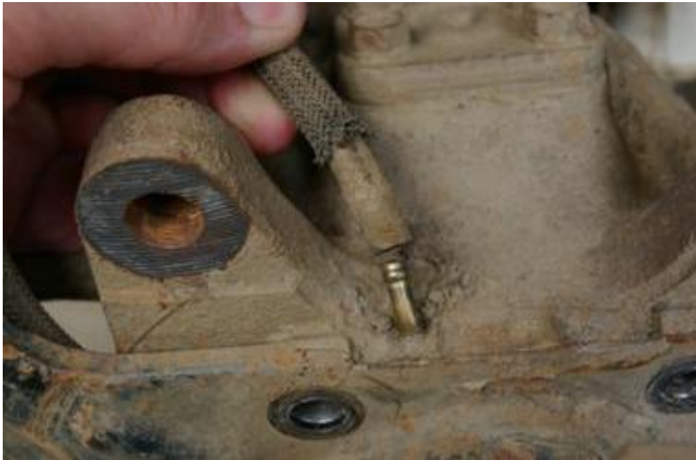
Figure 6. Lock tube (with brake calliper removed)
