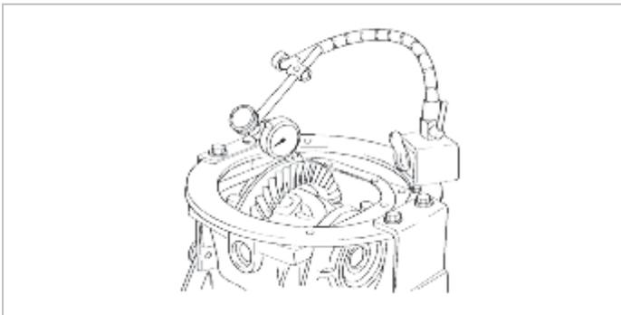
(8) Change the side bearing spacers as illustrated and then adjust the final drive gear backlash between the drive gear and the drive pinion.
