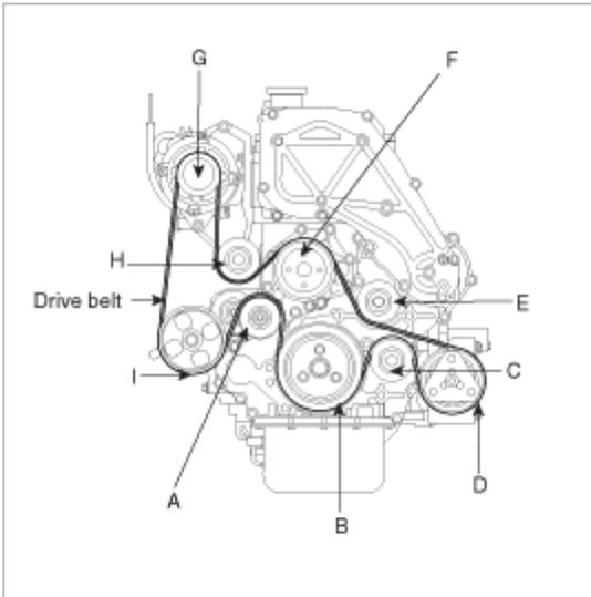
A. Install the belt in RH side of the auto-tensioner pulley.
