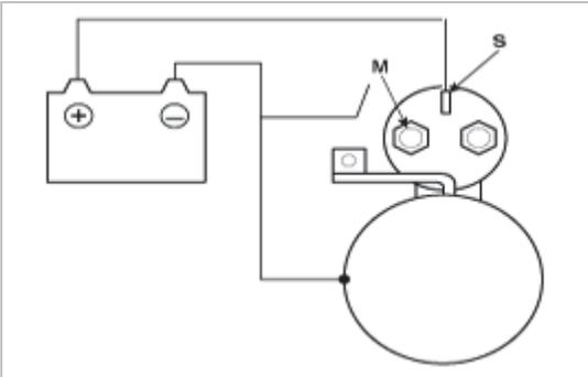
4. Disconnect the battery also from the body. If the pinion retracts immediately, it is working properly. To avoid damaging the starter, do not leave the battery connected for more than 10 seconds.
