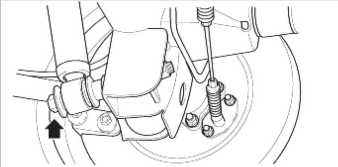
5. Loosen the lateral rod bolts and remove the lateral rod.
