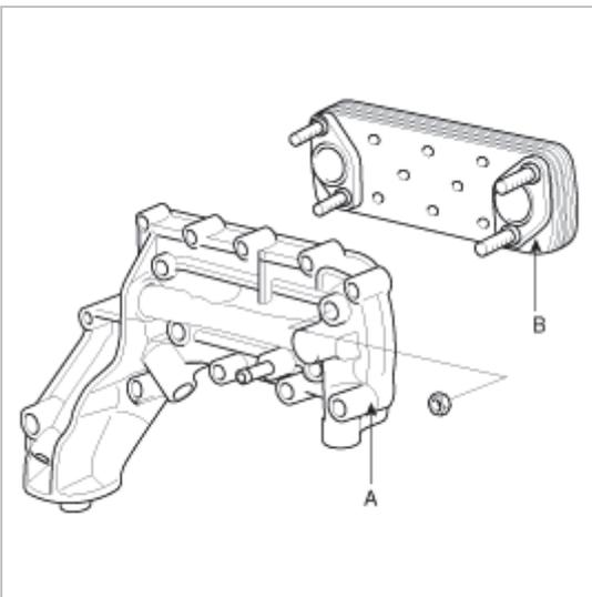
5. Remove the oil cooler by-pass valve (A) and the relief valve (B) from the oil cooler cover.
