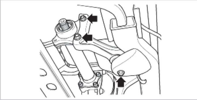
2. Remove output shaft from differential housing.
