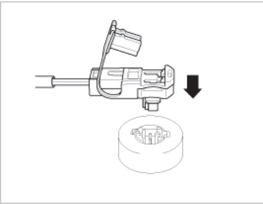
2. Press firmly the locking button of connector until the connector click to lock.
