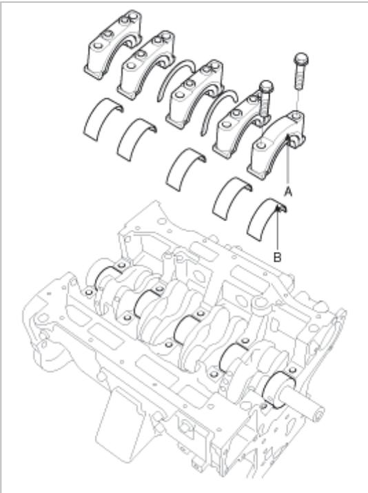
4. Remove the crank shaft (A) from cylinder block.
