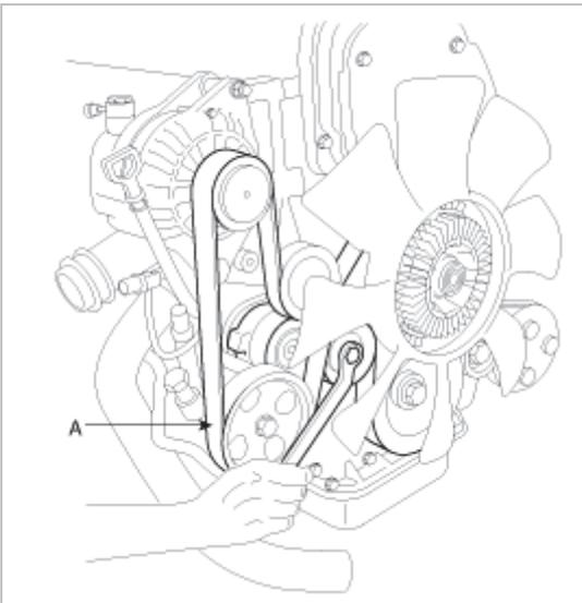
4. Remove the water pump pulley.
