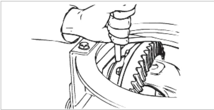
(6) Align the matchmarks on the gear carrier and the bearing cap and tighten the bearing cap.
