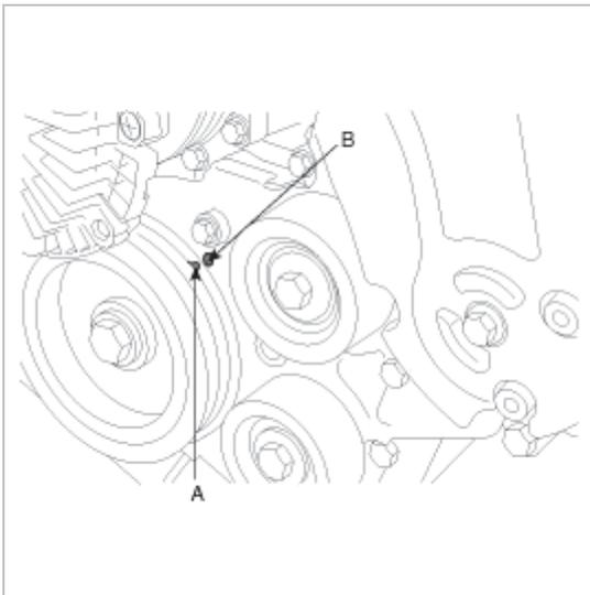
2. Remove the timing chain upper front cover(A).
