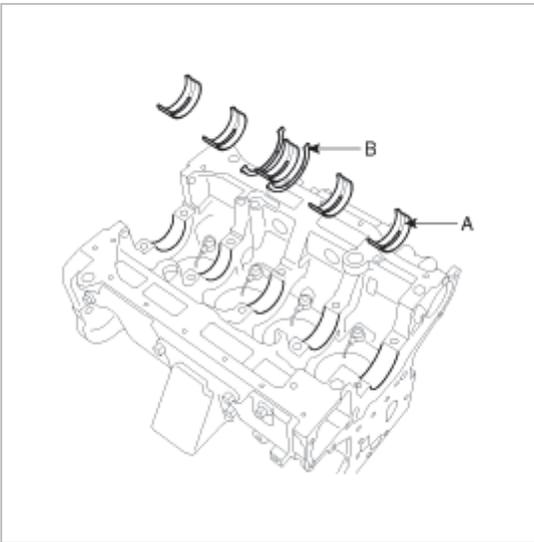
3. Install the thrust bearing (B).
