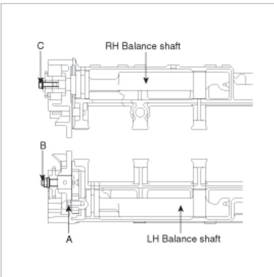
16. Install the balance shaft sprocket.
