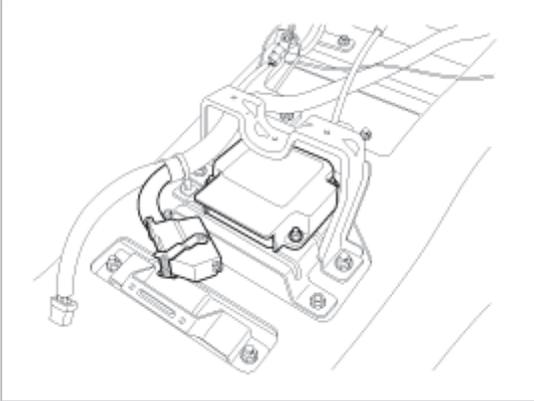
6. Remove the SRSCM mounting bolt (1EA) and nuts (2EA) from the SRSCM, then remove the SRSCM.
