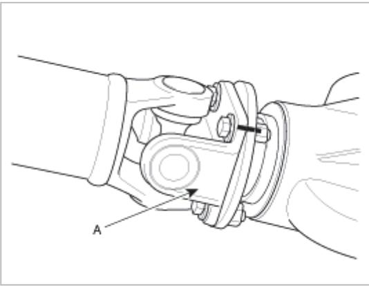
8. Remove the front propeller shaft (A).
