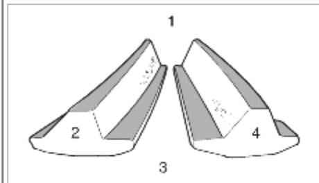
The drive pinion is positioned too close to the center of the drive gear.
