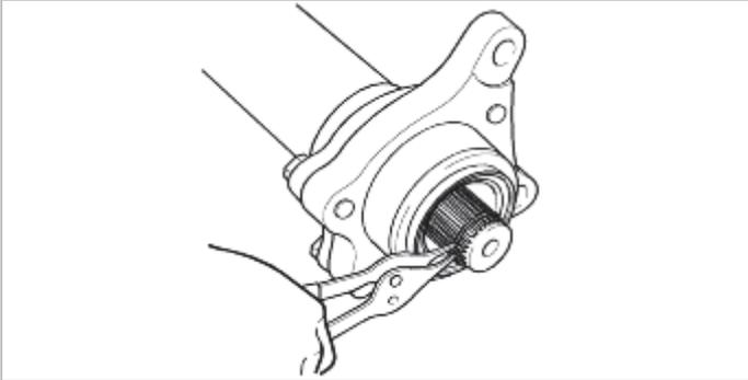
2. Remove output shaft housing.
