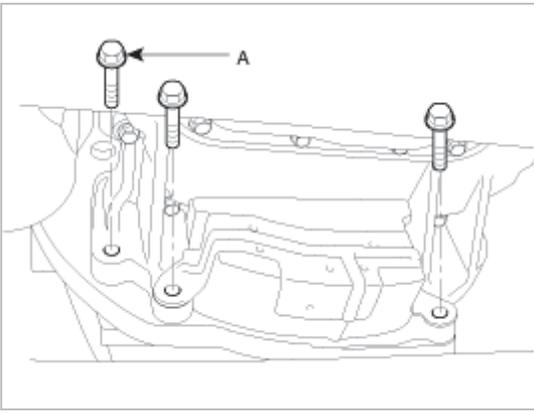
10. Remove the clutch release cylinder(A) and transmission mounting bolt(B).
