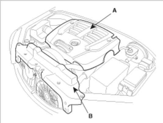
3. Drain the engine coolant after removing drain plug(A).
