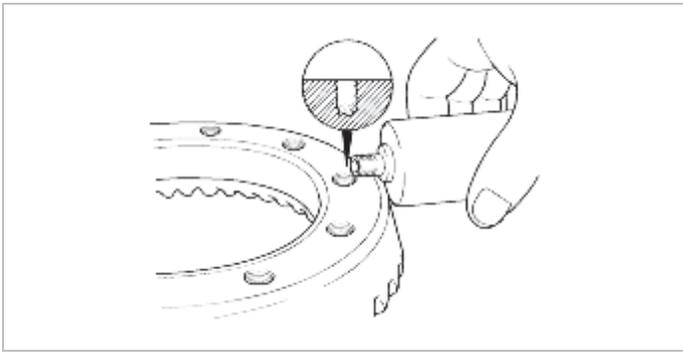
(4) Install the drive gear in the differential case with the matchmarks properly aligned. Tighten the bolts to the specified torque in a diagonal sequence.
