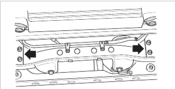
7. Remove the differential mounting bolt.
