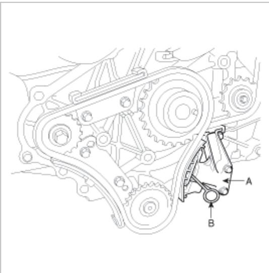
9. Assemble the RH balance shaft sprocket bolt(A).
