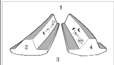
Decrease the thickness of the pinion height adjusting shim, and position the drive pinion further from the center of the drive gear.
