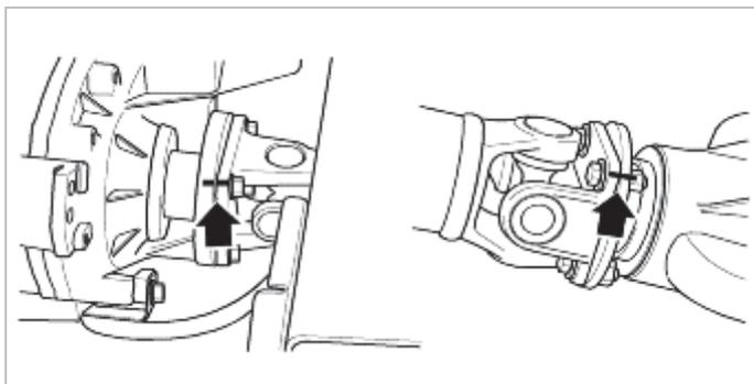
3. Remove four bolts holding universal flange to transfer case (4WD).
