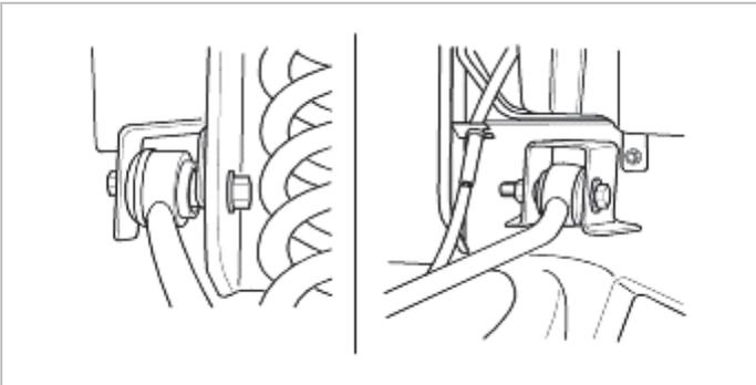
6. Install the upper arm ball joint into the top of the steering knuckle and tighten the side bolt and nut.
