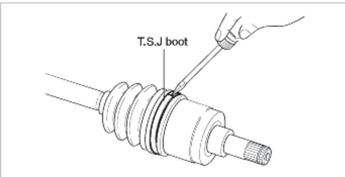
2. Remove the clip using a screwdriver.
