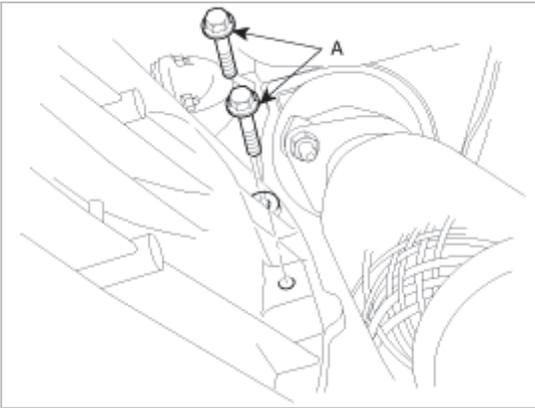
6. Install the starter motor mounting bolts(A) and wire harness mounting bolt(B).
