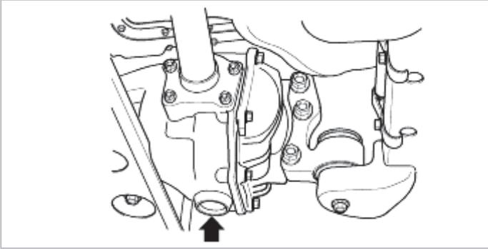
2. Remove the drive shaft and the output shaft.
