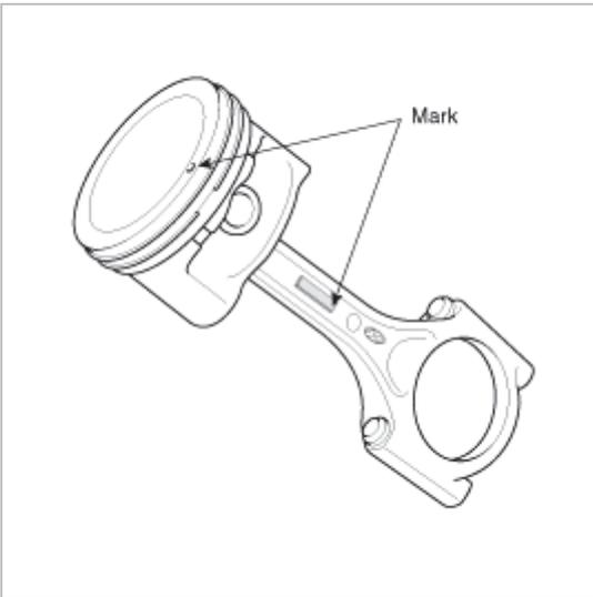
7. Line up the front marks and insert the piston pin. The piston pin must be smoothly pressed by hand into position.
