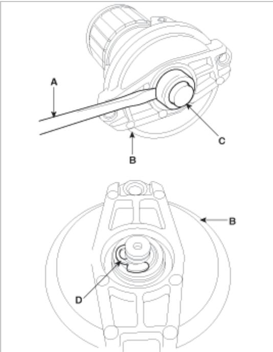
6. Separat the rear bracket(A), brush holder(B), armature(C).
