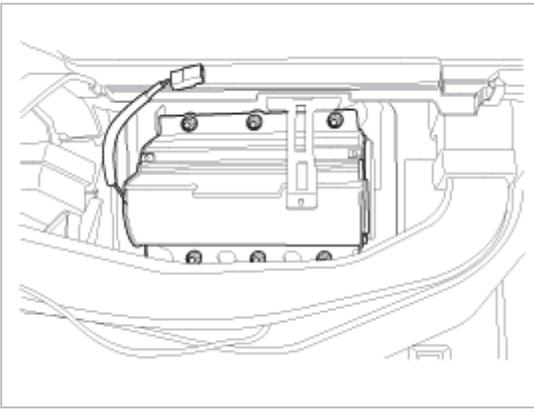
4. Install the heater duct to the crash pad.
