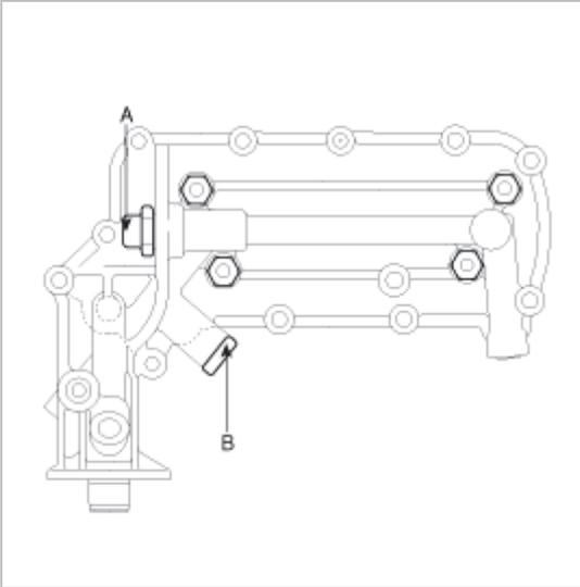
2. Install the oil cooler (B) to oil cooler cover (A).
