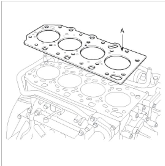
4. Install the cylinder head assembly with the cylinder head gasket.
