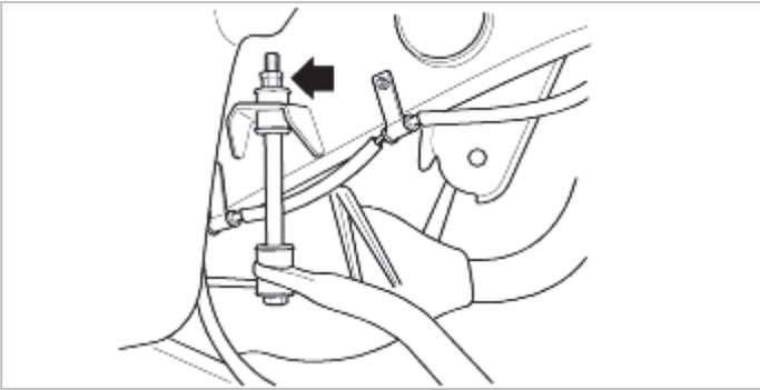
5. Remove the rear shock absorber lower nut and washer.
