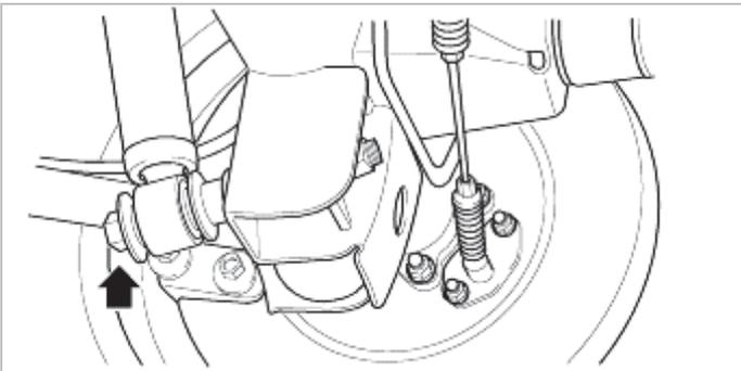
6. Remove the shock absorber upper bolt, and then remove the shock absorber.
