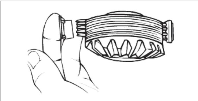
3. Select a shim 0.76mm (0.030in.) thick and place on the hub side of the disc pack subassembly.
