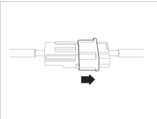
2. Disconnect the connector completely.
