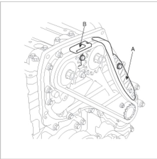
9. Remove the LH and RH camshaft sprocket bolts.
