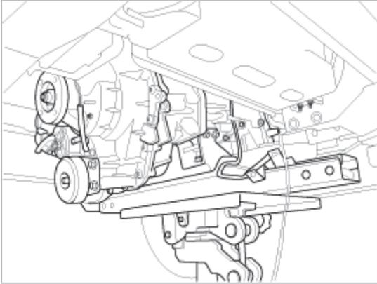
15. Remove the vehicle speed sensor connector(A).
