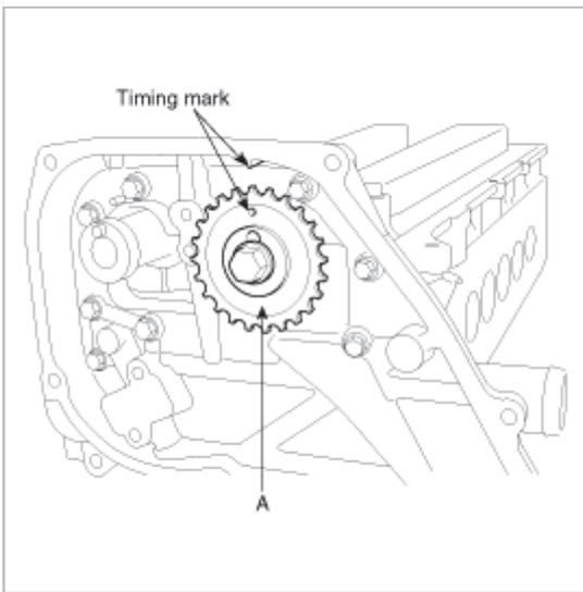
6. Align the RH camshaft dowel pin(A) with the timing mark(B) of the timing chain upper under cover.
