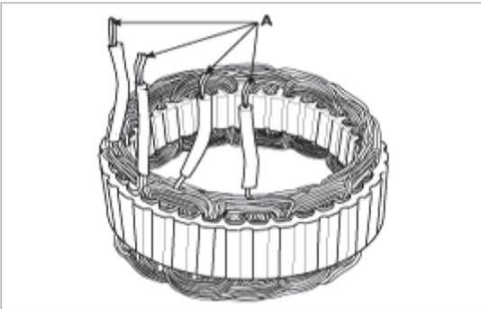
2. Check that there is no continuity between each lead and the coil core.
