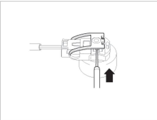
2. Lift up the connector inserting the driver underlay the connector body.
