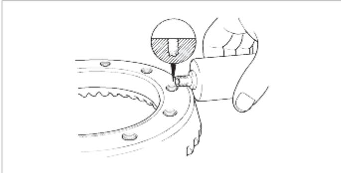
7. Press-fit the side bearing inner race
