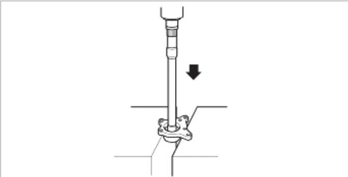
4. Install the output shaft housing to the bearing housing.
