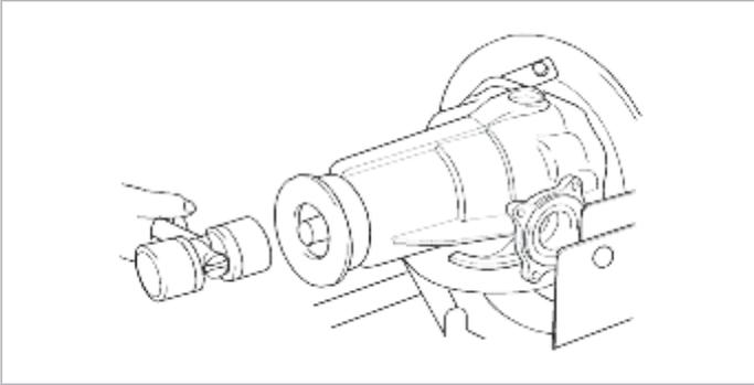
**7. REMOVAL OF DRIVE PINION REAR BEARING INNER RACE**
