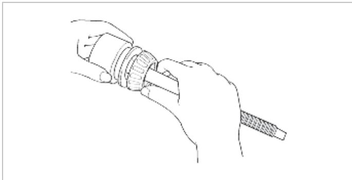
(3) Install pinion model assembly to carrier.
