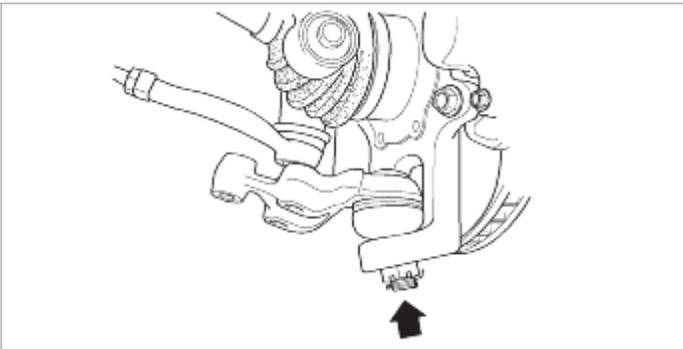
7. Remove the lower arm ball joint from the steering knuckle with SST.
