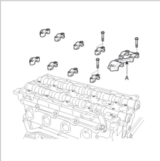
3. Remove the cam shaft(A).
