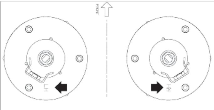
2. Install the mounting block nuts by 3-4 threads only.
