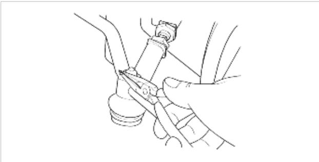
4. Insert upper arm link lock bolt with spring washer and tighten nut.
