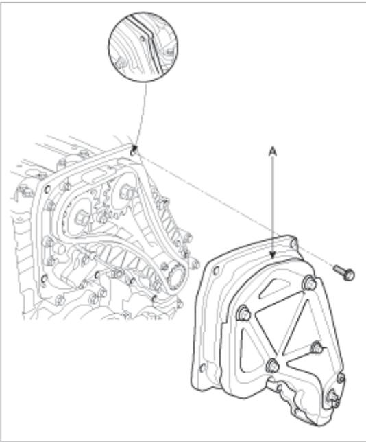
3. Remove the cylinder head cover.
