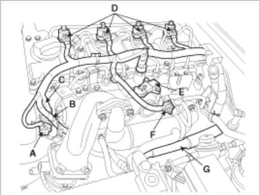
30. Remove the fuel hose from the high pressure pump.
