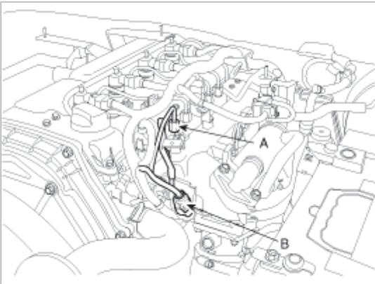
3. Remove the high pump fuel hose bracket(A).
