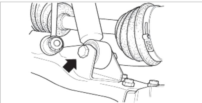
6. Install the lower nut of control link of stabilizer bar.
