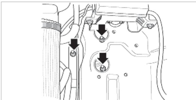
11. Install the battery mounting bracket and the battery.
