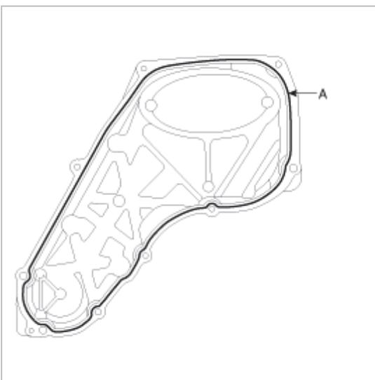
16. Install the timing chain upper front cover(A).
