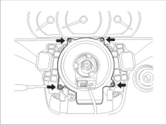
8. Disconnect the clock spring wiring harness and the horn wiring harness connector from the clock spring.
