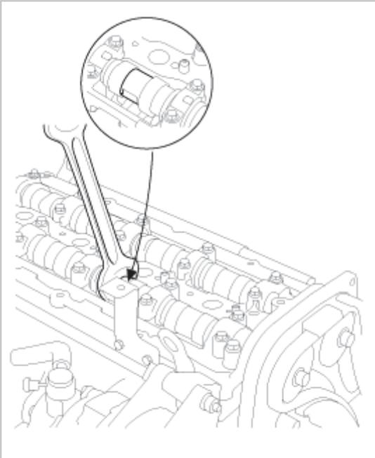
5. Insert the SST(09311-4A00) into timing chain upper cover. And then remove the high pressure pump and sprocket.
