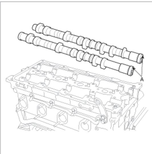
4. Remove the cam shaft carrier(A).
