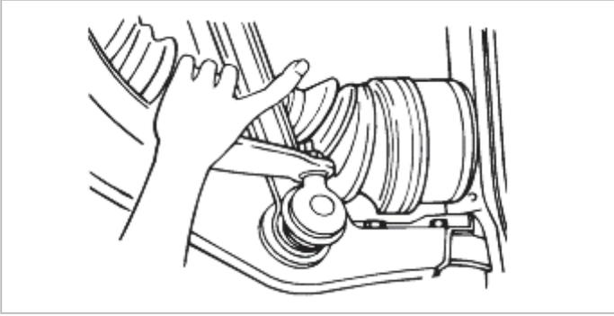
2. Test for loose drive shaft splines. By grasping the drive shaft and tugging up and down and fore and aft.
