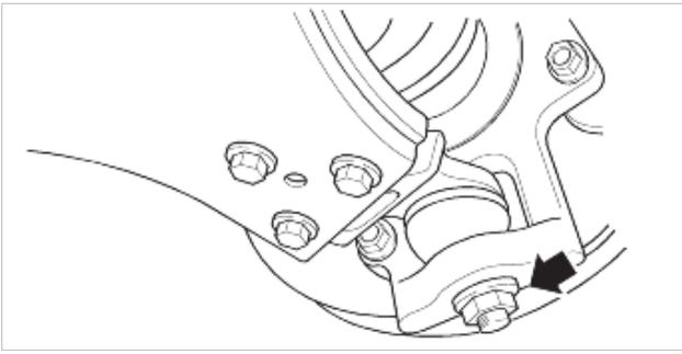
8. Remove steering knuckle from vehicle.
