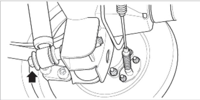
5. Remove wheel speed sensor cable from rear lower arm.
