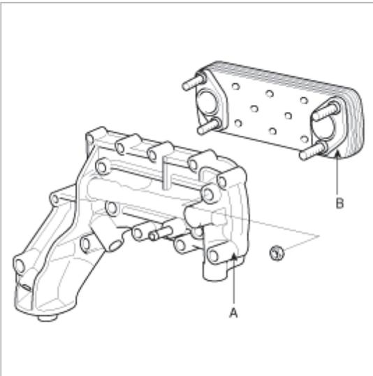
3. Install the oil cooler assembly (A) to the cylinder block with new gasket.
