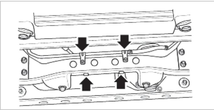
5. Remove the differential mounting bracket.
