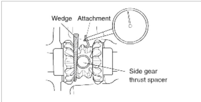
2. If the backlash exceeds the limit, adjust using side bearing spacers.
