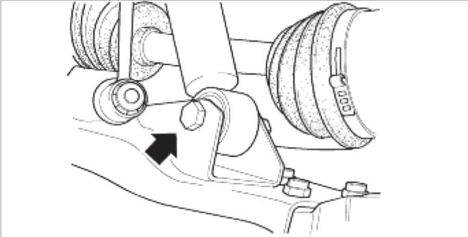
5. Remove the bolts and nuts that joins lower arm and lower arm ball joint.
