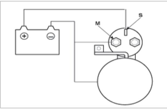
3. Disconnect the battery from the M terminal.
