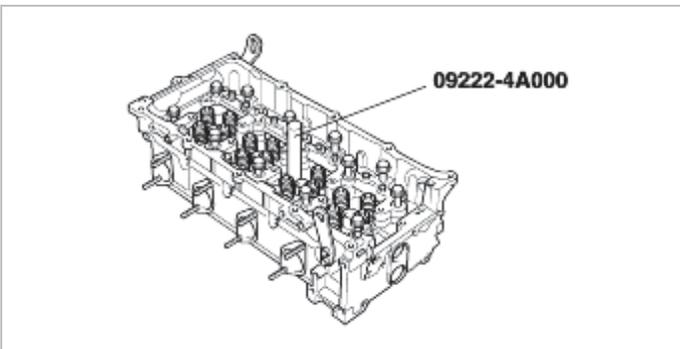
2. Using the special tool (09222-4A000), remove the valve.
