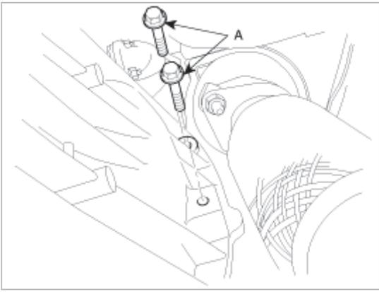
14. Lower the jack slightly to make easy to remove the related connector and bolts on the upper part of transmission.
