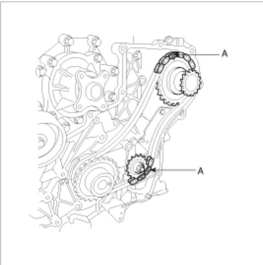
9. Assemble the high-pressure pump sprocket to the high-pressure pump tentatively.
