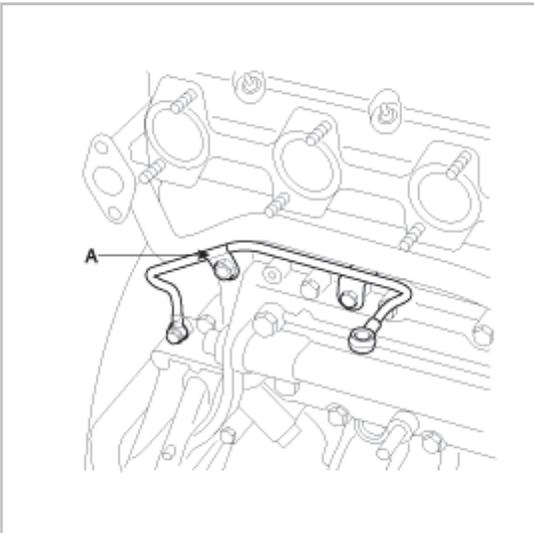
3. Install the exhaust manifold(A) from cylinder head.
