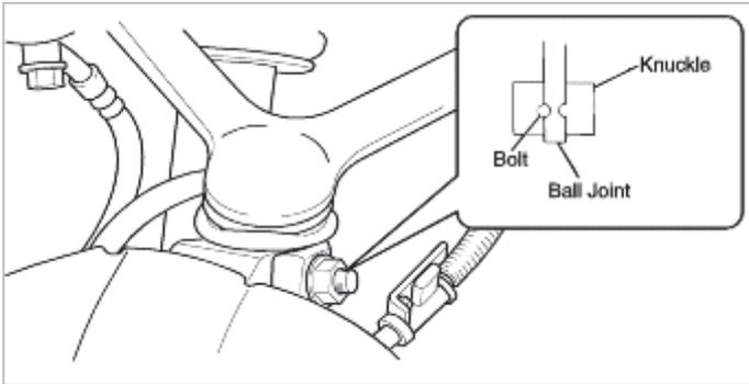
7. Tighten the upper arm bolts and nuts and then install brake hose brackets.
