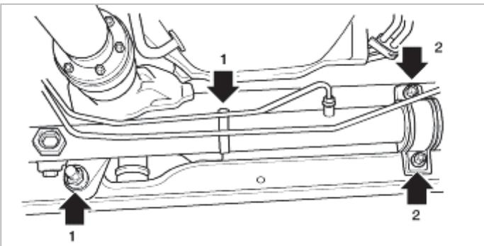
9. Remove the spindle from the front frame crossmember brackets during raising the steering gear box by using
