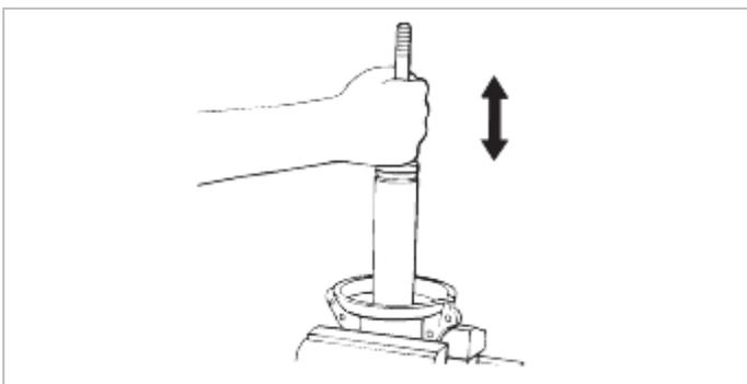
2. Inspect the entire shock absorber for signs of oil leakage; replace if required.
