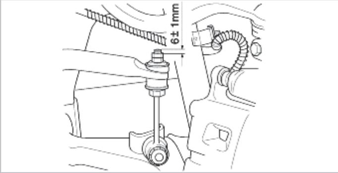
6. Tighten the lower nut of control link.
