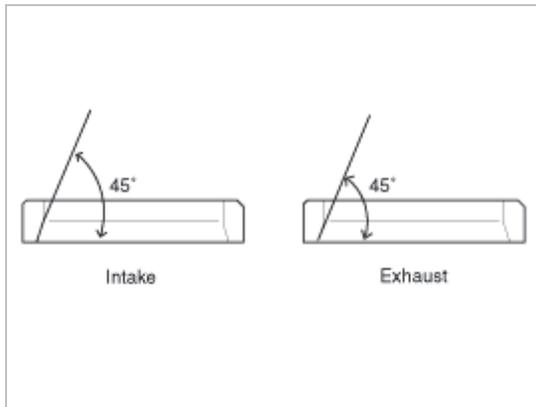
7. Seat the valve to the valve seat with a lapping compound.
