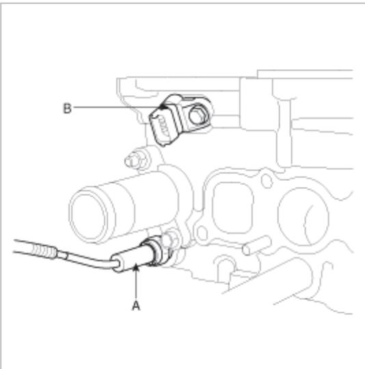
3. Install the water temperature sensor (A).
