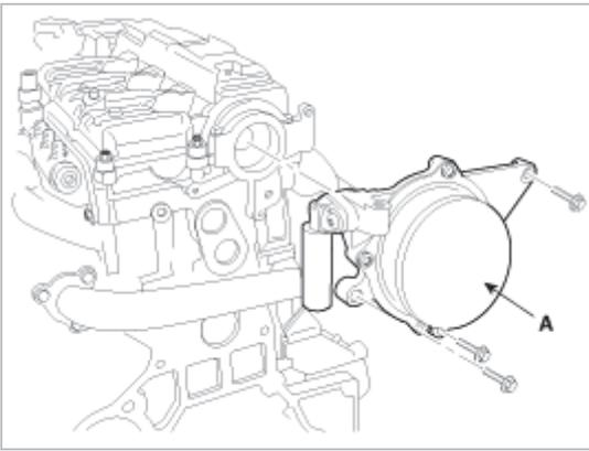
4. Remove the cylinder head cover(A).
