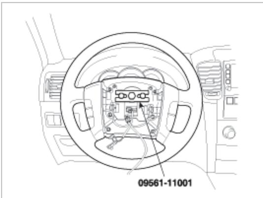
6. Remove the steering wheel column cover after unscrewing 3 screws.
