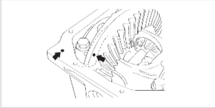
(7) With the drive pinion locked in place, measure the final drive gear backlash with a dial indicator on the drive gear.
