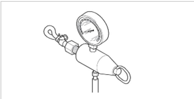
4. Check that if transfer lever is shifted to 2H then promptly Air pressure gauge value drops down.
