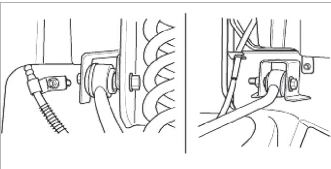
7. Remove the shock absorber lower nut.
