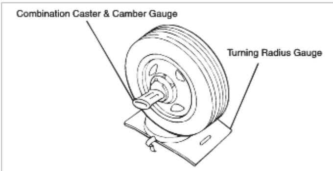
3. Attach a standard caster gauge to the hub and measure the caster.
