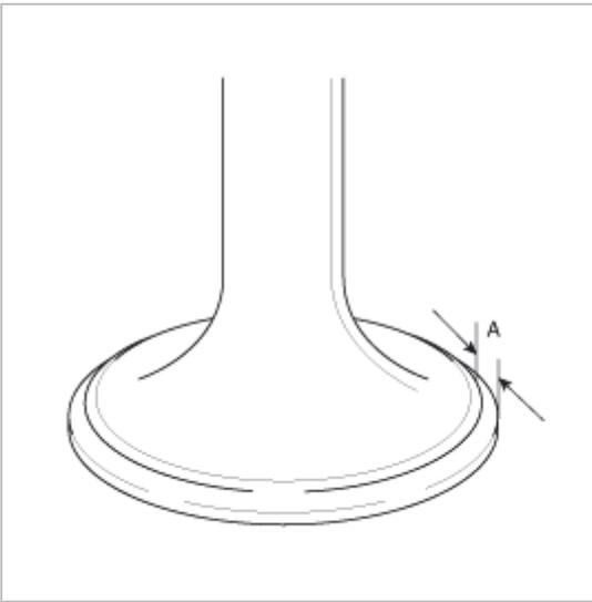
6. Check that valve seating position is at center of valve face.
