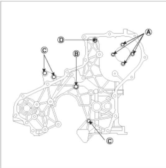
14. Insert a screw driver(C) in the cylinder block plug hole (B). Because, prevent rotation of balance shaft (A).
