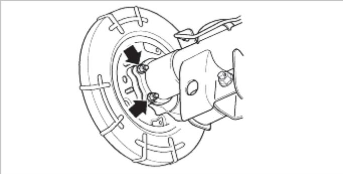
5. Adjust the parking brake lever stroke.
