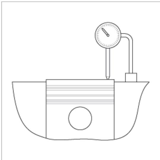
(2) Select the gasket from the grade A to C in the table below using the average of the 8 piston protrusion. Even if only 1 point is over than the limit of piston protrusion at each grade, 1 grade upper gasket than specified below.
