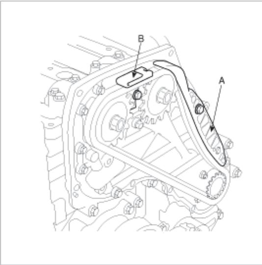
11. Install the timing chain lever "C"(A).
