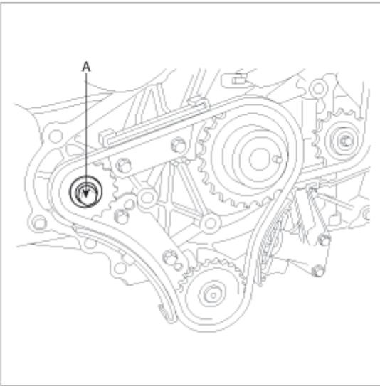
10. Remove the screwdriver (or bolt) from the plughole(A) and install the plug.
