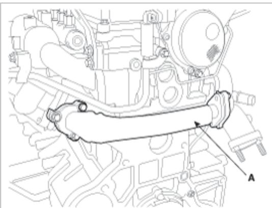
6. Install the oil hose(A) and coolant hose(B) from turbo charge.
