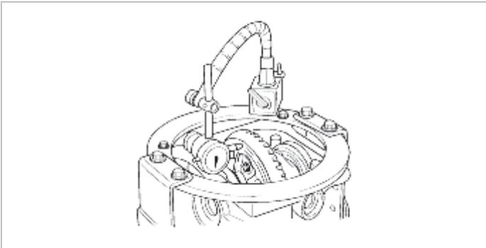
(11) If the drive gear runout exceeds the limit, reinstall by changing the position of the drive gear and differential case, and remeasure.
