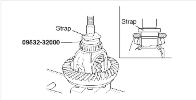
10. Attach actuator at differential case RH side as figure
