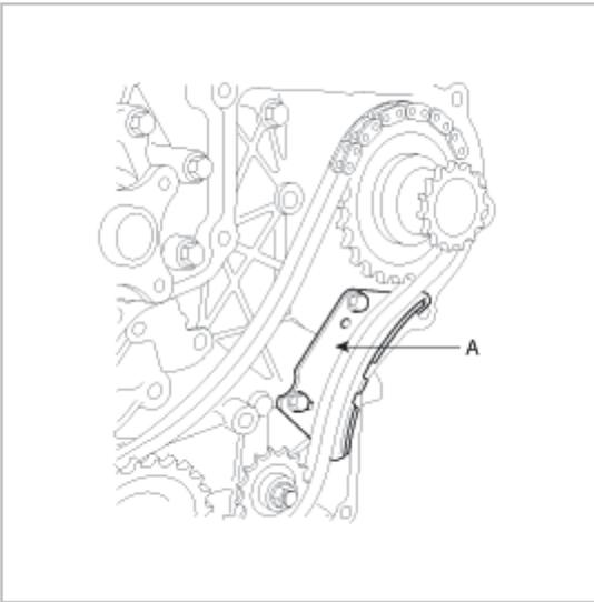
6. Remove the timing chain "A"(B) with the high-pressure pump sprocket(A).
