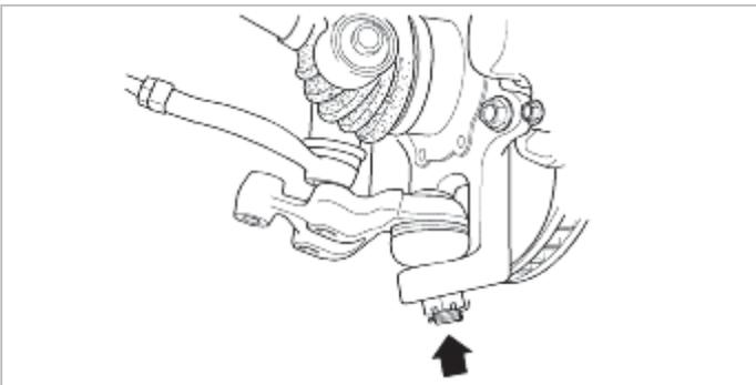
3. Position the lower arm to the front frame crossmember brackets and then position the spindle during lift up the
