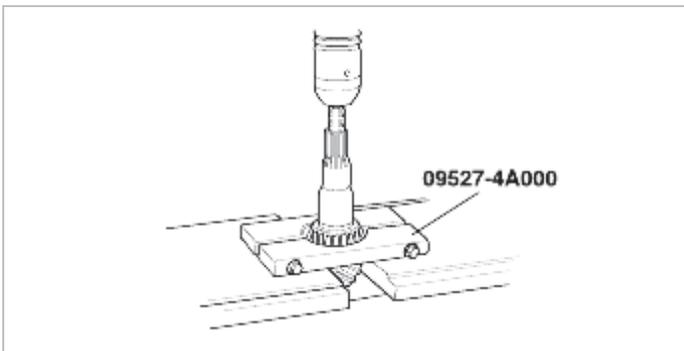
**8. REMOVAL OF OIL SEAR / DRIVE PINION FRONT BEARING INNER RACE / DRIVE PINION FRONT BEARING OUTER RACE**
