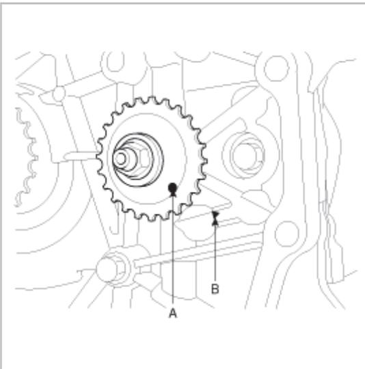
5. Check the LH balance shaft(A) whether it is located at the right position. To prevent the rotation of balance shaft, remove plug(B) at the side of cylinderblock. Insert screwdriver(C) (or bolt) with an 8 mm (0.32in) diameter into the plughole and check whether it slides more than 60 mm(2.4in).
