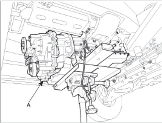
2. Tighten the transmission mounting bolts.
