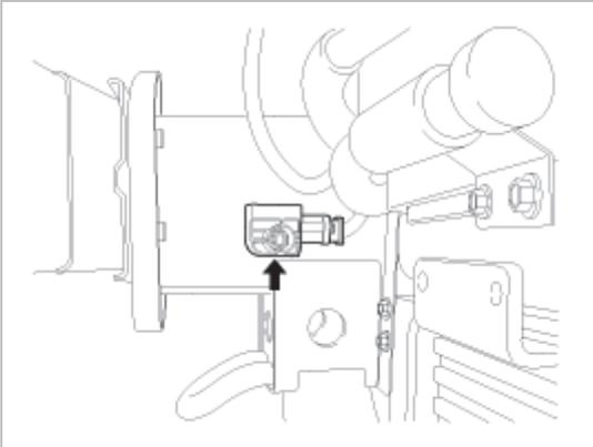
4. Disconnect the Front Impact Sensor connector.
