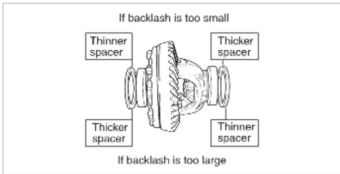
(9) Check the drive gear and drive pinion for tooth contact. If poor contact is evident, adjust again.
