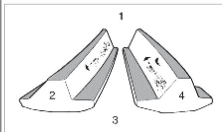
The drive pinion is positioned too close to the center of the drive gear.
