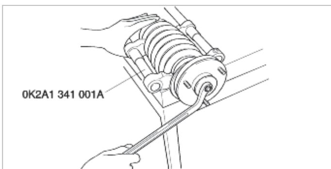
5. Carefully loosen the coil spring compressor and remove it.
