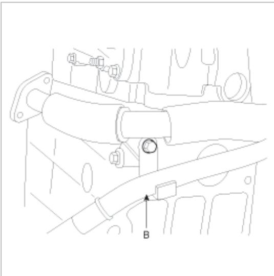
21. Install the power steering pump bracket (A).
