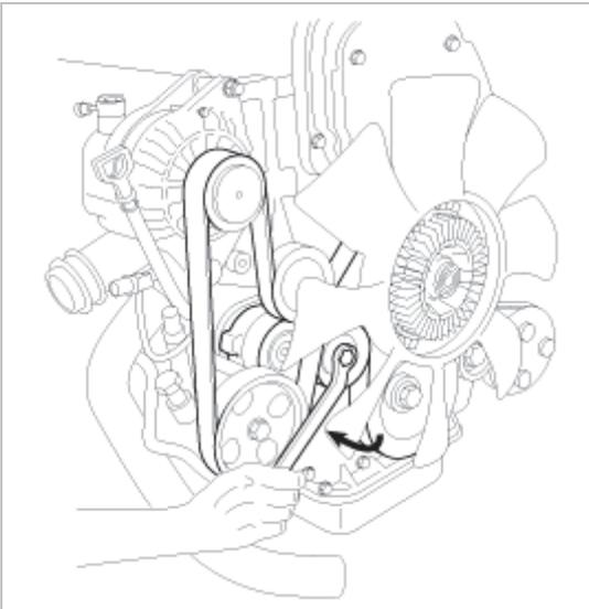
3. The tensioner mark should be between the " \* " position.
