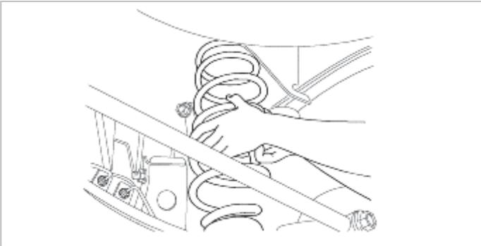
3. Install the shock absorber upper nut.
