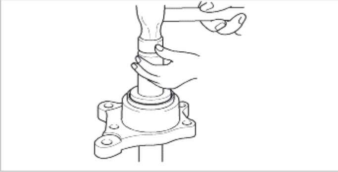
2. Using a hydraulic press, install bearing onto output shaft.
