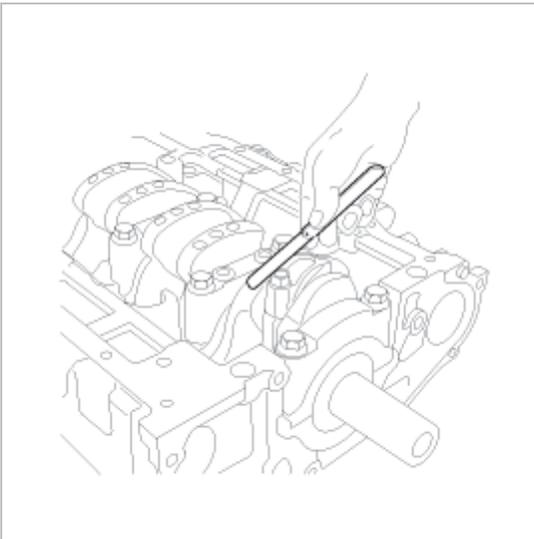
2. Remove the connecting rod cap.
