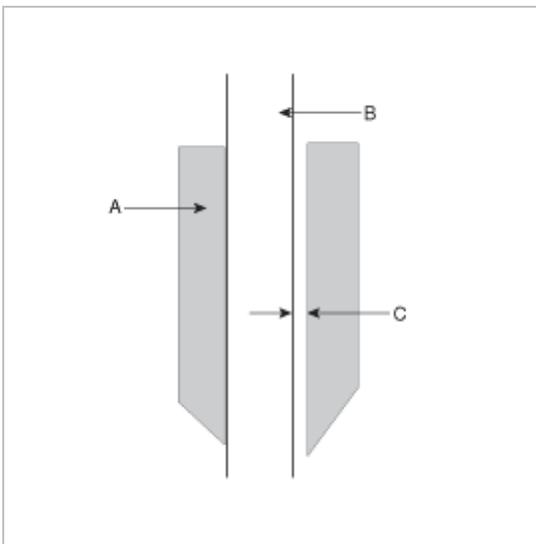
7. If clearance exceeds maximum, replace valve and/or cylinder head
