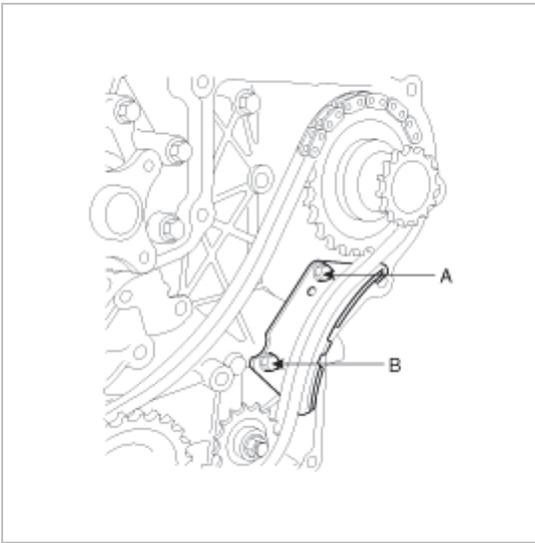
11. Install the timing chain lever "A"(A).
