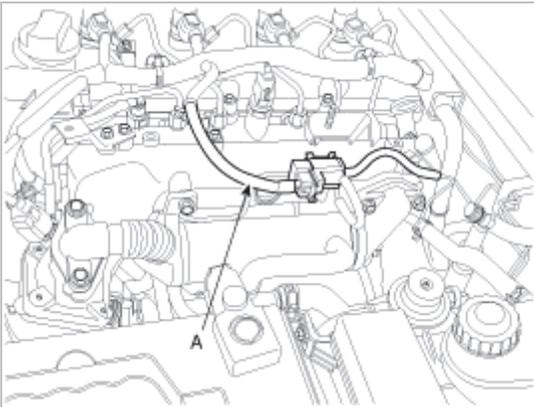
2. Remove the high pipe bracket(A) and the coolant temperature sensor connector(B).
