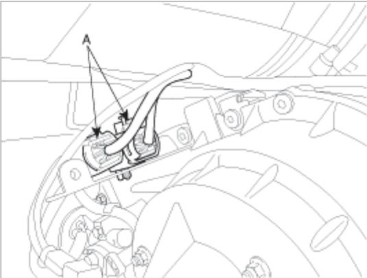
4. Install the vehicle speed sensor connector(A).
