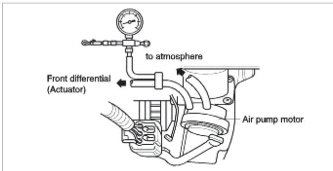
2. Turn the ignition switch on and shift the transfer lever 2H→4H.
