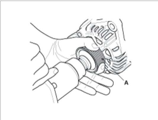
5. Remove the rear bracket nuts(A).
