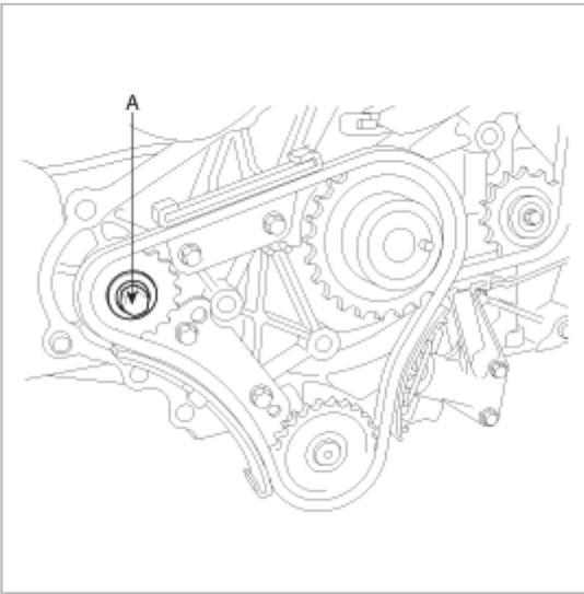
7. Remove the timing chain auto-tensioner "B"(A).
