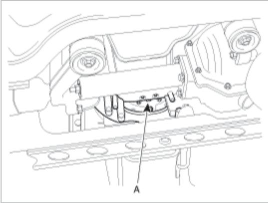
16. Remove the transmission housing mounting bolt.
