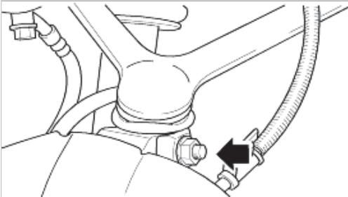
6. Remove tie rod end cotter pin and using a ball joint remover, remove tie rod end from steering knuckle.
