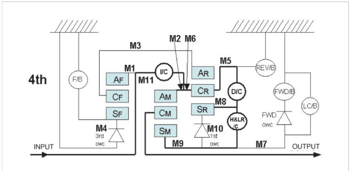
C. Driving force is conveyed to the front internal gear, the middle internal gear, and the rear carrier and the three planetary gears rotate forward as a unit.
