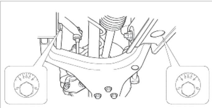
5. Install the lower nut of the shock absorber.
