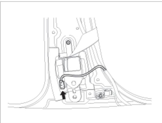
6. Loosen the Seat Belt Pretensioner mounting bolt and remove the Seat Belt Pretensioner.
