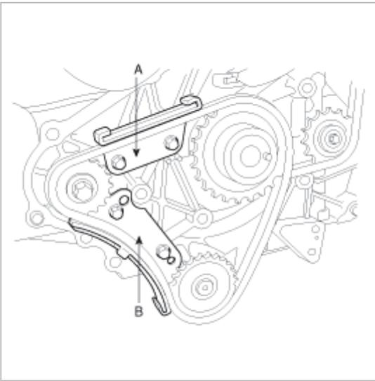
8. Install the timing chain auto-tensioner "B"(A), and remove the set pin(B) from the auto-tensioner.
