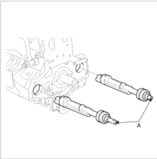
20. Remove the rear oil seal case (A).
