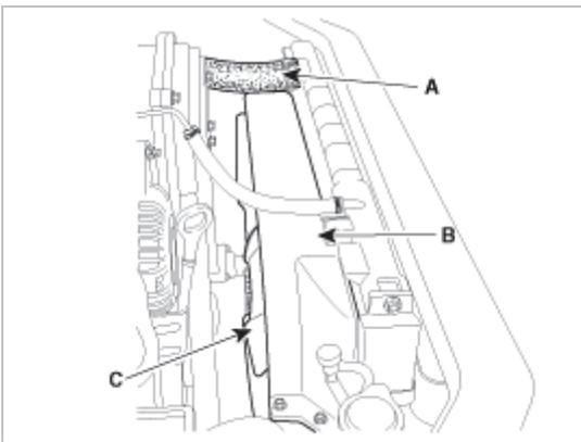
13. Remove the cooling fan(C).
