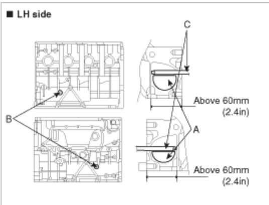
15. Install the LH balance shaft driven gear bolt (A) (8 x 16).
