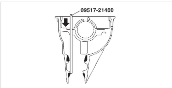
**9. REMOVAL OF DRIVE PINION REAR BEARING OUTER RACE**
