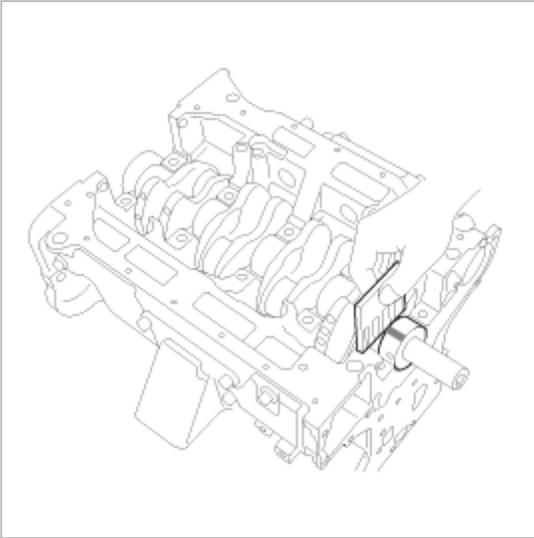
4. If oil clearance exceeds specification, replace the main bearing.
