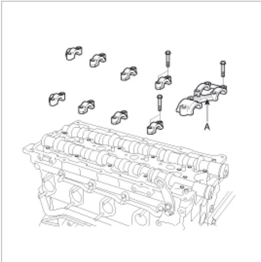
2. Check the camshaft journals for wear. If the journals are badly worn, replace the camshaft.
