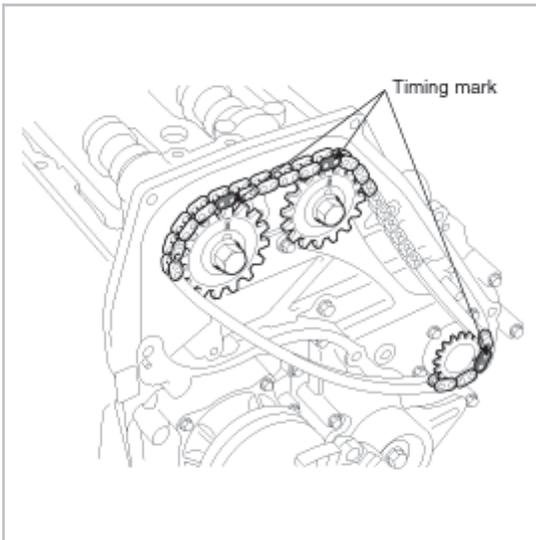
9. Assemble the RH camshaft sprocket to the RH camshaft tentatively.
