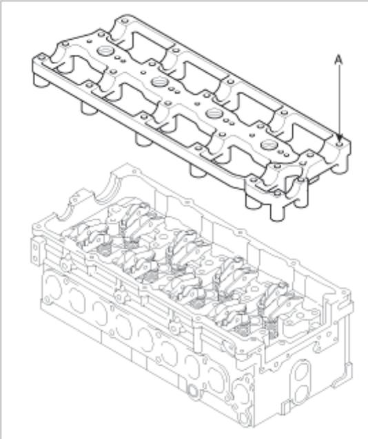
8. Install the camshaft (A) on the camshaft carrier.
