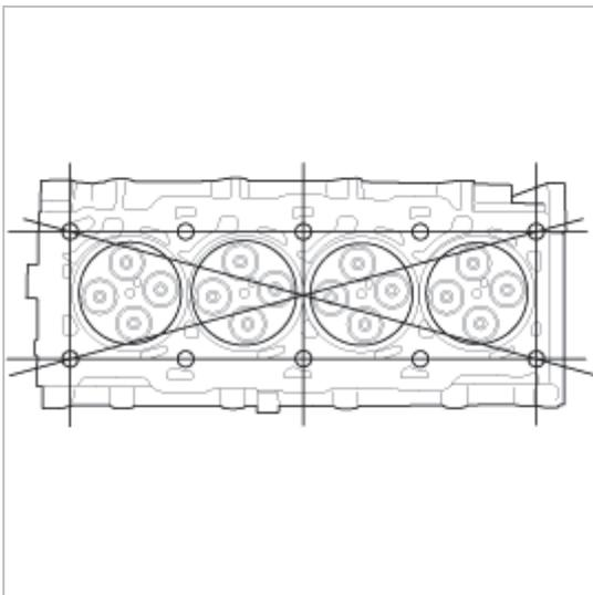
3. Measure manifold contact surface distortion in four directions shown in figure.
