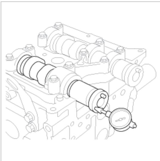
3. Clean the camshaft bearing surfaces in the cylinder head then set the camshaft back in place.
