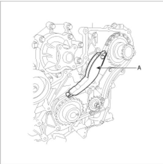
5. Remove the timing chain guide "A"(A).
