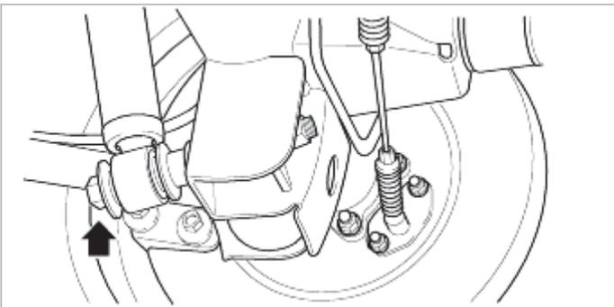
5. Install the stabilizer link upper mounting nut to the specified length.
