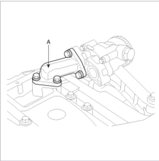
4. Install the oil screen (A) to the oil pump.
