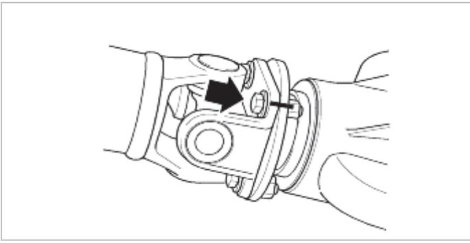
6. After installing the propeller shaft fill the grease into the nipple until it comes out from the sleeve yoke plug hole.
