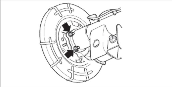
4. Remove the rear axle shaft.
