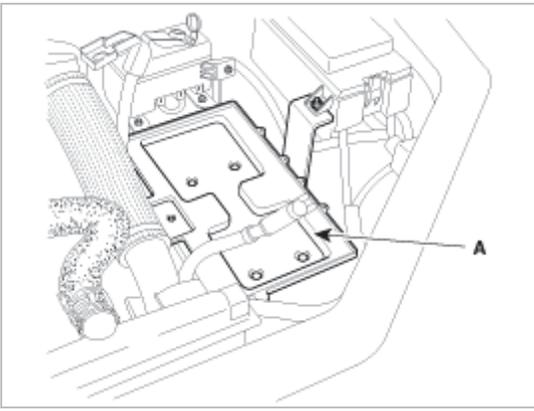
6. Remove the inter cooler hose and pipe on the intake manifold side(A).
