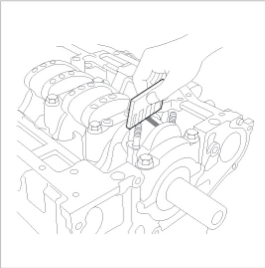
4. If oil clearance exceeds specification, replace the connecting rod bearing.
