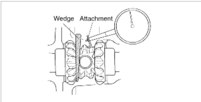
4. If the differential gear backlash exceeds the limit, adjust the backlash by installing thicker side gear thrust spacers.
