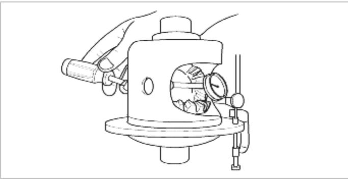
9. Remove the side gear subassembly and repeat the tooth backlash procedure for the other gear pack on the opposite side of the case.
