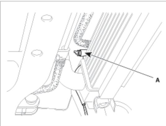
4. Remove the transmission oil drain plug(A).
