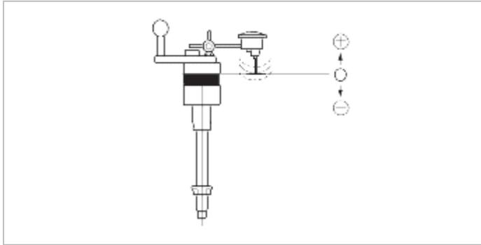
5. Adjustment of drive pinion preload.
