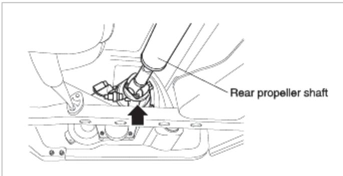
4. Connect the propeller shaft spline to transmission (2WD)
