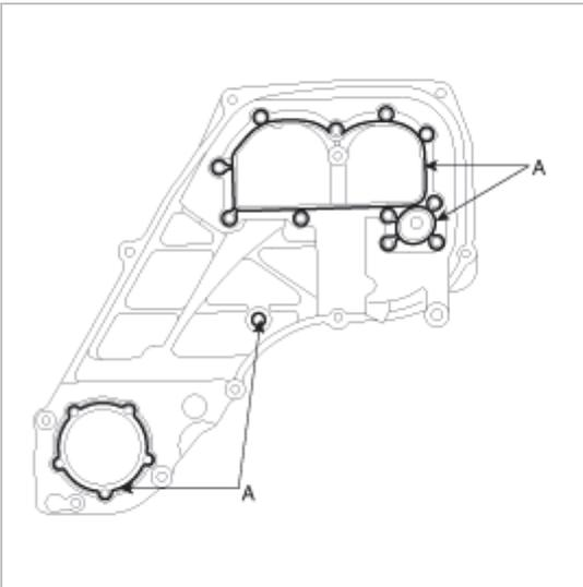
4. Install the timing chain upper under cover(A).
