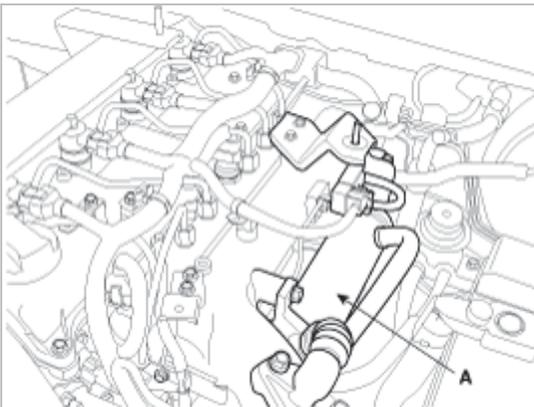
7. Remove the intake manifold.
