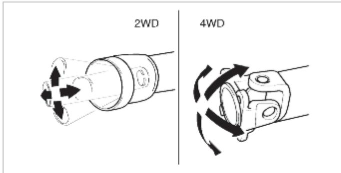
5. Check the center bearing for smooth movement (2WD).
