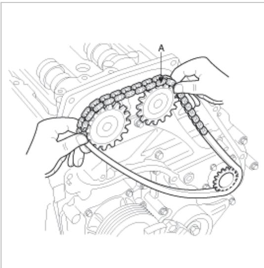
11. Remove the timing chain upper under cover(A).
