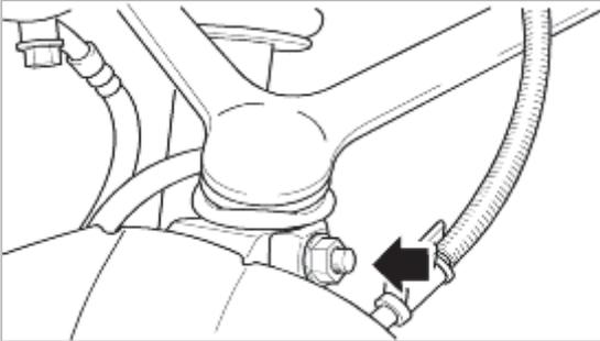
4. Remove the brake hose bracket and then remove the upper arm bolts and nuts.
