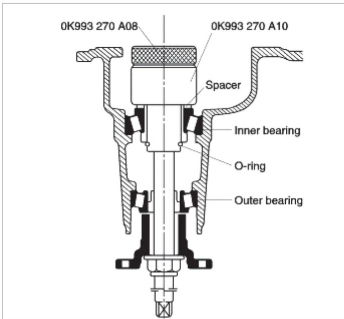
(6) Put pinion height adjusting gauge body at right angle and adjust it to 0.
