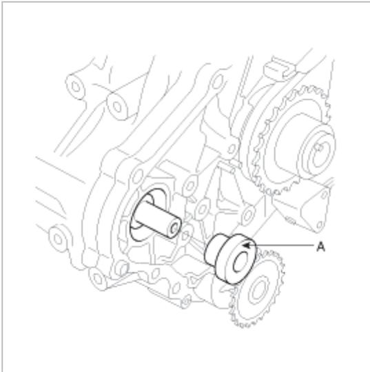
5. Using the chain connected to RH balance shaft sprocket, install as the timing marks(A) of crankshaft sprocket and oil pump sprocket align with each other.
