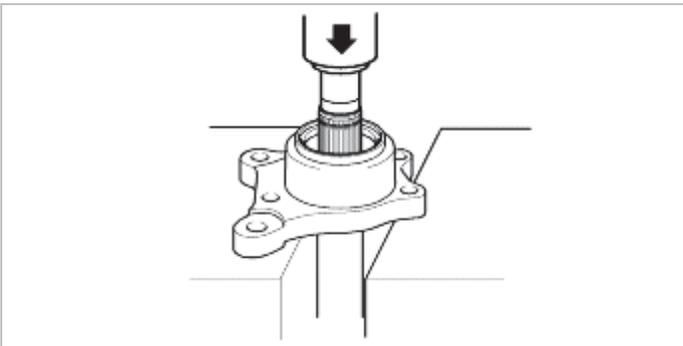
4. Remove dust seal and then using a hydraulic press, remove bearing.
