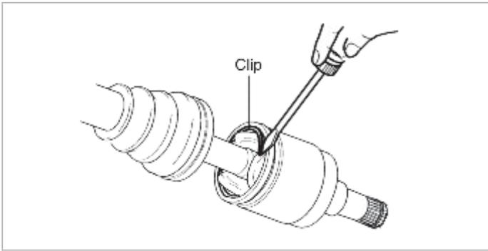
3. Remove the drive shaft from the T.S.J outer race.
