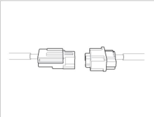
2. Connect the connectors till occurring the sounds of locking completely in the direction of an arrow below.
