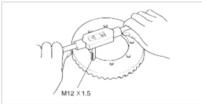
C. Apply the specified adhesive to the threaded holes of the drive gear.
