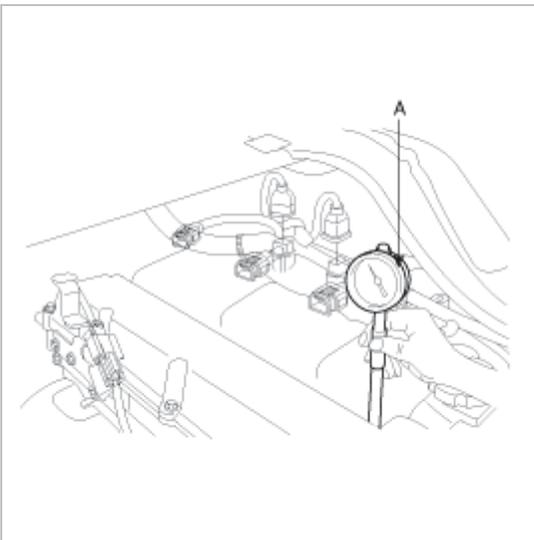
9. Repeat steps 7 to 8 for all cylinders, ensuring that the pressure difference for each of the cylinders is within the specified limit.
