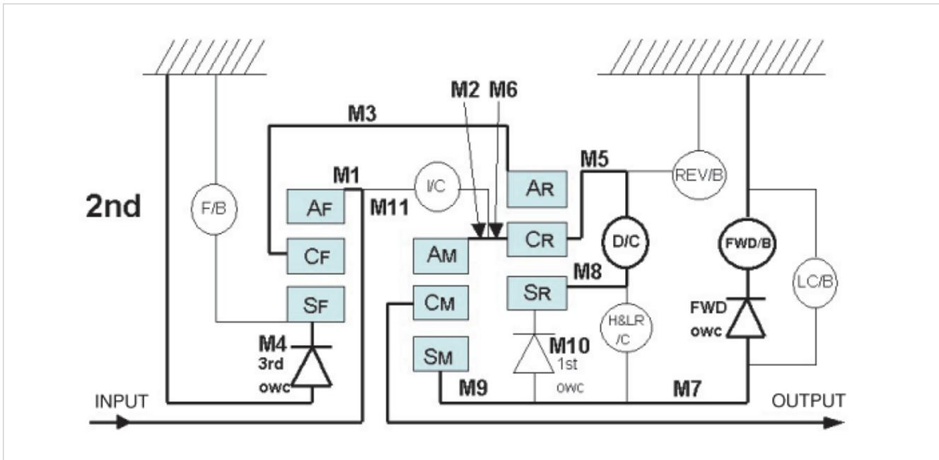
The direct clutch is coupled and the rear carrier and the rear sun gear are connected.
