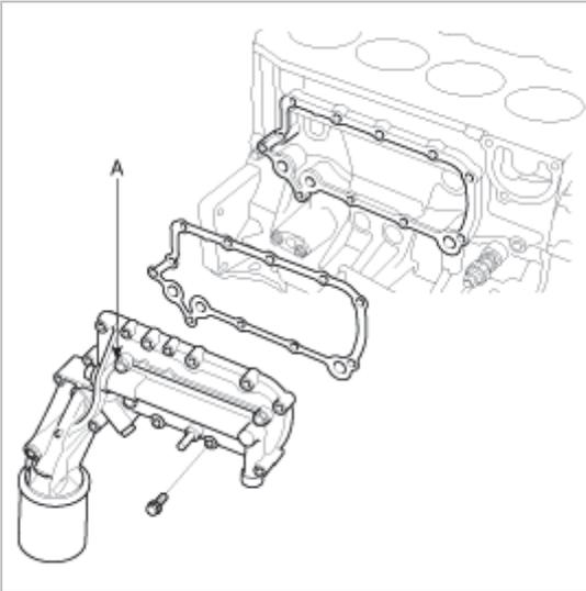
4. Remove the oil cooler (B) from the oil cooler cover (A).
