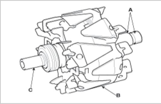
2. Check that there is no continuity between the slip rings and the rotor(B) or rotor shaft(C).
