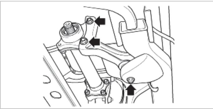
3. Tighten diff mounting bracket bolt.
