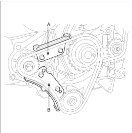
9. Remove the RH balance shaft sprocket bolt.
