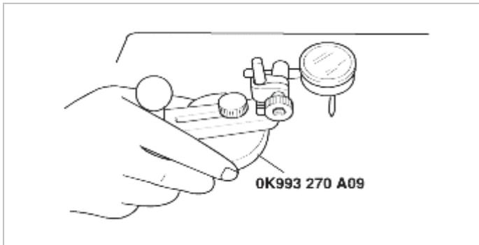
(7) Put pinion height adjusting gauge body and gauge block to the upper side of pinion model.
