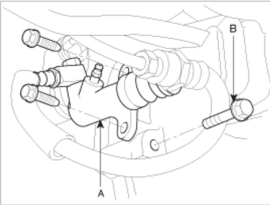
9. Install the Tighten the transaxle lower mounting bolts(A).
