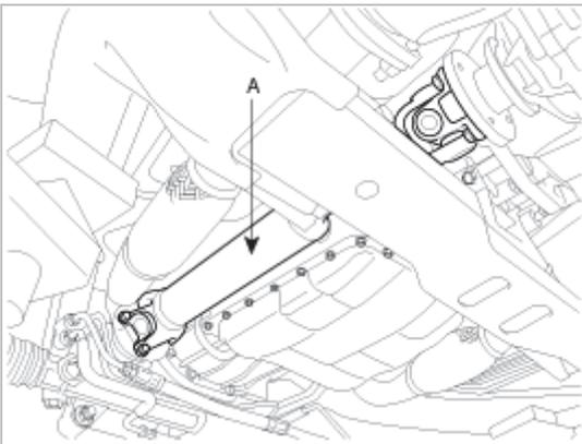
8. Remove the rear propeller shaft(A).
