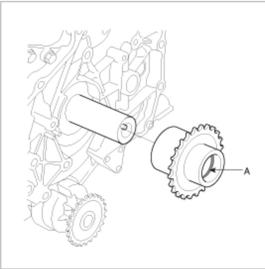
4. Align the timing mark of LH balance sprocket(A) with the timing mark of timing chain lower under cover(B).
