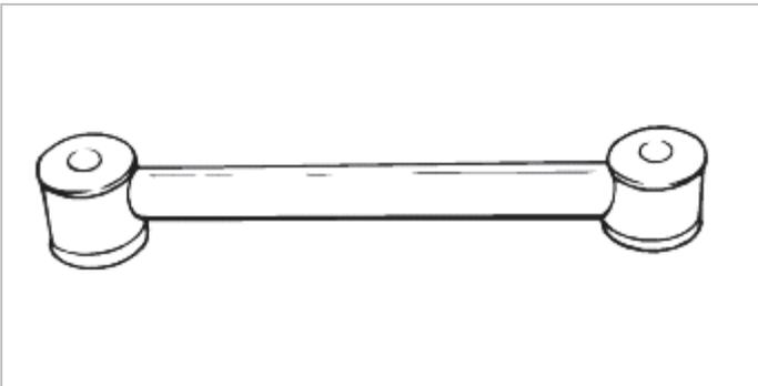
2. Inspect the lateral rod bushings for wear and/or deterioration.
