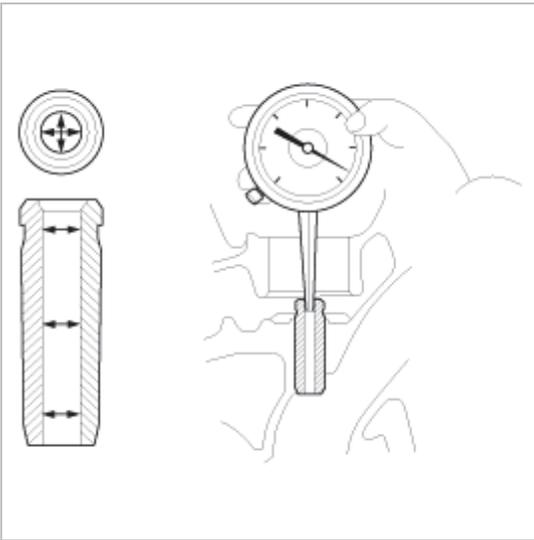
6. Measure valve stem to guide clearance(C) by subtract outer diameter of valve stem(B) from inner diameter of corresponding valve guide(A).
