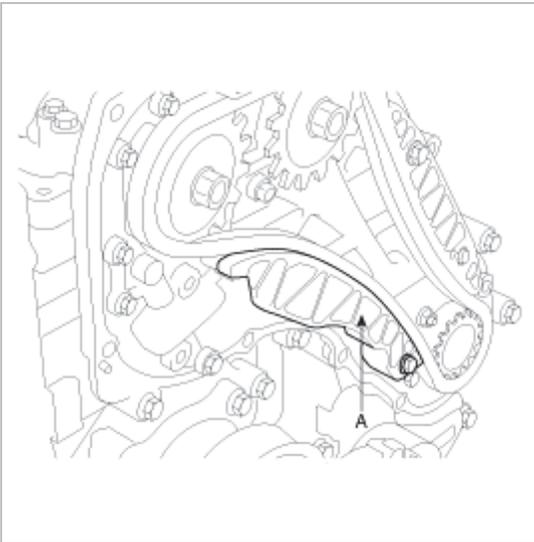
12. Install the timing chain auto-tensioner "C"(A), and remove the set pin(B) from the auto-tensioner.
