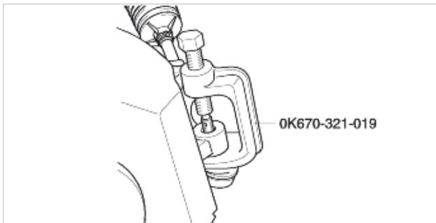
7. Remove lower arm cotter pin using a ball joint remover, and remove lower arm from steering knuckle.
