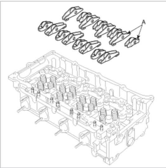
7. Install the camshaft carrier (A) on the cylinder head.
