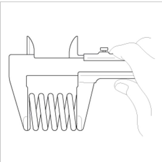
3. Check spring pressure, and replace it if necessary.
