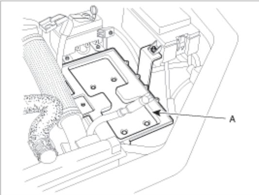
2. Drain the automatic transmission fluid after removing the drain plug (A).
