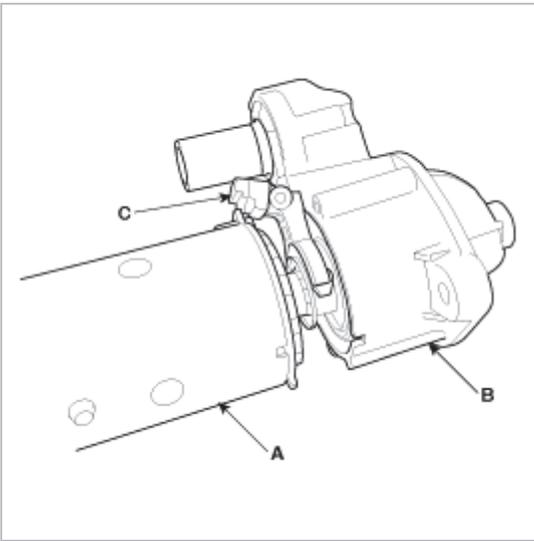
4. Remove the over running clutch assembly(A).
