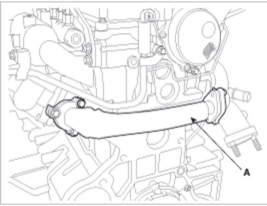
5. Install the high pump fuel hose bracket(A).
