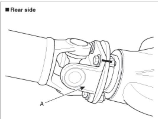
34. Remove the front propeller shaft(A).
