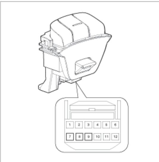
2. Measure voltage between terminals on the harness side connector when each function switch is ON (switch is depressed).
