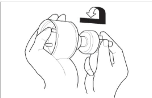
3. If the starter driver gear (B) is worn or damaged, replace the overrunning clutch assembly: the gear is not available separately.
