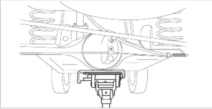
2. Remove the stabilizer link mounting nut.
