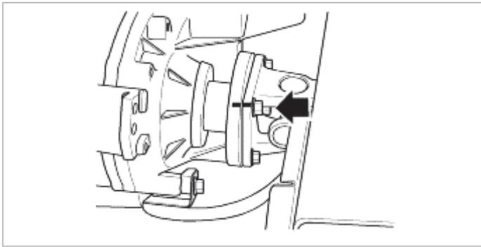
3. Connect rear propeller shaft flange to companion flange on transfer. (4WD)
