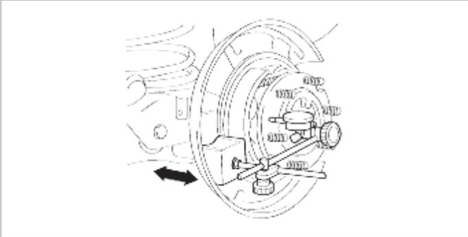
2. If the axle shaft end play exceeds the standard value, replace the bearing with a new one.
