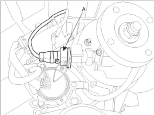
16. Remove the transfer case connectors(A). (4WD)
