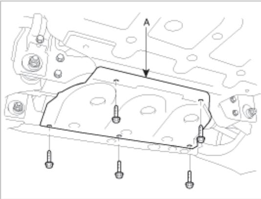
7. Remove the front propeller shaft(A). (4WD)
