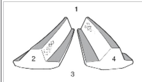
The drive pinion is positioned too far from the center of the drive gear.
