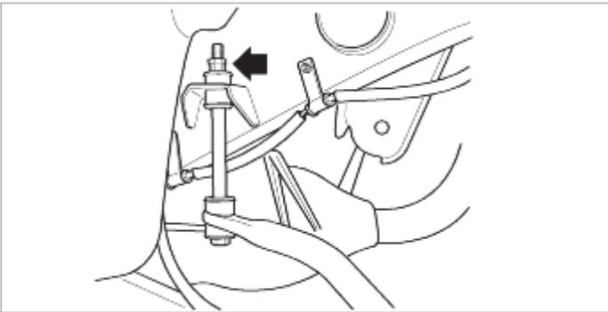
3. Remove the stabilizer bar bushing bracket.
