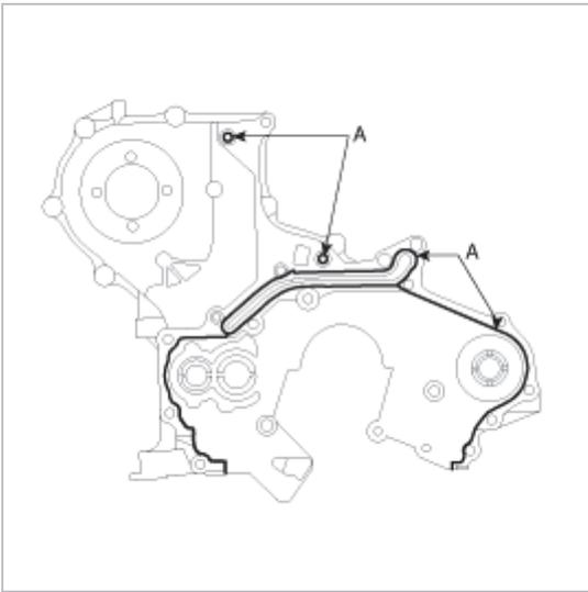
13. Install the timing chain lower under cover (A).
