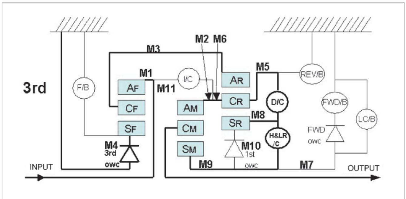
C. The high & low reverse clutch is coupled and the middle and rear sun gears are connected.
