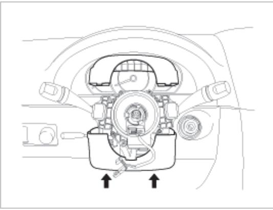
7. Unscrew the clock spring tightening screws. (4EA)
