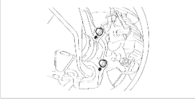
3. Remove two screws and remove brake rotor.
