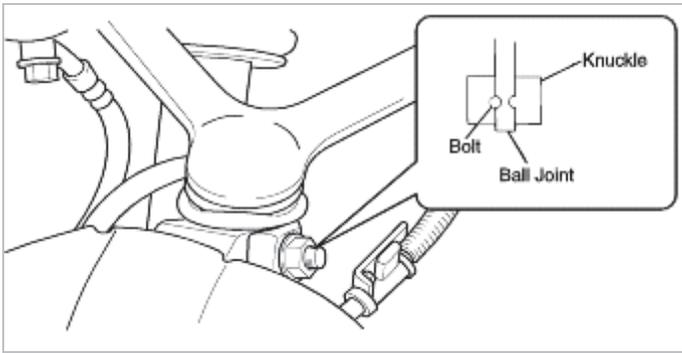
4. Tighten the upper arm bolts and nuts and then install brake hose brackets.
