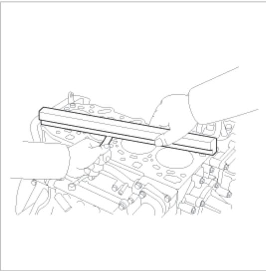
3. Check cylinder wall for scratches and seizure.
