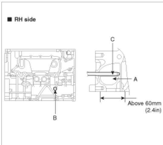
4. Install the space washer(A) from RH balance shaft.
