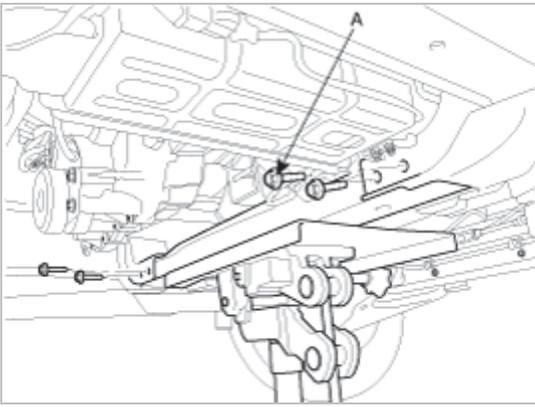
8. Install the clutch release cylindre(A) and transmission mounting bilt(B).
