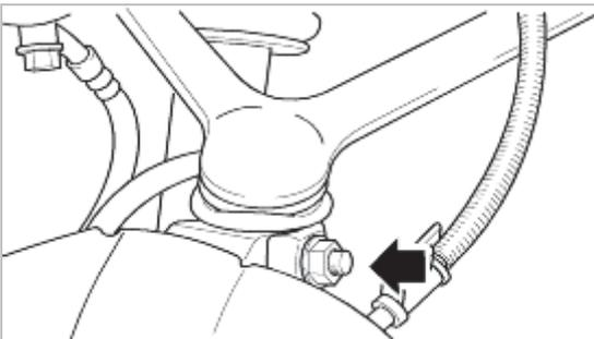
3. Remove tie rod end cotter pin and using a ball joint puller, remove tie rod end from steering knuckle.
