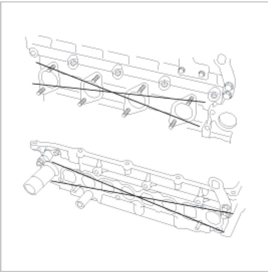
4. If distortion exceeds specification, grind surface or replace cylinder head.
