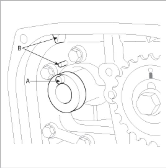
7. Align the timing marks of sprocket and chain when RH camshaft sprocket is not installed to the camshaft.
