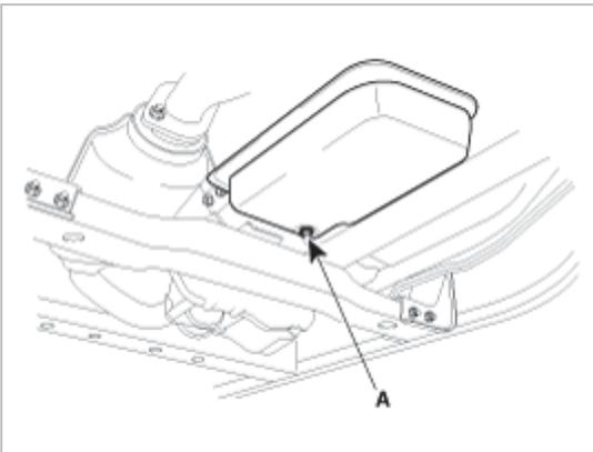
5. Remove the battery and battery tray(A).
