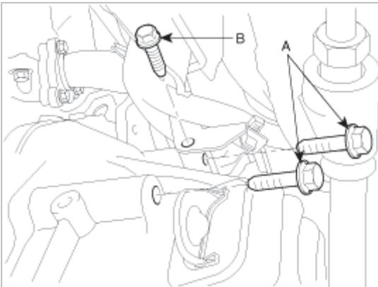
13. Remove the transmission mounting bolts(A).
