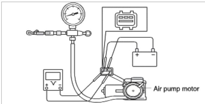
(2) Confirm that motor runs when battery has been connected. And check that motor stops when returned to specified pressure.
