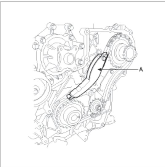
12. Install the timing chain auto-tensioner "A"(A), and remove a set pin(B) from the auto-tensioner.
