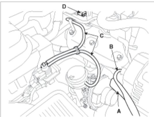
22. Disconnect the earth terminal and the glow plug connector(D).
