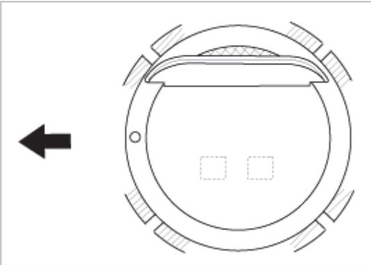
10. Insert the piston and connecting rod assembly from above the top of cylinder. Ensure that the front mark (A) on the piston crown and that (front mark) on the connecting rod face toward the front of engine (to the crankshaft pulley side).
