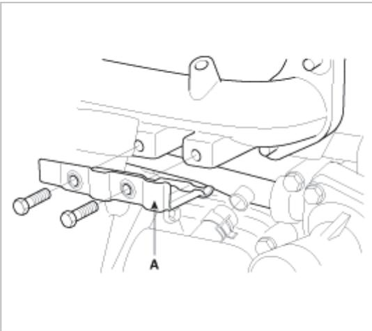
8. Install the oil separator(A).
