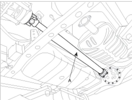
9. Remove the transmission lower mounting bolts(A).
