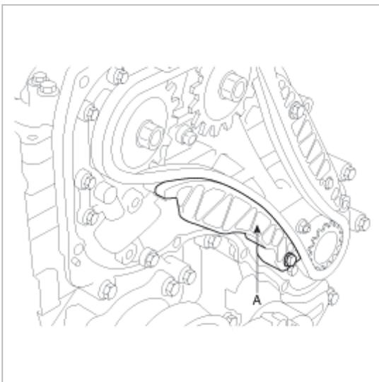
8. Remove the timing chain guide "C(1)(A), C(2)(B)".
