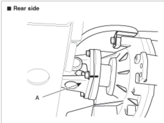
35. Remove the front exhaust pipe(A) and muffler(B).
