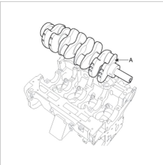
5. Check the main bearing, cap number. And then Install the main bearing (A) and bearing (B).
