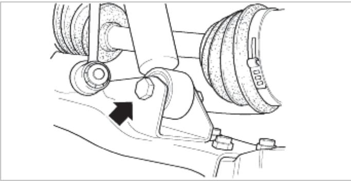
8. Remove the spring and shock absorber assembly from the vehicle as an assembly.
