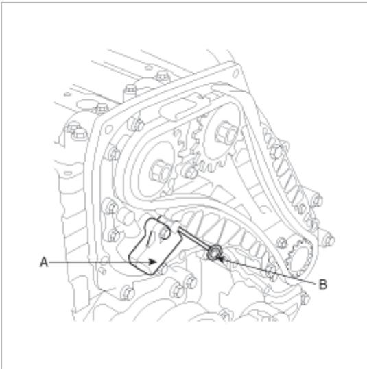
13. Assemble the high-pressure pump sprocket bolt.
