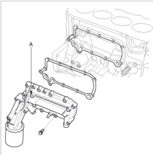
4. Install the engine oil filter.
