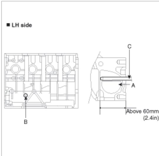
6. Assemble the upper bolt of timing chain guide "A"(A) tentatively.
