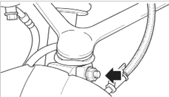
6. Remove the brake hose bracket and then the remove the upper arm bolts and nuts.
