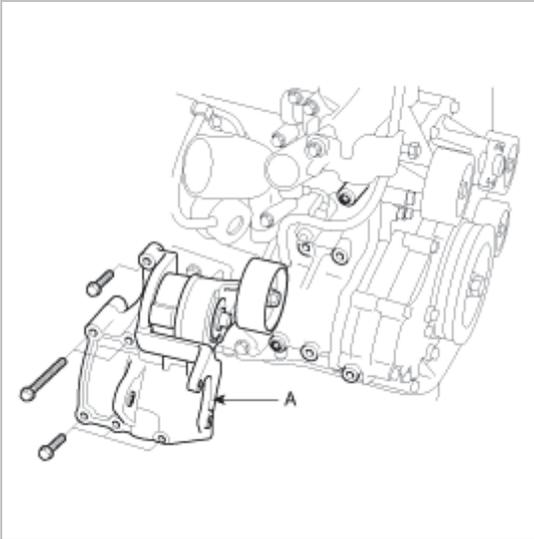
9. Remove the thermostat housing (A) and heater pipe (B).
