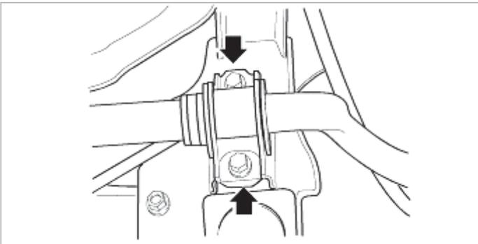
6. Remove the control link from the lower arm.
