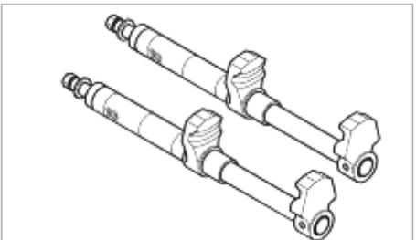
The illustration shows two identical coil spring compressors. Each tool consists of a long, cylindrical metal body with a threaded end on the left and a hook-like attachment on the right. The hook is designed to grip the top of a coil spring. The tools are shown from a perspective view, one slightly behind and to the right of the other. | For removal of front shock absorber spring |
