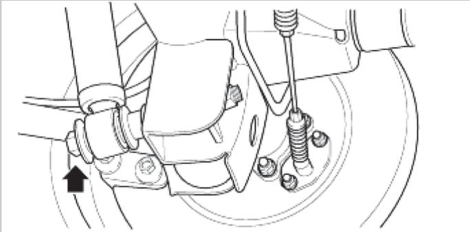
5. Loosen the upper arm bolts and remove the upper arm.
