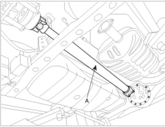
11. Install the front propeller shaft(A). (4WD)
