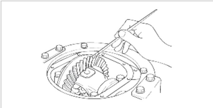
2. Insert a brass rod between the differential carrier and the differential case, and then rotate the companion flange by hand (once in the normal direction, and then once in the reverse direction) while applying a load to the drive gear so that some torque (approximately 25-30 kg-cm) is applied to the drive pinion.
