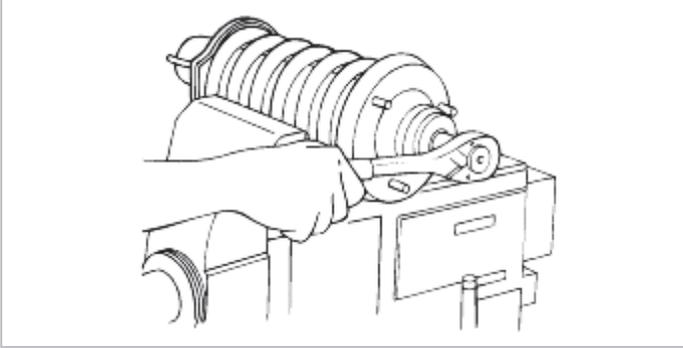
3. While still secured in a vise, compress the coil spring with SST.
