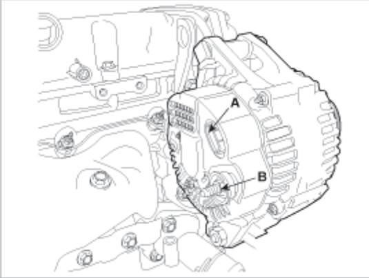
4. Remove the through bolt and the alternator(A).
