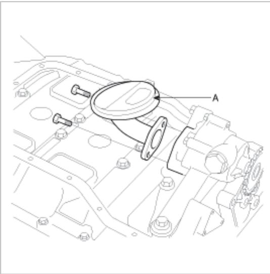
5. Remove the oil feed pipe (A) from the oil pump and bed plate.
