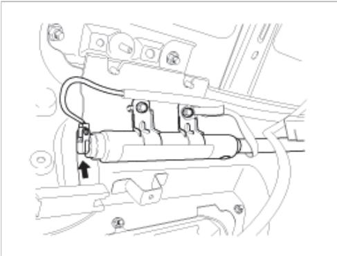
4. After loosening the mounting bolts(6EA) and nut (1EA) remove the curtain airbag.
