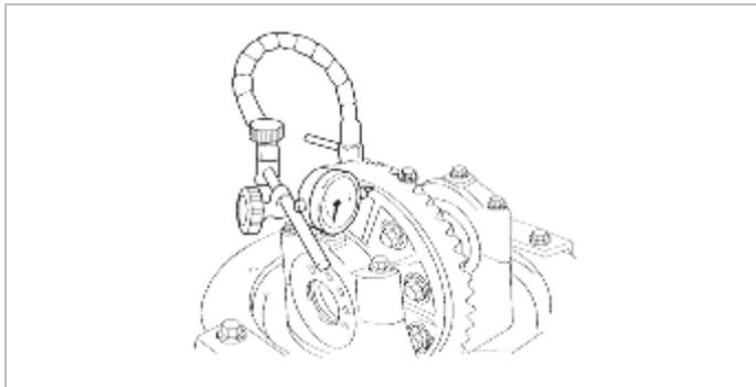
(3) Using the special tool (09521-43000), adjust the backlash to standard value by moving the side bearing nut as shown.
