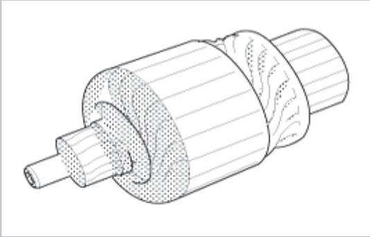
4. Measure the commutator (A) runout.
