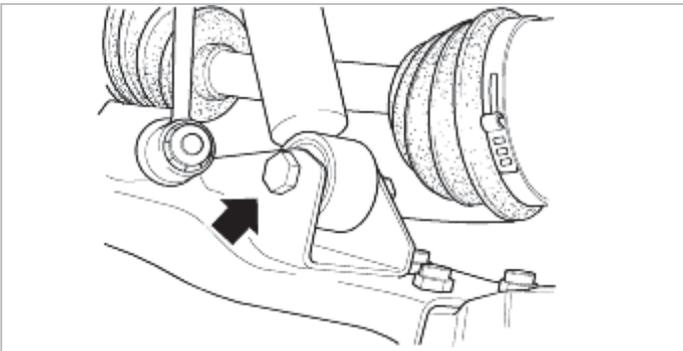
5. Position the upper arm to the frame brackets, insert the bolts and hand tighten the nuts.
