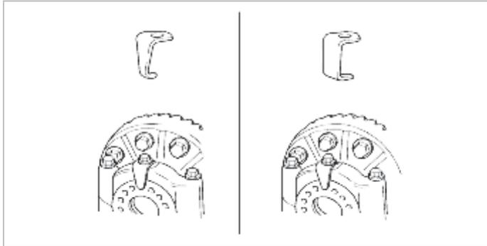
(6) Check the final drive gear tooth contact. If poor contact is evident, make adjustment.
