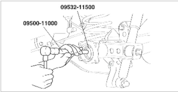
4. After installing the axle shaft, tighten the nut.
