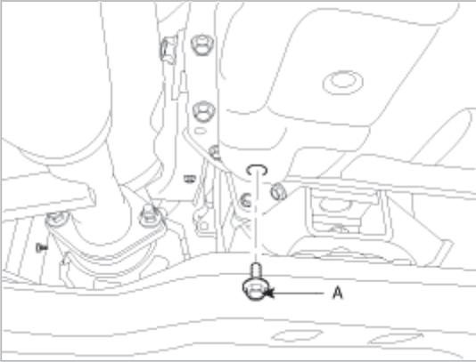
4. Install the drain plug via the gasket, and tighten it the specified torque.
