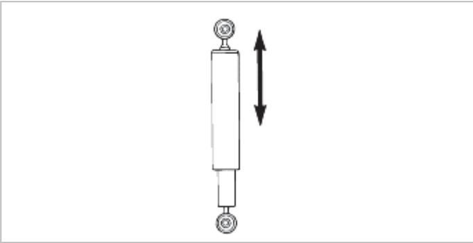
3. Inspect the shock absorber for a worn or deteriorated rubber bushing.
