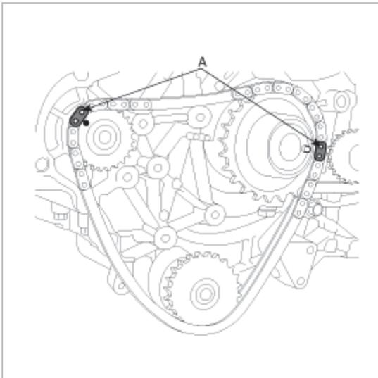
6. Assemble the RH balance shaft sprocket to the balance shaft tentatively.
