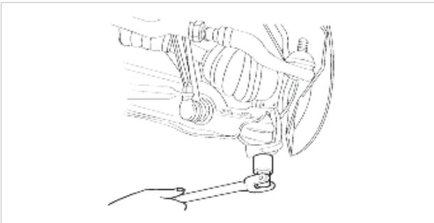
3. Attach tie rod end to knuckle, tighten nut, and install cotter pin.
