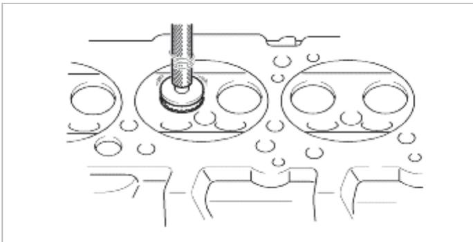
3. Apply a thin coat of Prussian blue to valve face.
