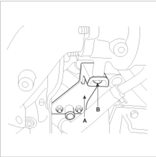
6. Remove the exhaust manifold(A).
