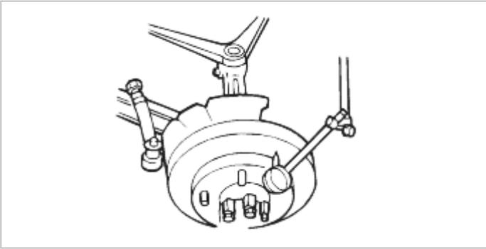
3. Turn rotor and read dial indicator for run out dimension.
