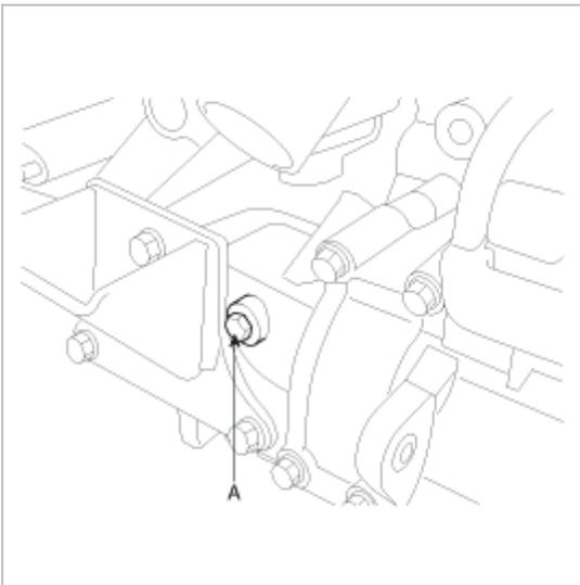
11. Apply the sealant(A) at the timing chain lower front cover.
