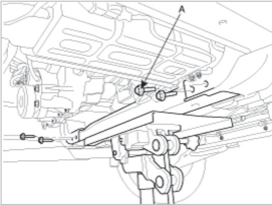
12. Remove the starter motor mounting bolts(A) and wire harness mounting bolt(B).
