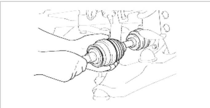
3. Remove the front propeller shaft.
