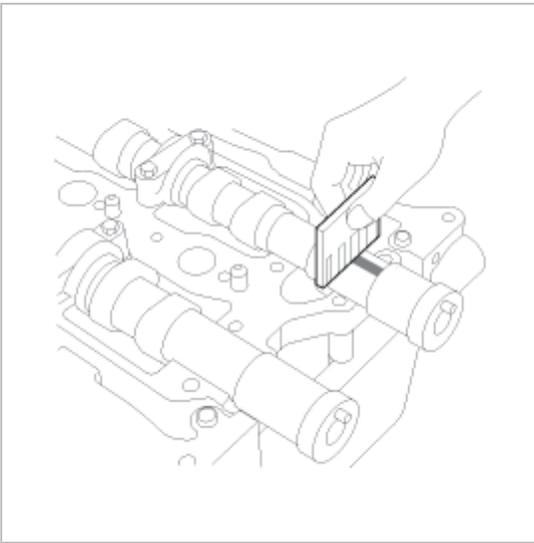
6. Check the cam lobes for damage. If the lobe is damaged or worn excessively, replace the camshaft.
