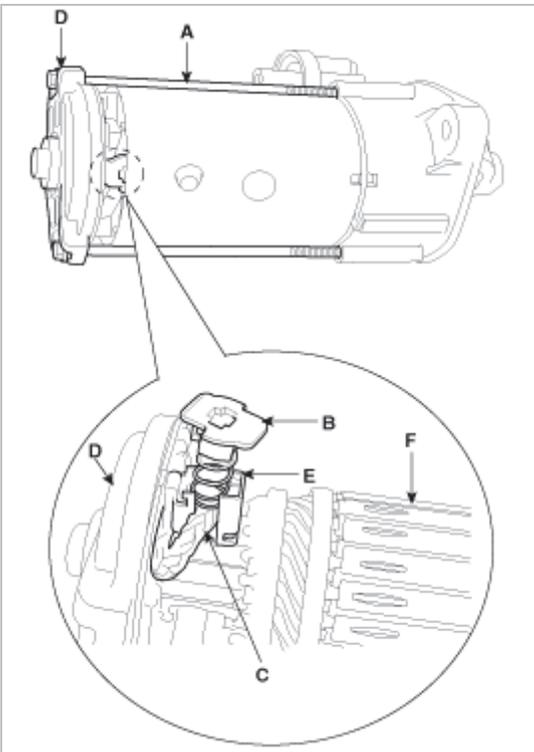
3. Remove the yoke assembly with the front bracket(B) and pinion shift lever assembly(C).
