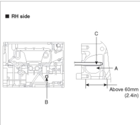
6. Loosen the RH balance shaft sprocket bolt(A).
