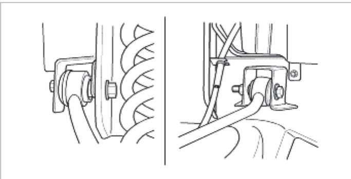
3. Install the upper arm ball joint into the top of the steering knuckle and tighten the side bolt and nut.
