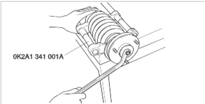
4. Remove the piston rod nut and each part as below.
