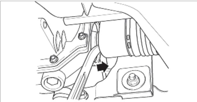
6. Remove the drive shaft from the knuckle
