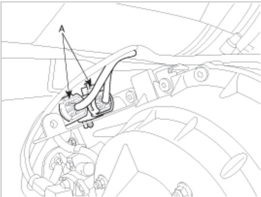
17. Remove the transmission upper mounting bolts.
