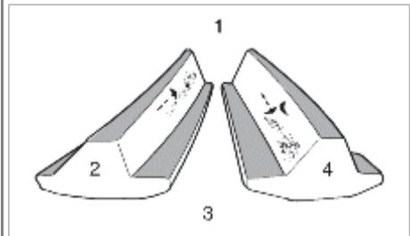
Increase the thickness of the pinion height adjusting shim, and position the drive pinion closer to the center of the drive gear.
