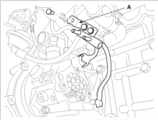
6. Install the high pipe bracket(A) and coolant temperature sensor connector(B).
