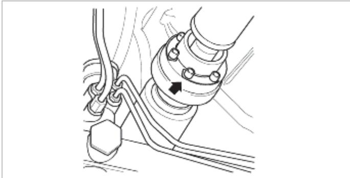
2. Connect front propeller shaft flange to companion flange on transfer (4WD).
