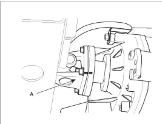
9. Remove the front muffler (A).
