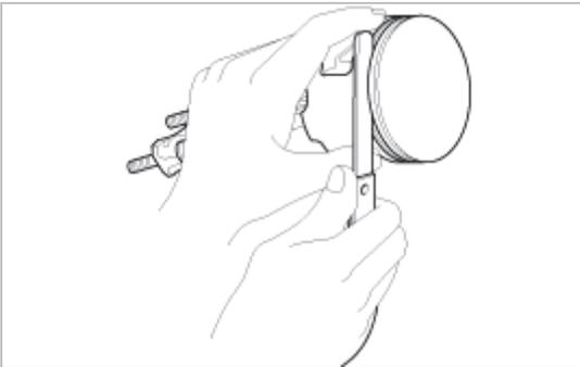
4. Place a piston ring in the cylinder bore and set it square by pushing it down with piston.
