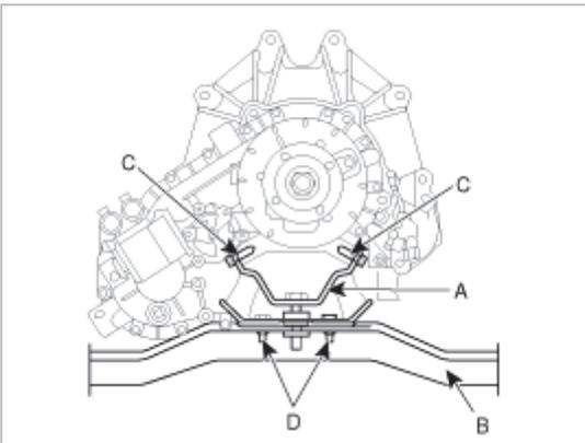
5. Install the transmission housing fixing bolts.
