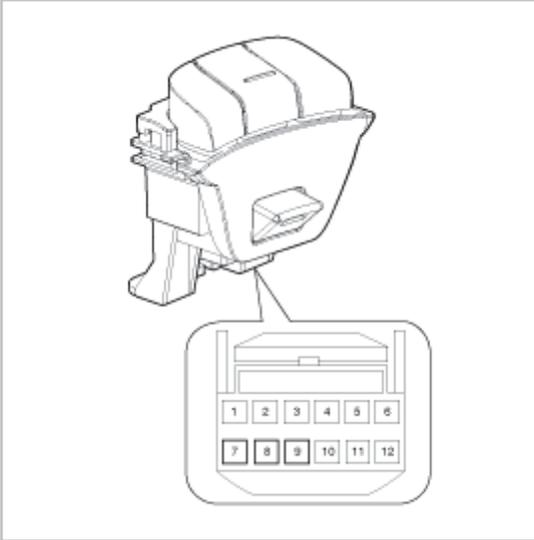
2. Measure resistance between terminals on the control switch when each function switch is ON (switch is depressed).
