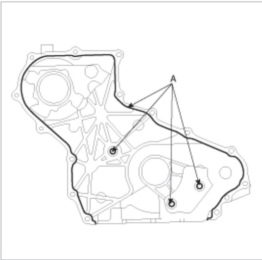
12. Install the timing chain lower front cover(A).
