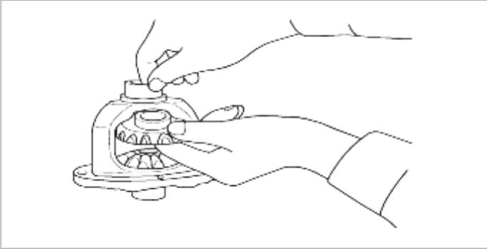
3. Insert a wedge in the side gear and measure the differential gear backlash with a dial indicator on the pinion gear.
