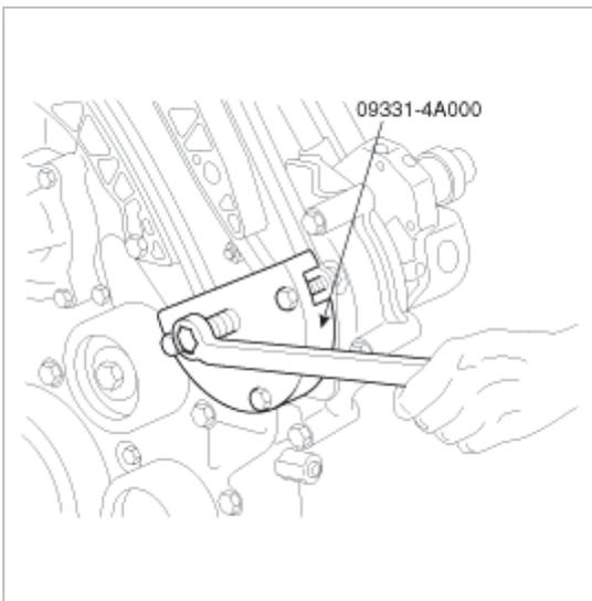
6. Remove the timing chain auto-tensioner "C"(A).
