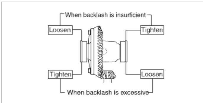
(4) Using the special tool (09521-43001) to apply the preload, turn down both right and left side bearing nut on half the distance between centers of two neighboring holes.
