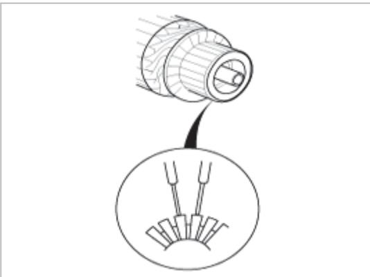
6. Check with an ohmmeter that no continuity exists between the commutator (A) and armature coil core (B), and between the commutator and armature shaft (C). If continuity exists, replace the armature.
