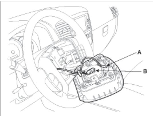
4. Release the connector locking pin, then disconnect the driver airbag module connector(B).
