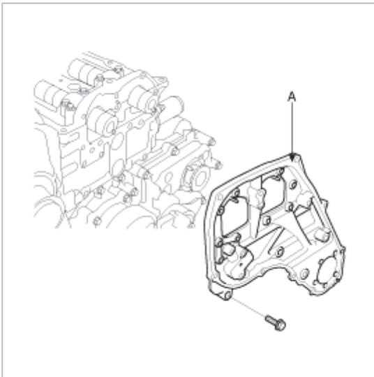
5. Assemble the LH camshaft sprocket(A) tentatively, and align the timing mark with that of timing chain upper under cover.
