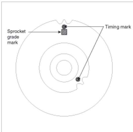
3. Install the crankshaft sprocket as the timing mark of crankshaft sprocket aligns with the timing mark(A) of lower under cover(B), at which No.1 piston locates at the top dead center of compression stroke.
