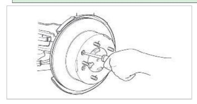
3. After turning the pin to coincide with hole of spring cap, remove the shoe hold spring.
