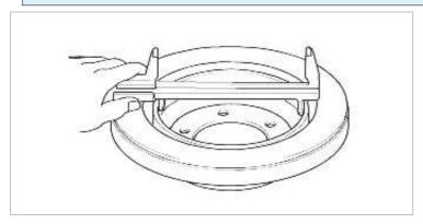
2. Measure the brake lining thickness.
