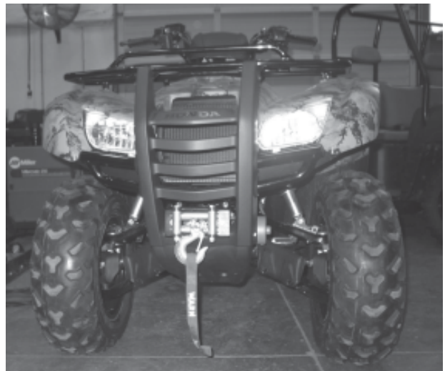
Figure 24 Winch and Mount Installed
