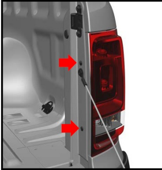
Fig. 4.1.1.1: Removal of the tail light (Figs. 1, 2 and 3)
