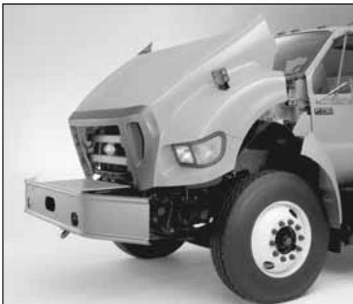
Standard Tilting Hood — allows for easier servicing of the engine area
