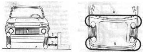
Fig 55. Checking front end alignment
