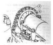
Fig 32. Setting No. 4 Cylinder piston in TDC
