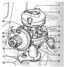
Figure 41. Ignition distributor. 1- noise resistor suppressor, 2- rotor, 3- breaker contacts, 4- screw, 5-slot, 6- terminal, 7- spring catch, 8- capacitor, 9-scale, 10- bracket, 11- nut, 12- body, 13- vacuum spark timer, 14- lubricator, 15- cam
