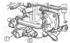
Fig 37. Idling system adjustment screws: 1-Idle speed screw limiting bushing, 2- idle mixture screw limiting bushing.
