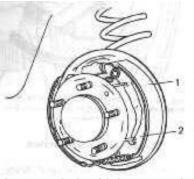
Fig 61. Rear brake with drum removed. 1- friction lining, 2- brake shoe
