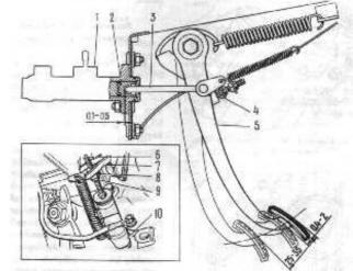
Fig 45. Adjusting Clutch control mechanism. 1- Clutch master cylinder, 2- pushrod piston, 3- pushrod, 4- pedal travel stop, 5- clutch pedal, 6- operating cylinder pushrod, 7- clutch release fork, 8- nut, 9-locknut, 10- operating cylinder.
