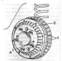
Fig 60. Rear Brake. A-holes, 1-bolts, 2-brake drum
