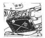
Fig 46. Gearbox. 1- check hole plug, 2- drain hole plug
