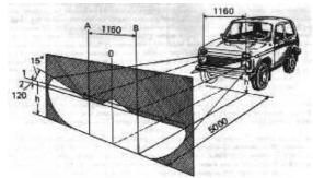
Fig 67. Aiming headlight lower beam
