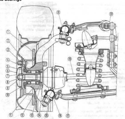
Fig. 51. Front Wheel: 1 - brake disc; 2 - hub; 3 - outer roller bearing; 4 - outer seal protective ring; 5 - outer seal; 6 tapered bushing; 7 - hub nut; 8 - hub cap; 9 - propeller shaft drive end; 10 - outer seal demounting ring; 11 - inner roller bearing; 12 - inner seel demounting ring; 13 - inner seal; 14 - inner real protective ring; 15 - steering knuckle; 16 - lower wishbone ball support; 17 - lower wishbone; 18-propeller shaft; 19-upper wishbone ball support; 20 - shims
