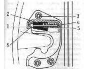
Fig 72. Door lock striker plate. 1- striker plate, 2- block, 3, bolt, 4-pin, 5- spring, 6 bushing.
