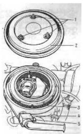
Figure 35. Air Cleaner 1- nut, 2-cover, 3- filter, 4- thermo-regulator, 5-handle
