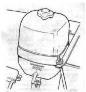
Fig 38 Cooling system expansion tank
