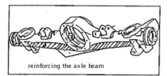
• Reinforce the anchorage points of the rear shock absorbers and the lower ties of the axle with a plate.
