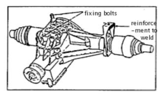
The power train must be in good condition and not have any significant play. The rubber boots must be changed if they show signs of leakage or damage. If used for long periods with damaged boots it will be necessary to change the complete transmission.
