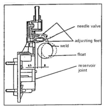
**Important :** it is essential to redo the tin welds of the float leg. These have a tendency to break under vibration.
