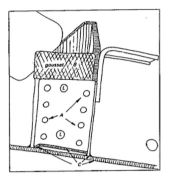
B. Double the existing plate by a support in 2mm plate – see the diagram below – and weld this all around the perimeter.
