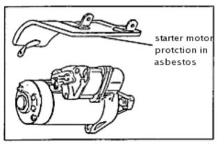
• Check and lock the solenoid bolts.
