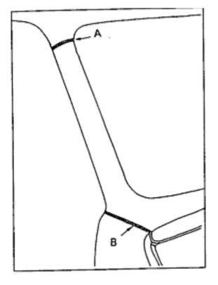
Using 2.5mm plate, bracket the cheek of the wing and apron (fig A)
