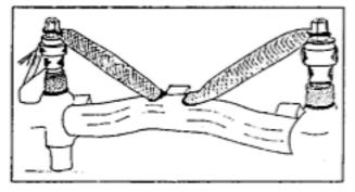
to measure in place) and about 25mm long should be slipped into place in a way that leaves room for the tightening collars. Replace the original mounting bolts with upper and lower ball joints with BTR bolts and Nylstop nuts.
