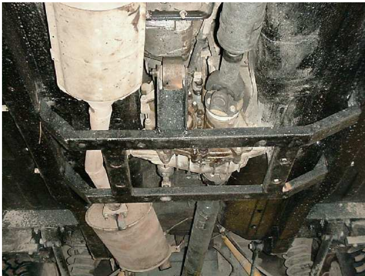
And here's the all-in-one's mounts (bolted through the chasis)
