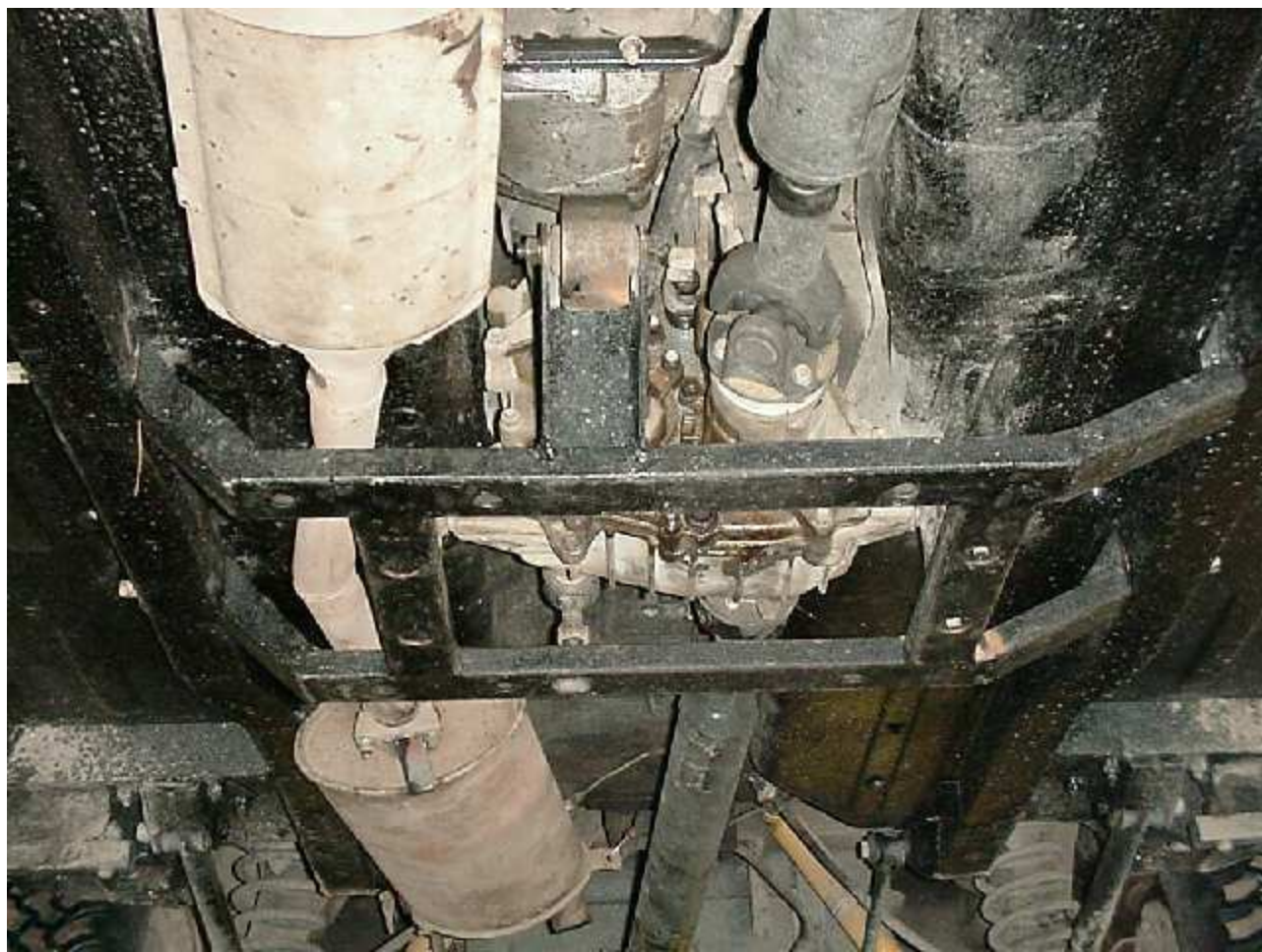
And here's the all-in-one's mounts (bolted through the chassis)
