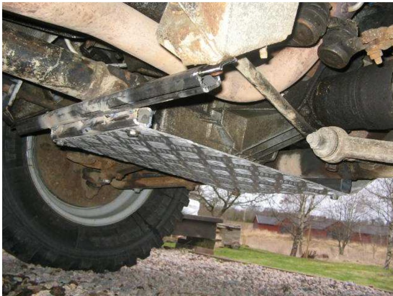
Front diff and sump guard (no roll-bar)
