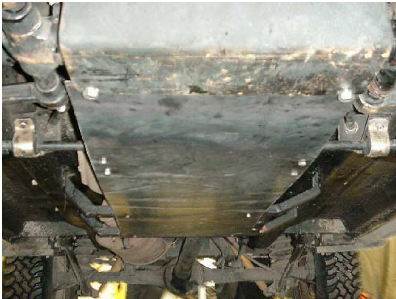
All-in-one: Sump, front diff, gearbox and TC guard (with roll-bar)
