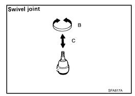
2. Check condition of dust cover. If it is cracked excessively, replace as a complete unit.
