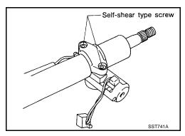
Install self-shear type screws, then tighten until heads break off
