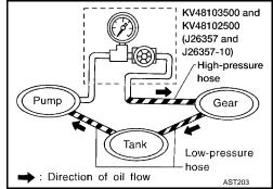
4. Check pressure with steering wheel fully turned to left and right positions while idling at 1,000 rpm.
