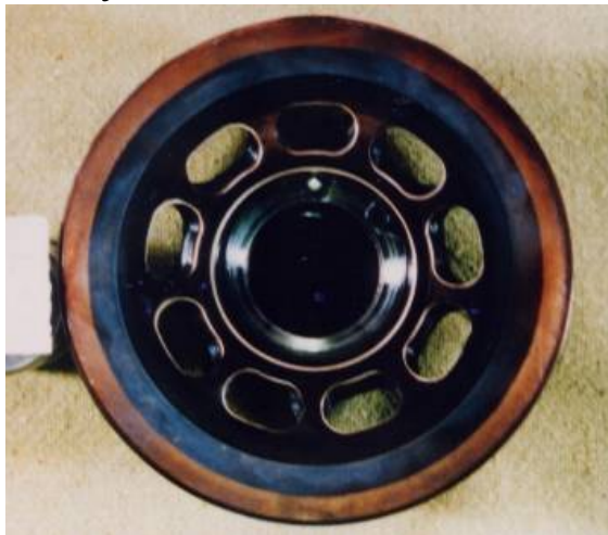
Corroded Cylinder Block
