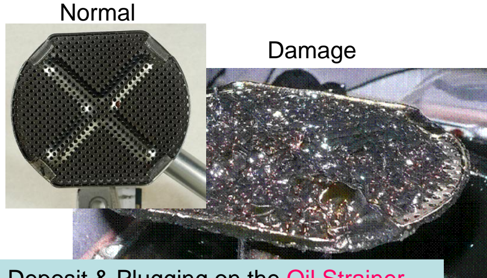
Deposit & Plugging on the Oil Strainer
