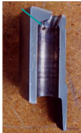
Cavitation and Wear of Cylinder Bore
