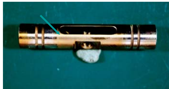
Lacquer on Servo Piston Caused Flow Reduction
