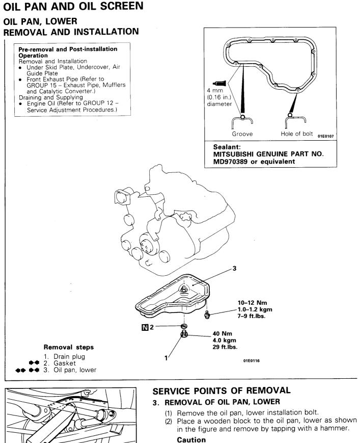
The use of an oil pan remover (MD998727) can damage the oil pan, upper (aluminum made).
