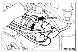
(2) Insert a paper clip into the 1-pin connector between the primary side of the ignition coil and the noise filter. The connector should not be disconnected.
