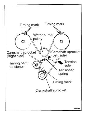
(2) When the timing belt is to be reused, in order to allow reinstallation of the belt so that it travels in the same direction as before it was removed, mark the direction of travel with an arrow before removing it.
