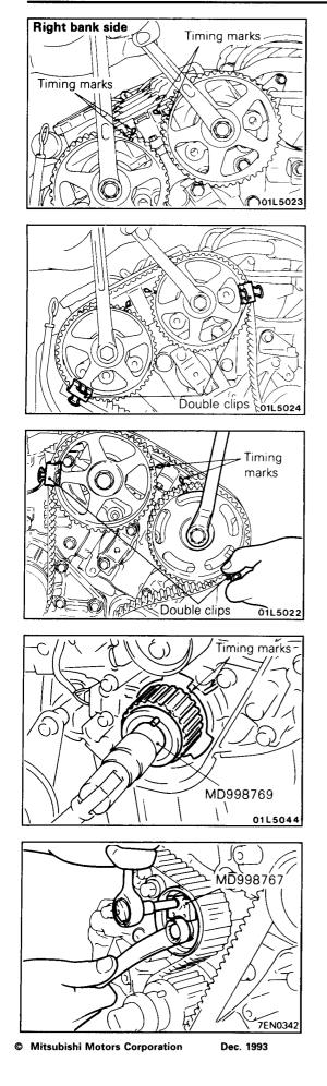
(3) Align the timing mark of the right bank side camshaft sprocket and support it not to rotate with a closed wrench.
