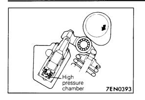
If the air mixed in with the oil due to the above reasons gets into the high pressure chamber of the auto-lash adjuster, the air inside the high pressure chamber will be compressed when the valve is open and the auto-lash adjuster will overcompress, resulting in an abnormal noise when the valve closes. This is the same effect as if the valve clearance is adjusted to be too large by mistake.
