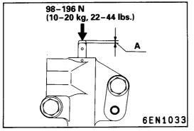
**11.REMOVAL OF CRANKSHAFT PULLEY**
