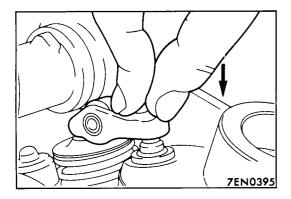
6. If the rocker arm moves down when it is pushed, replace the auto-lash adjuster.
