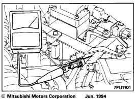
IGNITION TIMING INSPECTION AND ADJUST-MENT <SOHC-12 VALVE>
