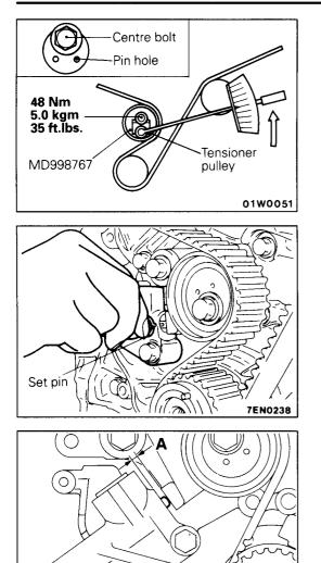
(6) Loosen the centre bolt on the tensioner pulley. Using the special tool and torque wrench, apply tensioning torque to the timing belt and, at the same time, tighten the centre bolt to specification.
