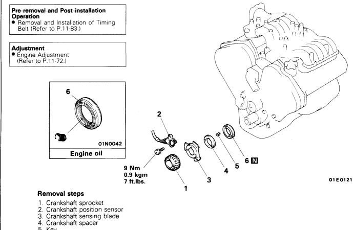
5. Key 6. Crankshaft front oil seal
