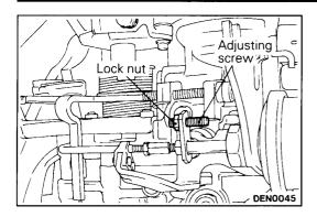
(7) Check the engine speed when a negative pressure of 87 kPa (650 mmHg, 26 in.Hg) is applied.
