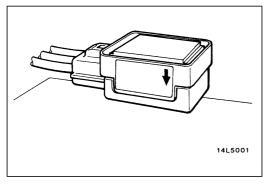
(3) With the special tool still connected, secure the G-sensor so that the arrow mark on the sensor mounting surface faces straight down, and then take a reading of the following output voltage between terminals (2) and (3).
