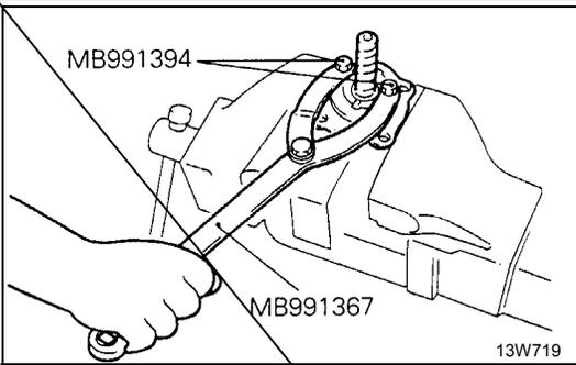
**13. INSTALLATION OF LOCK NUT**
