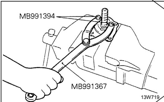
**20. REMOVAL OF MAIN SHAFT/21. BEARING RACE/22. CAGE/23. BALL**
