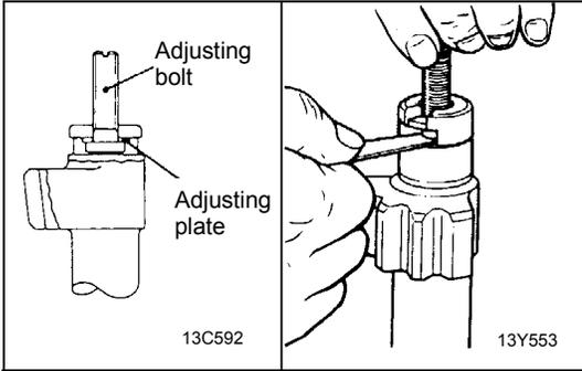
**24. INSTALLATION OF ADJUSTING PLATE/25. ADJUSTING BOLT**
