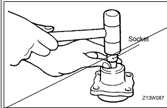
**◀G▶ BEARING AND OIL SEAL REMOVAL**
