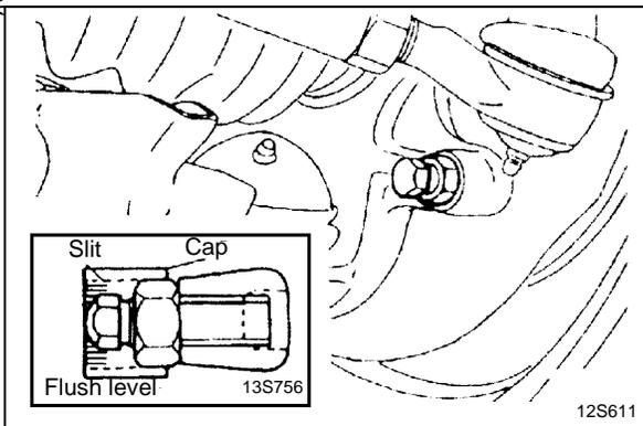
**CHECKING STEERING GEAR OIL LEVEL (MANUAL STEERING)**
