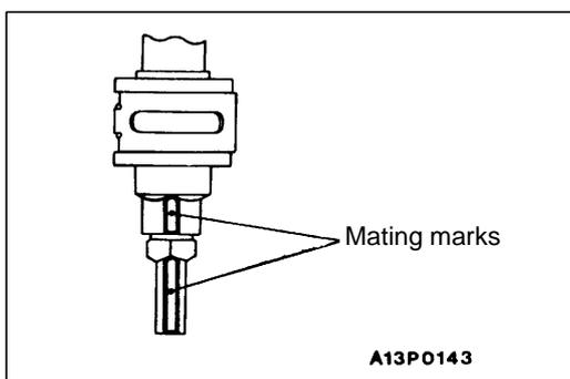
2. Align the marks on the pressure hose and pressure tube, and install the pressure hose.
