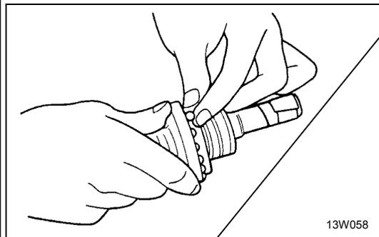
(6) When installing the main shaft, connect it to the valve housing while pressing the bearing race so that the balls do not come out.
