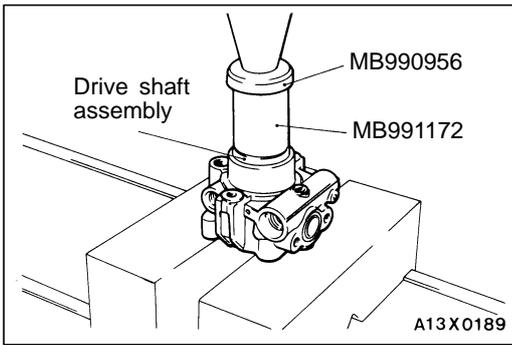
**▶B◀ DRIVE SHAFT ASSEMBLY INSTALLATION**
