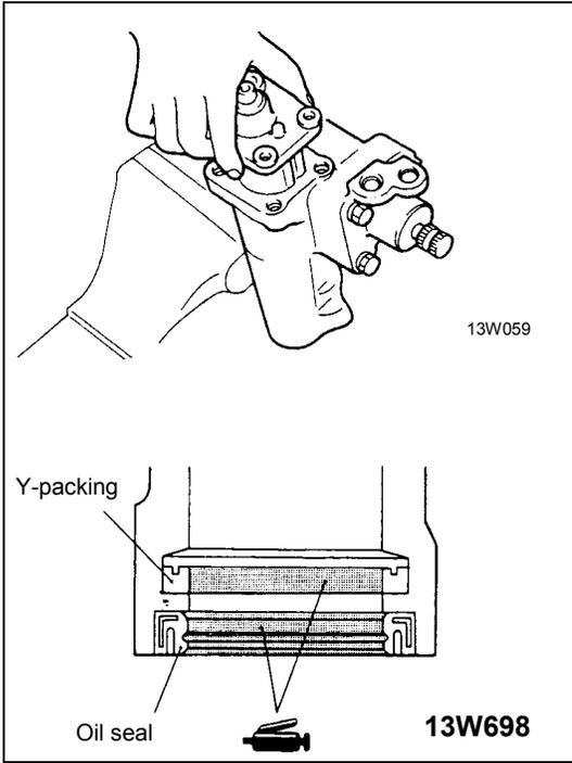
**29. INSTALLATION OF SIDE COVER AND CROSS-SHAFT ASSEMBLY**
