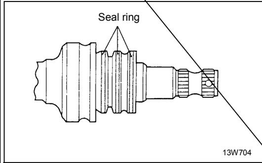
**8. INSTALLATION OF SEAL RING**
