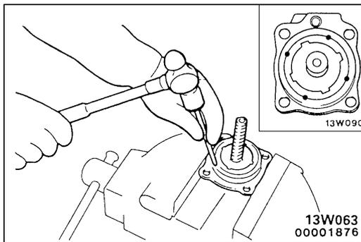
2. Use a punch to crimp the circumference of the lock nut so as to secure the lock nut.
