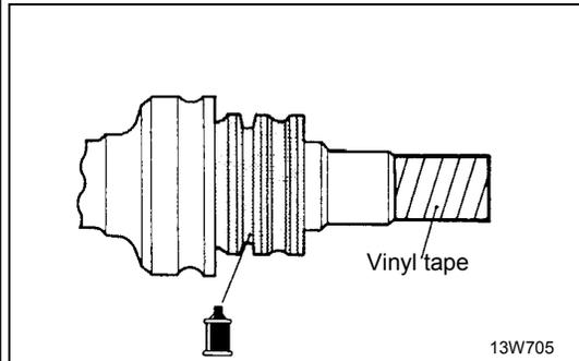
**9. INSTALLATION OF CAGE/10. BALL/11. BEARING RACE/12. MAIN SHAFT**
