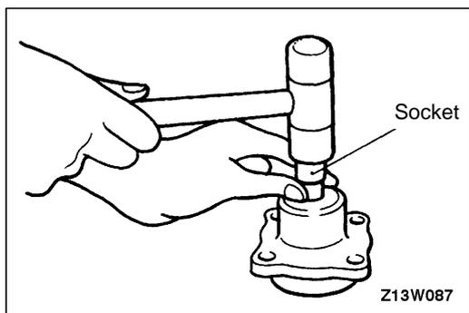
**◀G▶ BEARING AND OIL SEAL REMOVAL**
