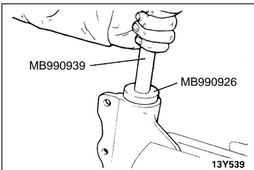
**REASSEMBLY SERVICE POINTS****▶A▶ OIL SEAL INSTALLATION**
