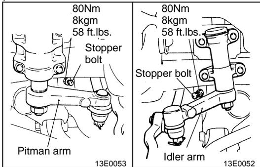
2. If the steering angle is outside the standard value, after checking the toe-in, (Refer to GROUP 33-Service Adjustment Procedures), adjust the steering angle with the stopper bolt.
