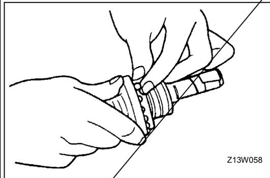
**►E◄ CAGE, BALLS, BEARING RACE AND MAINSHAFT INSTALLATION**
