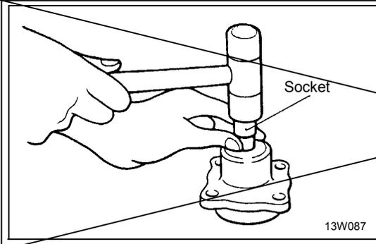
**27. REMOVAL OF BEARING/28. OIL SEAL**
