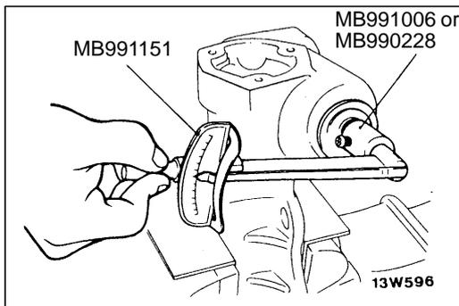
**►D◄ MAINSHAFT STARTING TORQUE ADJUSTMENT**
