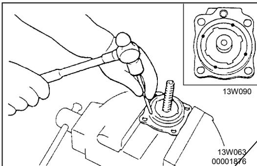
2. Use a punch to crimp the circumference of the lock nut so as to secure the lock nut.
