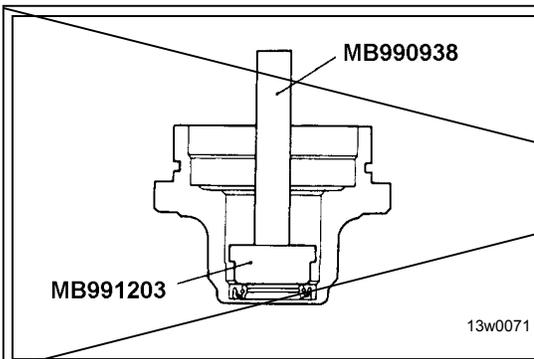
4. INSTALLATION OF OIL SEAL
