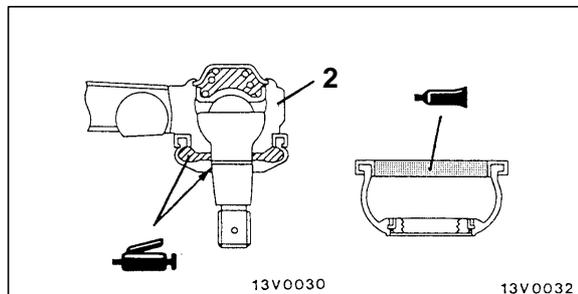
Sealant: 3M ATD Part No.8661 or equivalent
