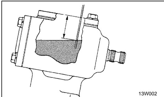
**STEERING GEAR OIL LEVEL CHECK (MANUAL STEERING)**
