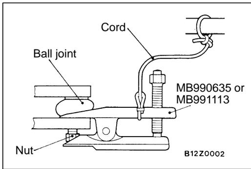
**REMOVAL SERVICE POINT****◀A▶ PITMAN ARM AND RELAY ROD DISCONNECTION**
