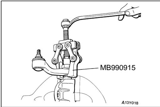
**DISASSEMBLY SERVICE POINTS****◀A▶ PITMAN ARM REMOVAL**
