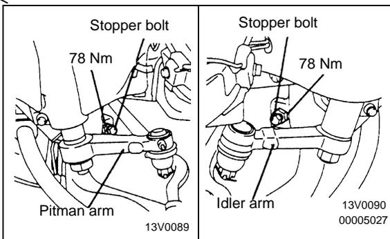
2. If the steering angle is outside the standard value after checking the toe-in (refer to GROUP 33A – On-Vehicle Service), adjust the steering angle with the stopper bolt.
