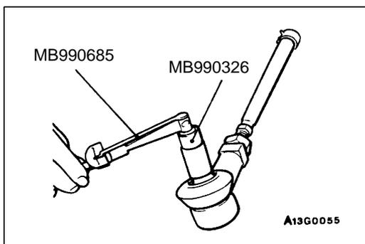
2. Move the ball joint stud several times and install the nut on stud. Measure ball joint starting torque with special tools.
