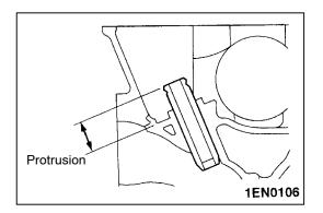
(3) Press-fit the valve guide until it protrude specified value (SOHC: 14 mm, DOHC: 19 mm) as shown in the illustration.
