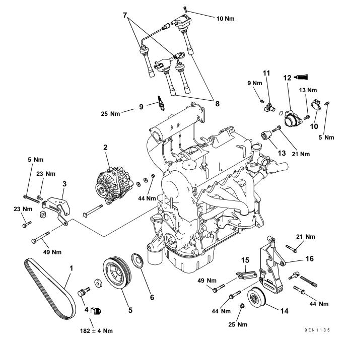
**REMOVAL AND INSTALLATION <SOHC for other than PAJERO io>** (Engines without distributor)
