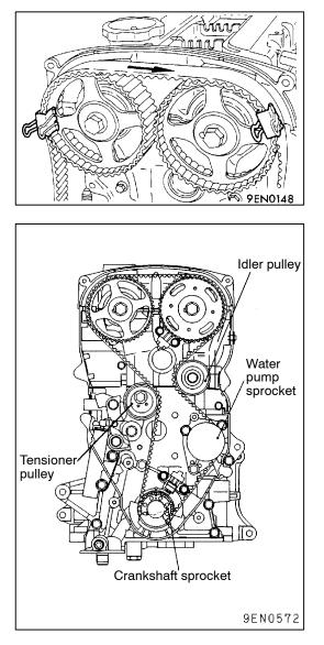
(6) Secure the timing belt with a paper clip at the illustrated position.
