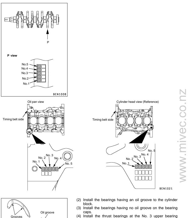
(4) Install the thrust bearings at the No. 3 upper bearing with the grooved side towards the crank web.
