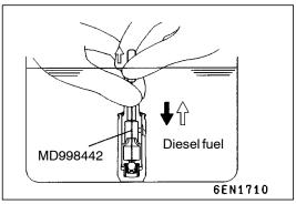
(4) Remove the lash adjuster from the container. Then, push down the steel ball gently and push the plunger to eliminate diesel fuel from the pressure chamber.
