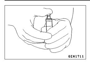
(9) Remove the lash adjuster from the container, then stand the lash adjuster with its plunger at the top. Push the plunger firmly and check that it does not move. Also, check that the lash adjuster's height matches that of a new lash adjuster.
