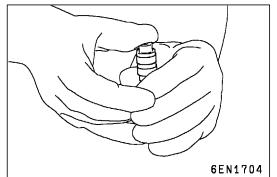
(6) Remove the lash adjuster from the container. Then, push down the steel ball gently and push the plunger to eliminate diesel fuel from the pressure chamber.
