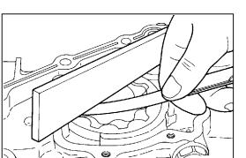
(2) Check the side clearance. Standard value: 0.04 - 0.10 mm
