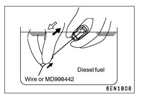
(4) Remove the lash adjuster from the container. Then, push down the steel ball gently and push the plunger to eliminate diesel fuel from the pressure chamber.
