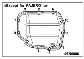
(4) Tighten the lower oil pan mounting bolts in the sequence shown in the illustration.
