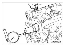
(8) After installing the bearing caps, make sure that the crankshaft turns smoothly and the end play is correct. If the end play exceeds the limit, replace crankshaft bearings.
