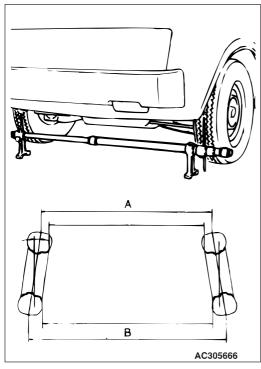
Using a toe-in gauge, measure toe-in. Toe-in = B – A
