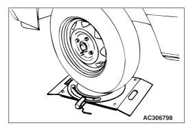
4. Use a turning radius gauge to check that the steering angle is at the standard value.
