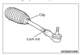
1. Adjust the toe-in by undoing the clip and lock nut, and turning the left and right tie rod turnbuckles by the same amount (in opposite directions).
