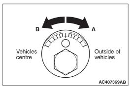
2. How to read this table (example). If the camber difference –0°35' and the caster difference is 0°17' by comparing the measurement value with the standard value, rotate the front adjusting cam by 1.5 graduations and the rear adjusting cam by 2.5 graduations to the opposite direction against the "A" direction.
