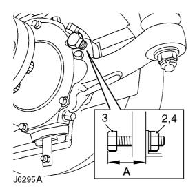
**1.** Measure stop bolt protrusion 'A'. Refer to table for correct setting.
