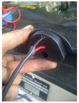
• Once in the switch, employ 2 of your butt connectors and join the new cable to the switch cables you've cut
