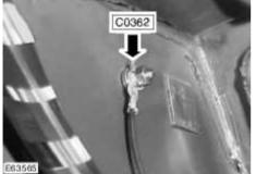
8. If there is no continuity (or intermittent continuity when the wire is flexed), repair as necessary and ensure the wire is correctly crimped and soldered.
