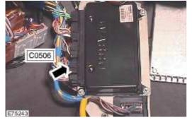
4. Inspect both connectors for moisture ingress or corrosion and correct as follows:
