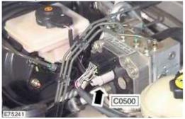
CAUTION: Connector pins must only be renewed one at a time to ensure the pins are returned to the correct position.
