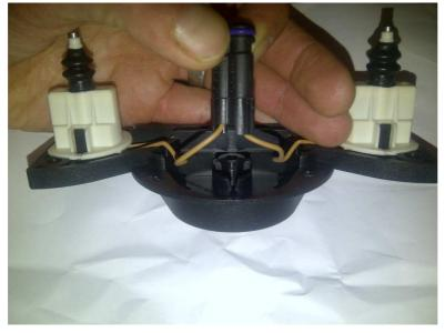
• Cut the connector off as close to the housing as possible so you have enough wire to play with (either if a new or old SVS).
