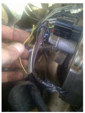
• You can now cut down your twin core to length...I took the red trace of my twin core and used another connector to join the two. Tape it and conduit it.
