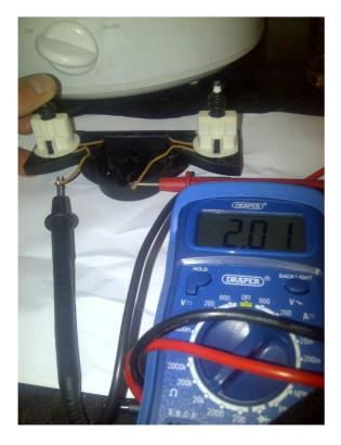
Reading 2...1 switch closed (push one switch down)-PASS
