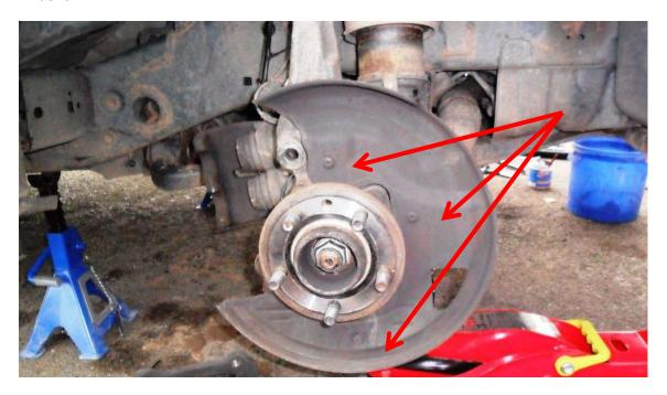
I then removed the brake back shield, although this isn't absolutely necessary, it helps provide better access.
