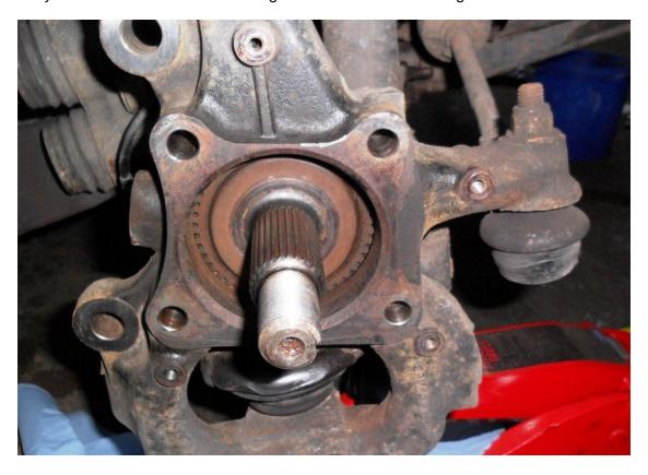
7, The new hub simple slides on to the drive shaft splines, I applied some copper slip grease, it is not a must, but will make dismantlement 'next time' a whole lot easier!!
