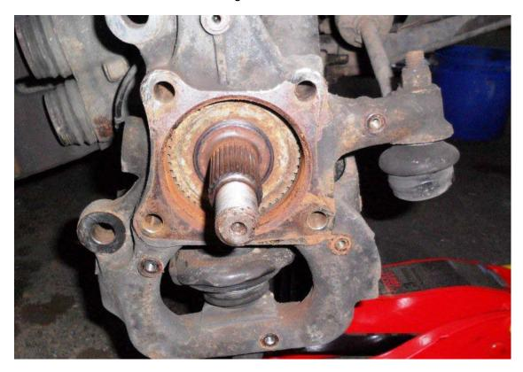
I then cleaned up the hub/axle mating faces, the splines on the drive shaft and any other rusty areas as much as I could using a wire brush and cleaning solvent.
