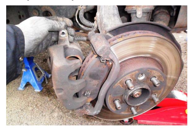
3, Remove the wheel rotation sensor (carefully, as easily breaks) it may be rusted in !!
