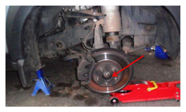
The jack is only supporting the weight of the hub NOT the vehicle, this is firmly sitting on the axle stand.
