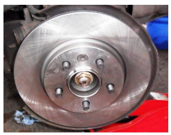
9, Refit the brake calliper anchor, calliper, pads, wheel sensor etc, and apply a smear of copper slip to the disc wheel spigot (this prevents the wheel from becoming 'welded' by corrosion to the hub.
