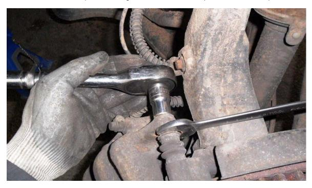
The calliper will hinge outwards allowing access to the pads. Support the whole calliper up out of the way using the cable ties onto the upper suspension arm, being careful not to kink/damage the hoses or cabling to the wheel sensor.
