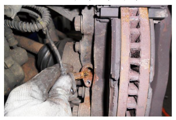
4, Remove the brake calliper anchor bolts, (the  $2^{\rm nd}$  one is arrowed).
