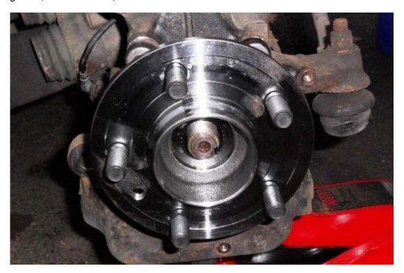
The hub is then secured with the 4 No retaining bolts, tighten to 115Nm, fit the drive shaft retaining nut 'hand tight'
