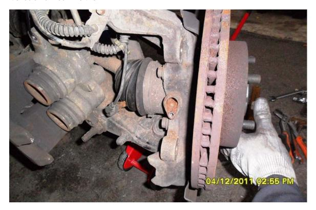
5, The next task is to remove the disc, this is secured by a 'Torx' bolt, which can be difficult to release and can strip easily, I used a hammer impact driver.
