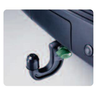
Quick Release Tow Bar KNB500013 Lockable for security. Easily removed. Tow ball height 400mm from ground. 3,500kg trailer load capacity (250kg trailer nose load).
