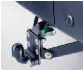
Multi-Height Tow Bar VUB501430 Four different towing heights. Lowest tow ball height 350mm from ground. Highest tow ball height 500mm from ground. 3,500kg trailer load capacity (250kg trailer nose load).
