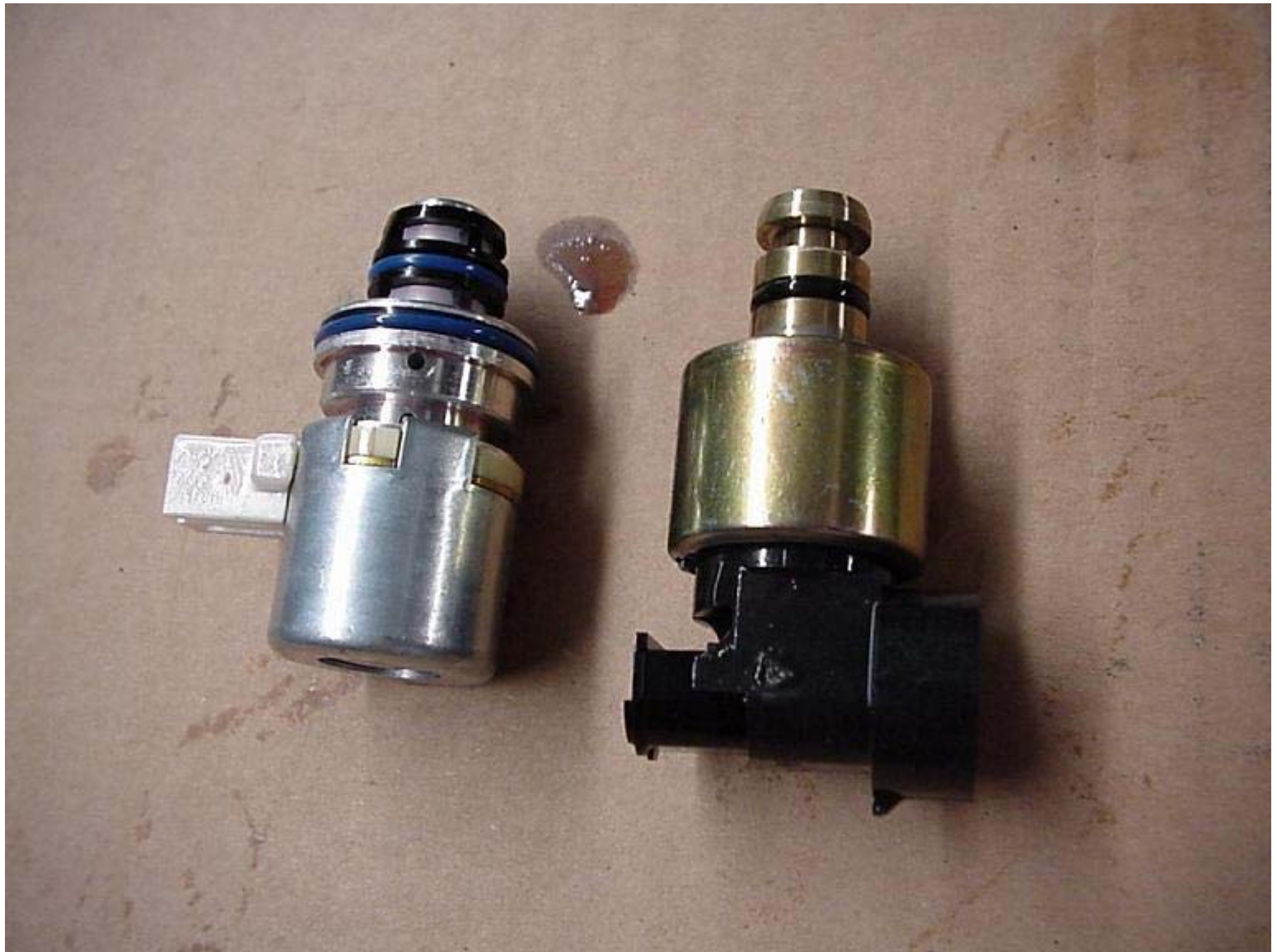
The solenoid is on the left and sensor on the right. The solenoid is backwardly compatible in all versions of the
