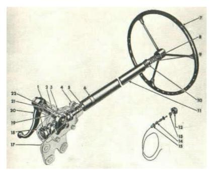
FIG. 31--STEERING GEAR
