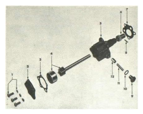
FIG. 11—OIL PUMP 1—Cover Screw 2—Cover 3—Cover Gasket 4—Outer Rotor 5—Shaft and Rotor 6—Body 7—Driven Gear 8—Gasket 9—Gear Retaining Pin 10—Relief Valve Retainer 11—Relief Valve Retainer, Gasket 12—Relief Valve Ppring 13—Relief Valve Plunger
