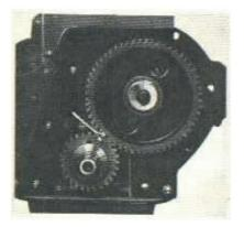
FIG. 8-TIMING GEAR MARKS
