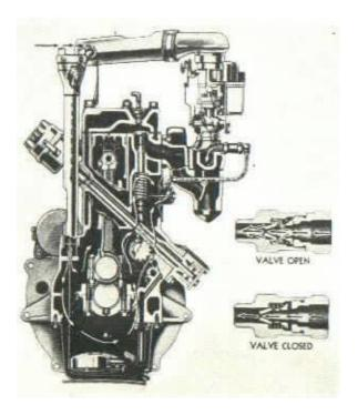
FIG. 12—CRANKCASE VENTILATING SYSTEM
