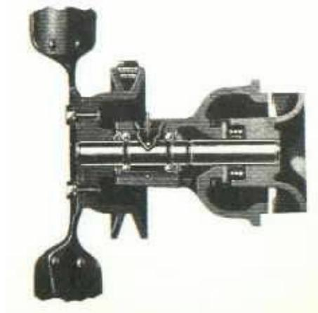
FIG. 15 —WATER PUMP ASSEMBLY
