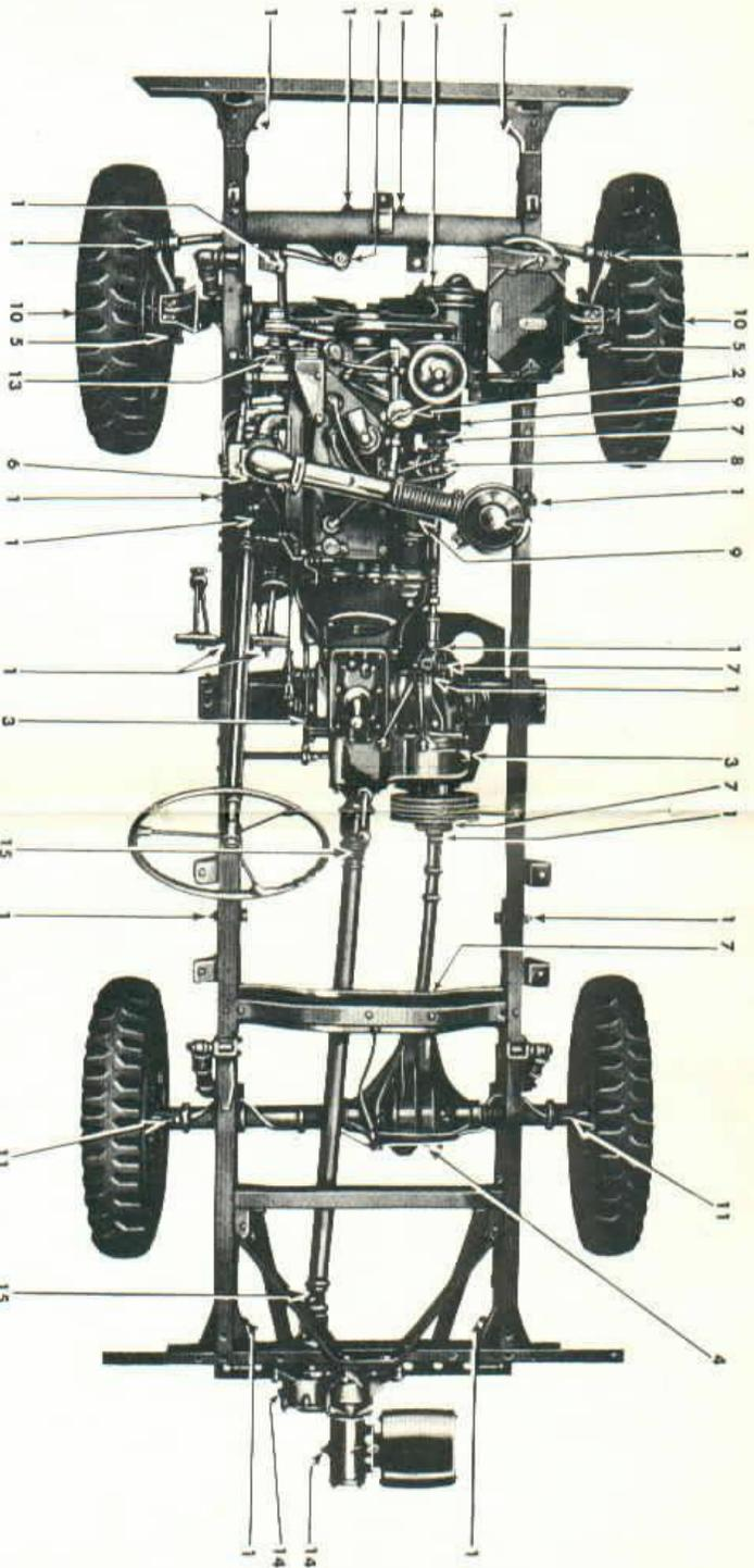
FIG. 20—CHASSIS, SHOWING PARTS REQUIRING LUBRICATION
