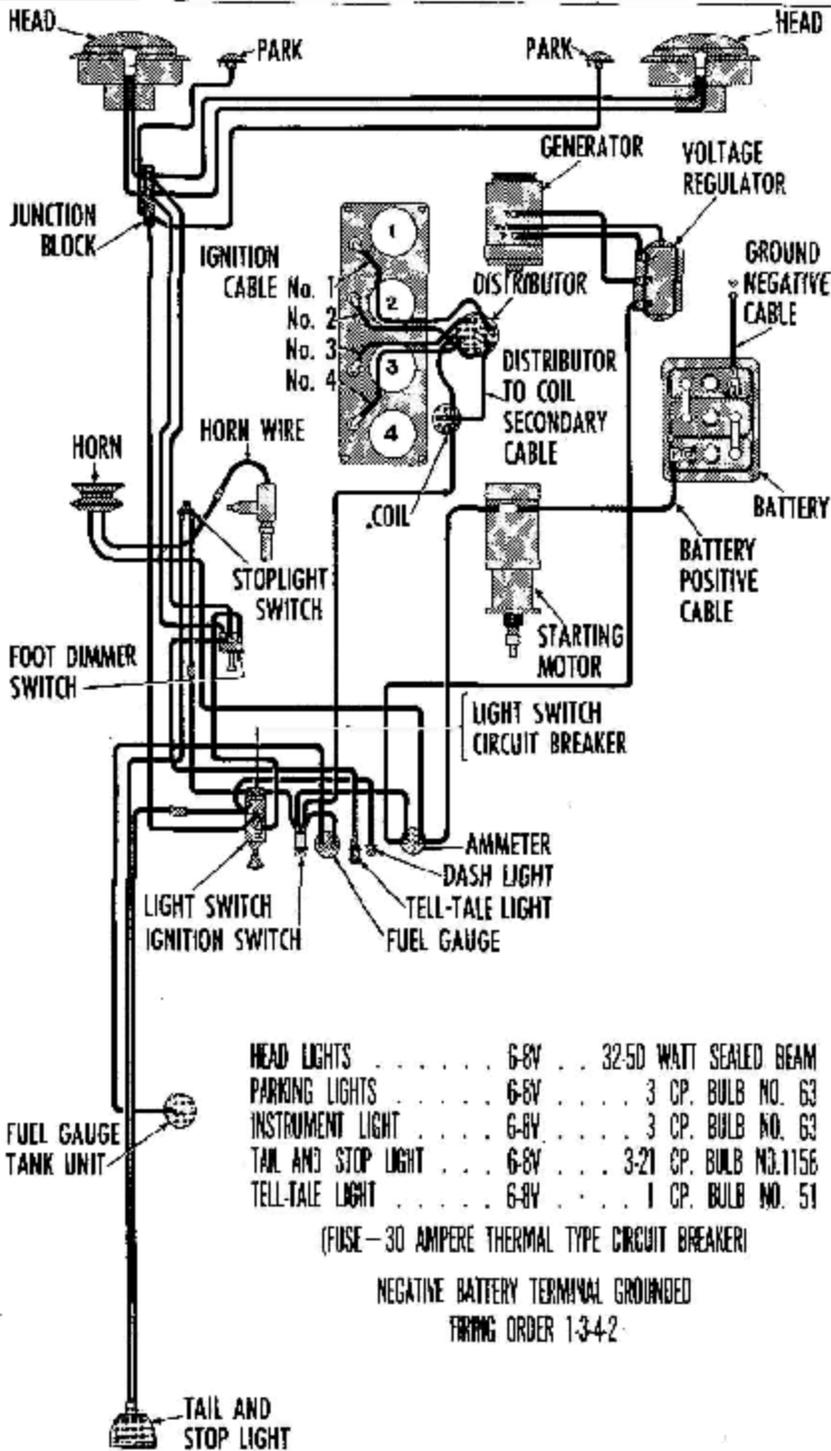
FIG. 16 -WIRING DIAGRAM
