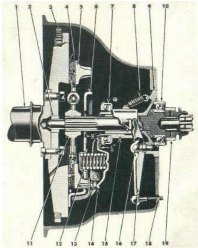
**FIG. 21 CLUTCH ASSEMBLY**
