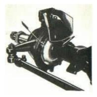
FIG. 5-KNUCKLE OIL SEAL
