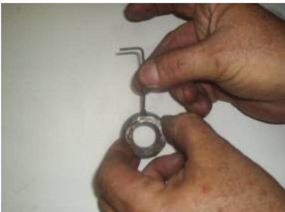
DETALHE DO PARAFUSO ALLEN DE TRAVA MONTADO NA LATERAL DA PORCA
