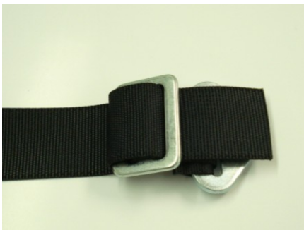
Figure 3d: Lock Down the 3-Bar. Make sure to leave lace the free end of the webbing back through the 3-bar to lock it down. Leave about 2-3" of webbing after the 3-bar.
