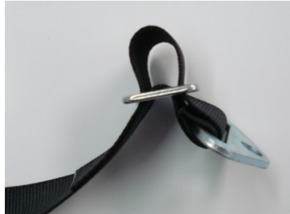
Figure 3b: Place the anchor as close as possible to the 3-bar to reduce slipping. Lace the free end of the webbing through both sides of the 3-Bar.
