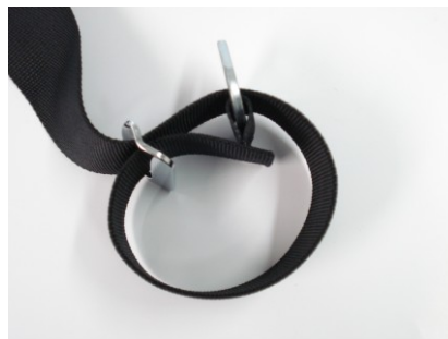
Figure 4b: Lace the webbing over the top of the 2-bar and back into the middle of the webbing loop.
