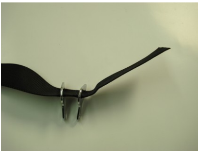
Figure 5a: Initial Lacing of the two anchors. Lace the webbing through both tongues.
