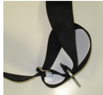
Figure 4c: Continue to lace the free end of the webbing through the top side of the anchor.
