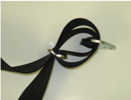
Figure 4d: The free end of the webbing then routes through the 2-bar in the middle of the two pieces of webbing already there.
