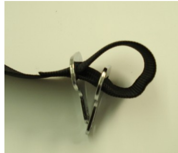
Figure 5b: Bring the free end of the webbing back through ONE of the anchors.
