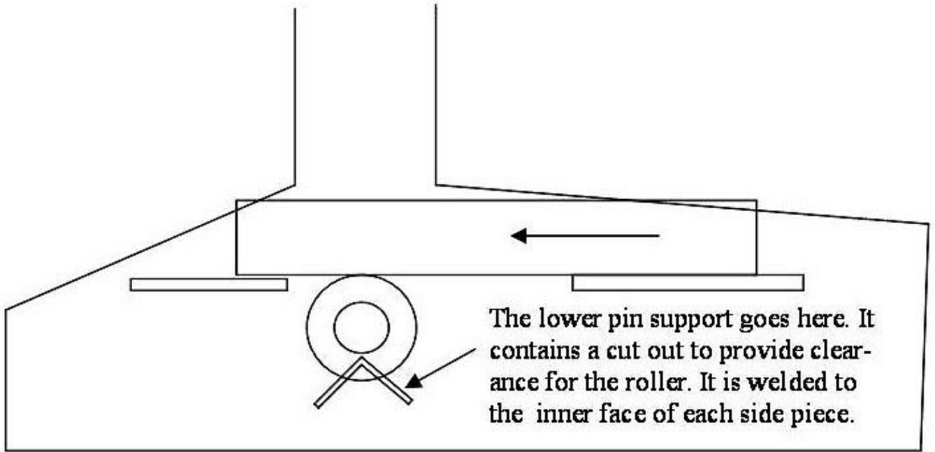
The ends of this angle support the lower pin. It is notched to allow clearance for the roller
