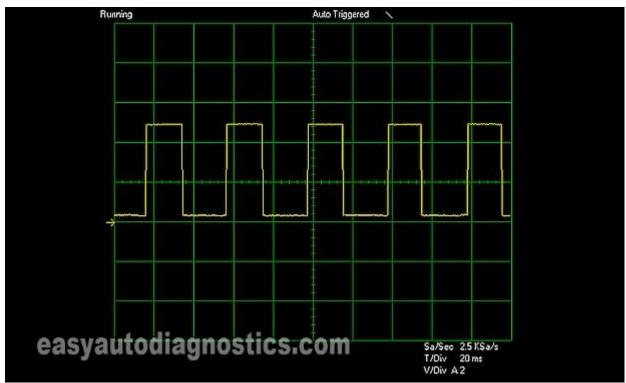
If you have access to an oscilloscope, this is what the mass air flow (MAF) sensor waveform looks like at idle.
