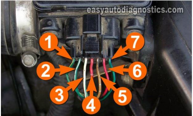
The last part of the Mitsubishi volume air flow sensor (mass air flow sensor) is the verify that it's producing a Reset Signal the Fuel Injection Computer can use. This is just an On/Off type DC voltage signal that turns 'On' when the throttle opens and turns 'Off' when the throttle closes.
