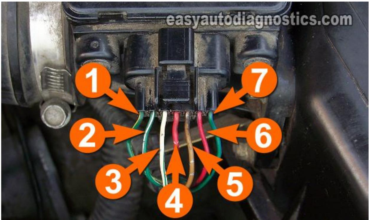
The last part of the Mitsubishi volume air flow sensor (mass air flow sensor) is to verify that it's producing a Reset Signal the Fuel Injection Computer can use. This is just an On/Off type DC voltage signal that turns 'On' when the throttle opens and turns 'Off' when the throttle closes.
