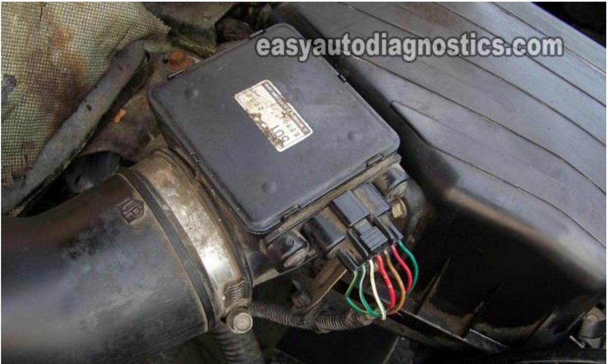
The mass air flow sensor on your Mitsubishi vehicle (or Chrysler Sebring or Dodge Stratus) can be tested without a scan tool and in 4 easy steps. All you'll need is a digital multimeter that can read Hertz frequency.
