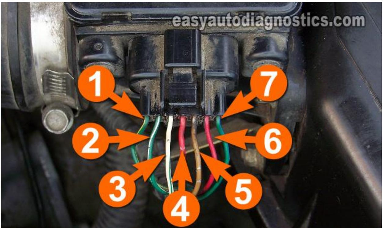
This Mitsubishi mass air flow (MAF) sensor has a total of 7 wires coming out of the connector. Although you won't be testing every single circuit, I've included the Circuit Descriptions of all them anyway for your viewing pleasure.
