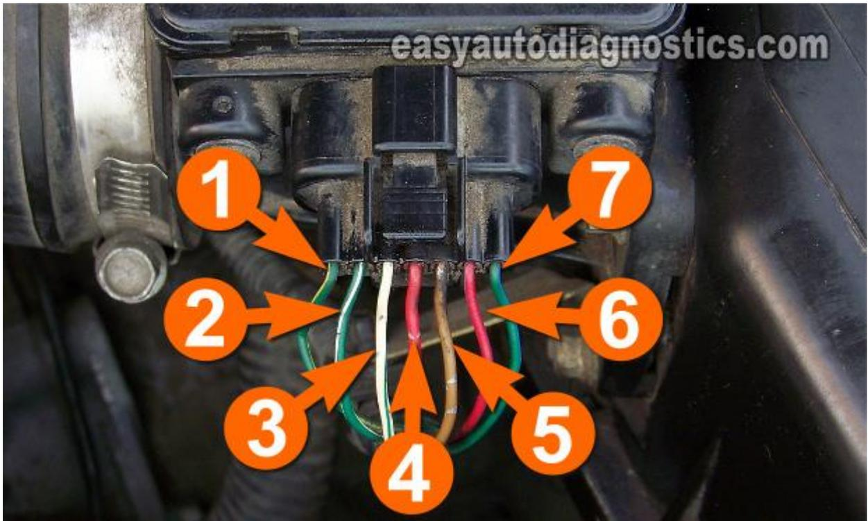
Testing the ground circuit follows pretty much the same procedure as the test steps for testing the power circuit. One word of caution... this ground is provided internally by the PCM, so you have to be careful NOT to short this circuit to power (12 Volts) or you'll damage the PCM. OK, here are the steps:
