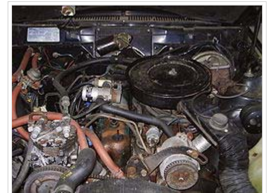
Engine bay of a 1980 AMC Spirit AMX with numerous emissions controls
