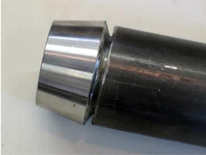
Figure 12 – Evolution threaded tube insert in 1.75" ID tube
