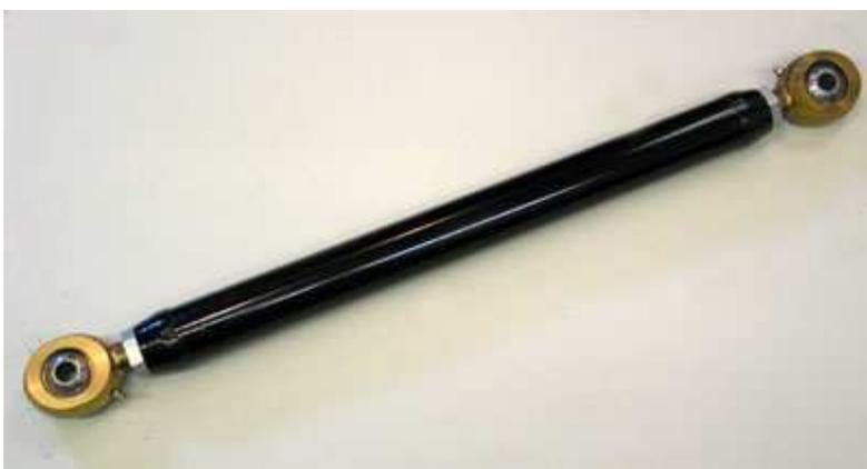
Figure 16 – Link frontal ajustavel usando Evolution Joints e 2.25 X 1/4" DOM
