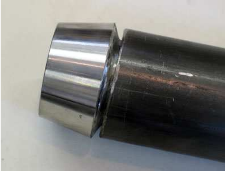
Figure 12 – Evolution threaded tube insert in 1.75" ID tube
