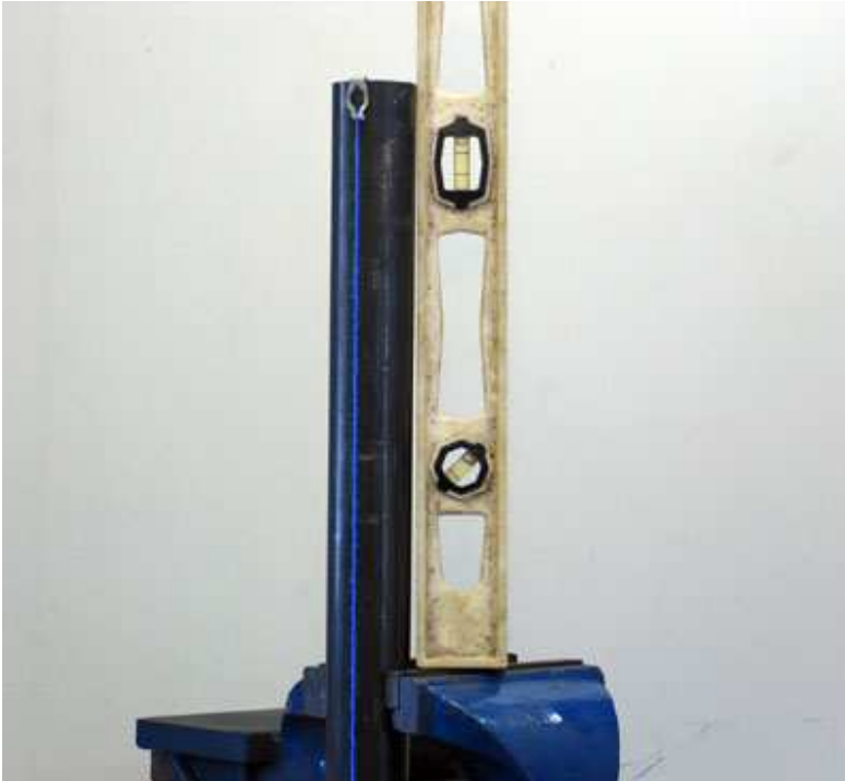
Figure 1 – Using a level and plumb-line to mark tube centerline
