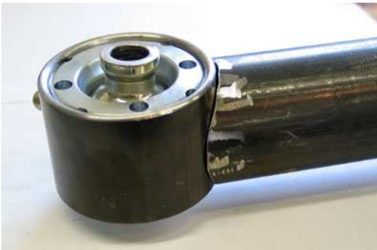
Figure 11 – 2” tube being test fit with RE bearing
