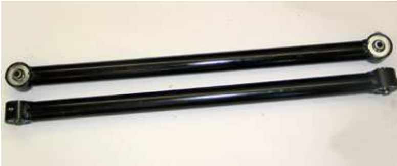
Figure 14 – Fixed length lower front links using RE bearings and 2" x 3/8" DOM
