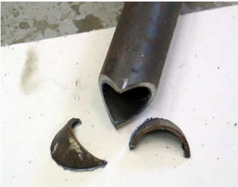
Figure 7 – Chop saw notch cut at 45°
