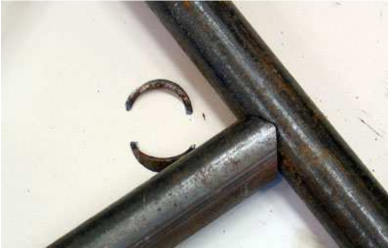
Fig 8 – Test fitting the notch
