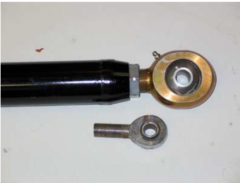
Figure 15 – Completed link with Evolution Joint shown next to standard 3/4" Heim joint for scale.
