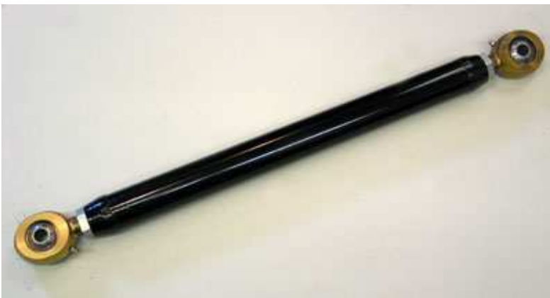
Figure 16 – Adjustable top front link using Evolution Joints and 2.25 X 1/4" DOM
