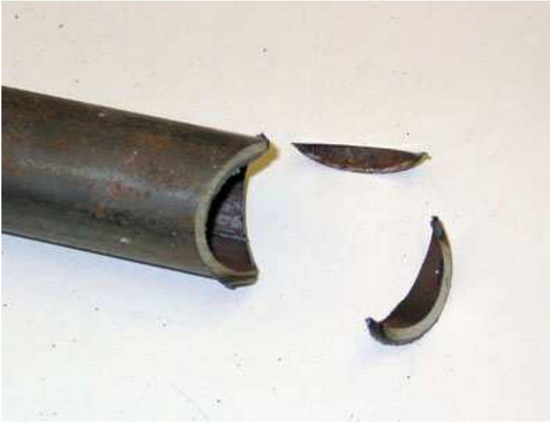
Figure 6 – Completed chop saw notch cut at 30°
