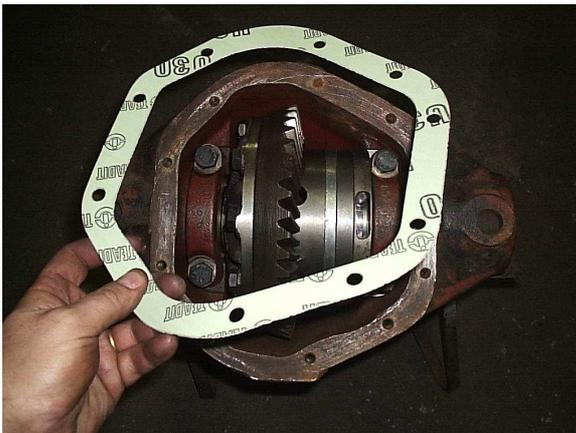
COLOQUE A JUNTA DA TAMPA
