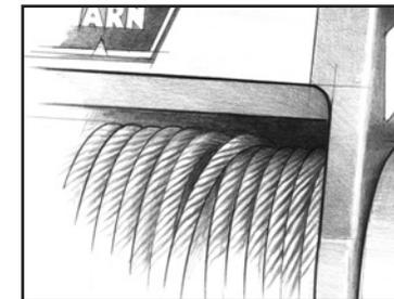
**Step 11: CHECK WIRE ROPE.** The wire rope should be neatly wound around the spooling drum. Improper winding can cause damage to the wire rope.
