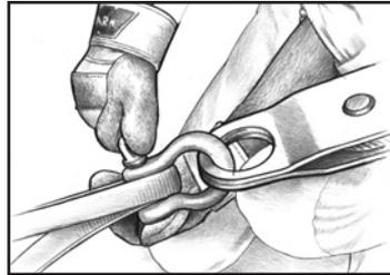
careful not to over tighten (tighten and back-off 1/2 turn).
