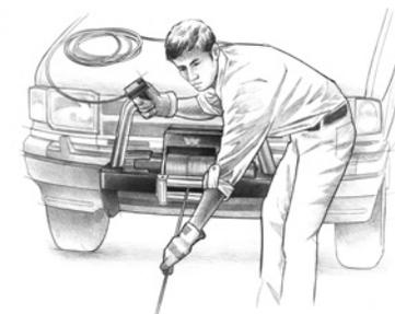
**Step 9: PUT WIRE ROPE UNDER TENSION.** Using the winch switch, slowly wind the wire rope until no slack remains. Once the wire rope is under tension, stand well clear, and never step over it.
