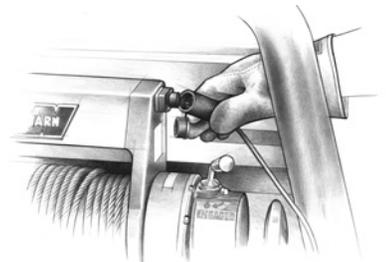
**Step 19: DISCONNECT REMOTE CONTROL.** Disconnect the remote control cord from the control box and store in a clean and dry place. Winching operations are now complete. Put the cap on the solenoid plug in.
