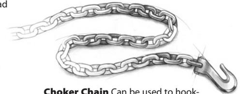
**Choker Chain** Can be used to hook-up to another vehicle or sharp objects for an anchor point. Chains, however, will damage or kill trees.
