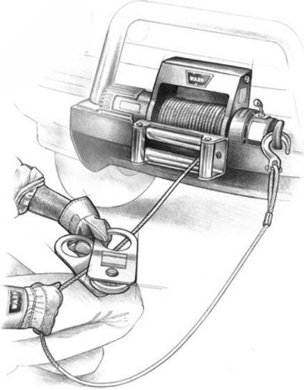
Disengage the clutch and, using the snatch block, pull out enough wire to reach your anchor point. Do not attach hook to mounting kit.
