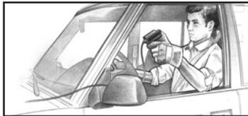
**Step 14: BEGIN WINCHING.** With the winching vehicle's engine on and light tension already on the wire rope, begin winching slowly and steadily. Be sure that the wire rope is winding evenly and tightly around the spooling drum. For additional assistance, the winched vehicle can be slowly driven while being pulled by the winch.
