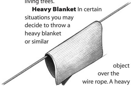
object over the wire rope. A heavy blanket, such as a quilted mover's blanket, can absorb energy should the wire rope break. Place it on the wire rope midway between the winch and the anchor point. Do this before the wire rope is put under tension. Do not approach or move the blanket once tension is applied. Do not allow it to get pulled into the fairlead. If necessary to move or remove the blanket, slack the tension on the wire rope first.
