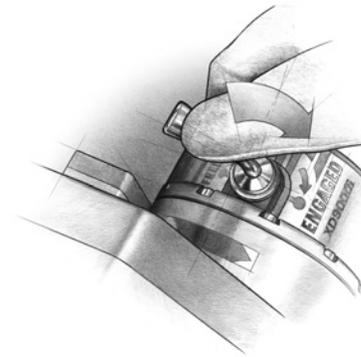
**Step 7: LOCK THE CLUTCH.** Lock the winch drum by rotating the clutch lever on the winch to Engage.
