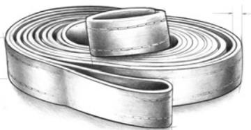
**Recovery Strap** Never use a recovery strap in a winching operation. Because it is designed to stretch, it stores energy and could react like a rubber band should your rigging fail. Use the recovery strap to "snatch" out a stuck vehicle.
