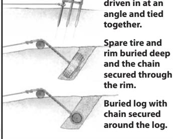
Stakes or axles, driven in at an angle and tied together.
