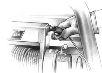
**Step 8: CONNECT THE REMOTE CONTROL.** Be careful not to let the remote control cord dangle in front of the winch. If you choose to control the winch from inside your vehicle, always pass the remote through a window to avoid pinching the cord in the door. **Always disconnect the remote control when not in use.**
