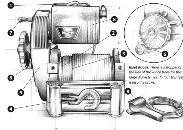
*Inset above: There is a stopper on the side of the winch body for this large diameter reel. In fact, this reel is also the brake.*
