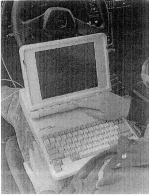
Fig. 7-22. The laptop computer is a basic tool for creating and tuning fuel curves of aftermarket fuel injection systems.
