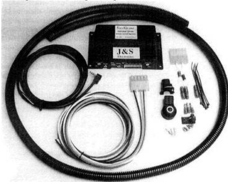
Fig. 9-4. A native knock-detection system with control of ignition timing is an excellent means of establishing a margin of safety for an engine. These items often add power as well as safety, by permitting ignition timing to stay closer to the knock threshold than is possible when tuning by ear.
