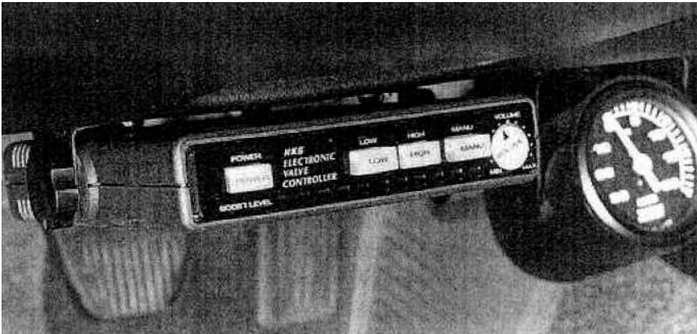
Fig. 12-20. The HKS Electronic Valve Controller is a multilevel boost-change device that also produces faster boost rise by blocking the signal to the wastegate until near-maximum boost is achieved.
