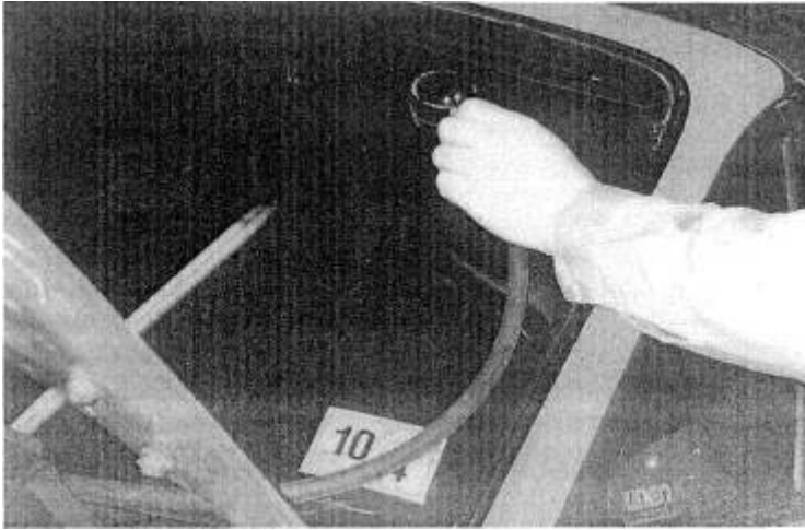
Fig. 18-24. For reasons of safety, the fuel pressure gauge, which is needed to complete the tuning process, should not be placed inside the cockpit. Tape the gauge to the outside of the windshield at a convenient location for viewing while driving.
