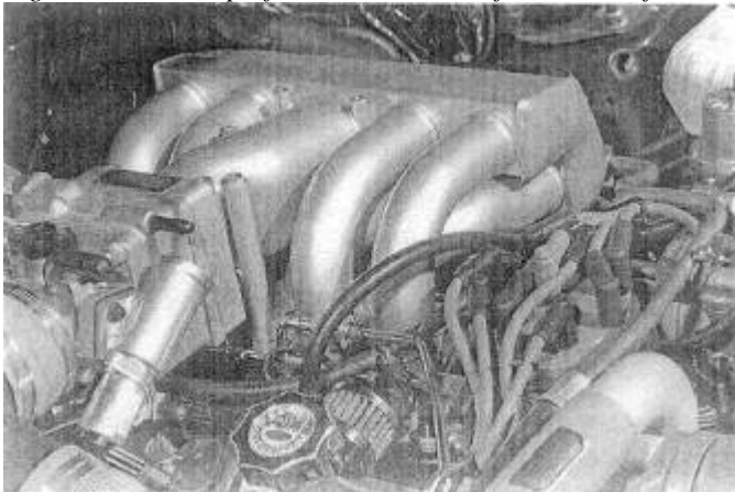
Fig. 6-6. Individual intake runners from a plenum are useful design features. A good example of a symmetrical design.
