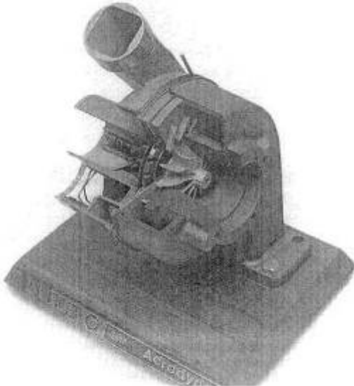
Fig. 16-4. The fastest-response turbo in the world is the VATN Aerocharger.
