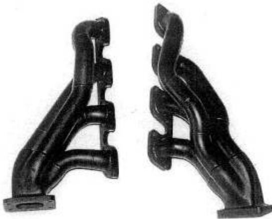
Fig. 10-5. Four-into-one designs for 4- or 8-cylinder engines
