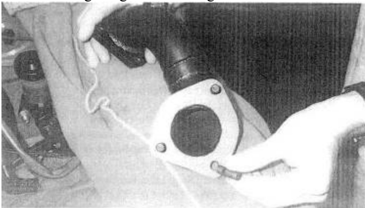
Fig. 18-8. Preparation of the turbine outlet pipe is limited to installation of the studs needed to fasten to the stock Miata exhaust header pipe.
