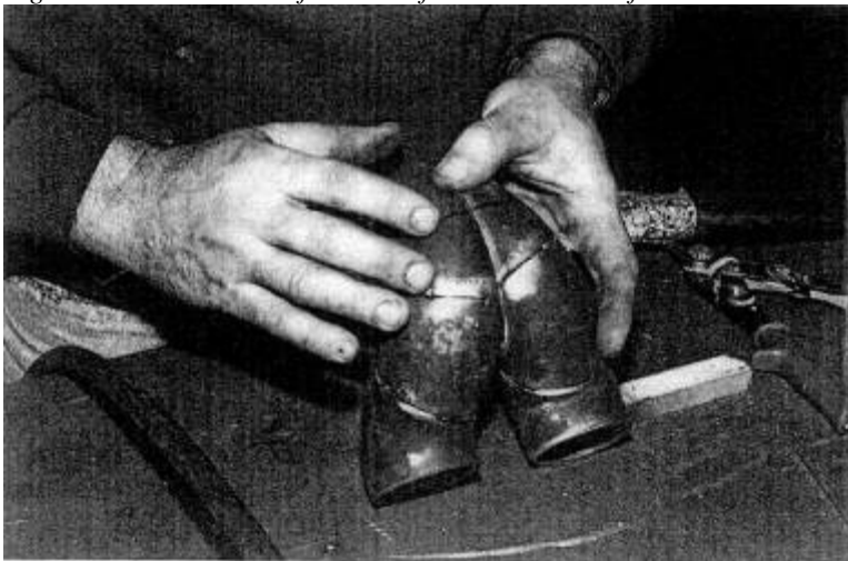
Fig. 10-11. Fitting weld els together to form the triple-turbo Jaguar exhaust manifolds
