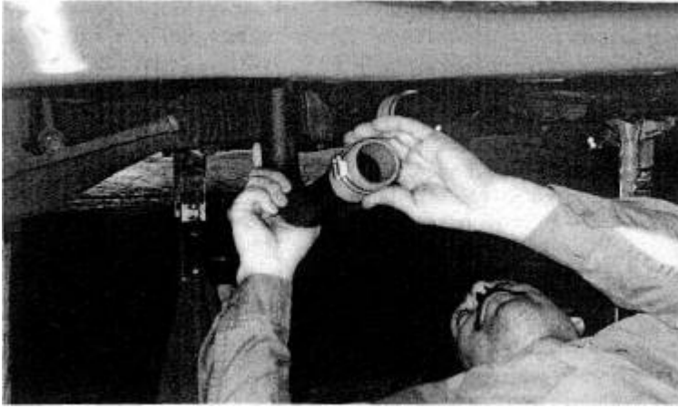
Fig. 18-17. With the turbo and intercooler in position, the interconnecting tubes can be installed.
