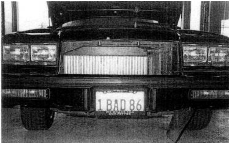
Fig. 5-2. The front mounted intercooler is a typical aftermarket replacement for the Buick GN/GNX series cars.
