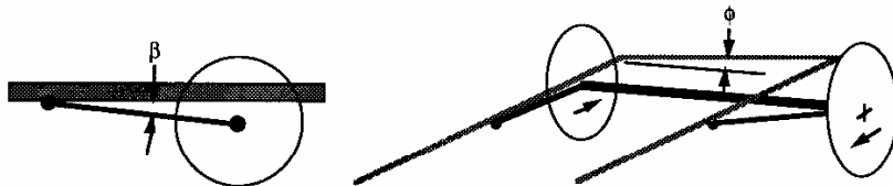
Fig. 6.16 Roll steer with a solid axle.
