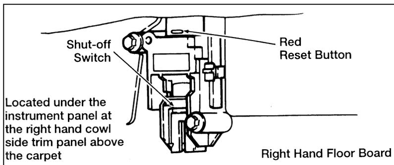
*Fuel pump shut-off switch location*
