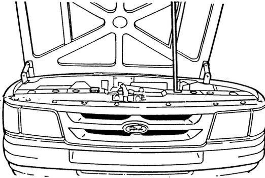
While applying upward pressure on the hood, lift the auxiliary latch release handle and raise the hood. Insert support rod in hood prop hole. To close, raise hood slightly and remove support rod from the prop hole. Slam hood shut. After closing, always make sure your hood is latched securely by trying to lift it.
