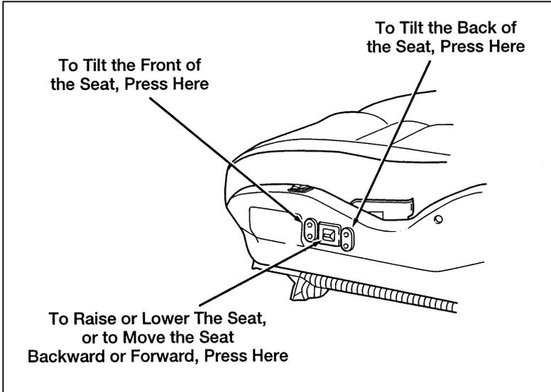
*The power controls on the driver's seat*
