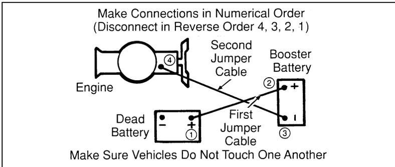
**Attaching jumper cables**
