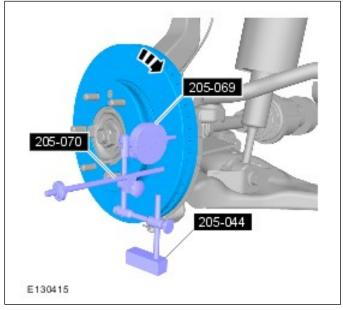
5. NOTE: If any of the measurements exceed the run out specification of 0.05 mm or the brake disc thickness variation is more than 0.018 mm, a new brake disc must be installed and the brake disc runout re-checked.
