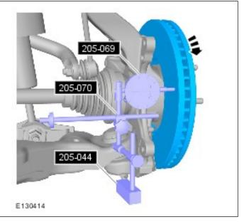
**4. NOTE:** The total dial indicator gauge reading should not exceed specification.
