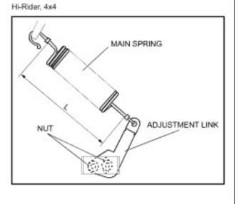
3. Adjust main spring dimension L between the LSPV and the adjustment link loosening and repositioning the LSPV.
