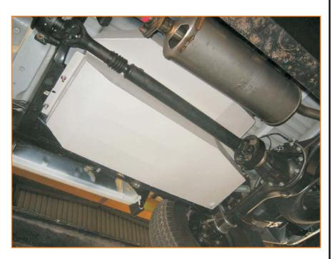
Stop when you want, not where your vehicle needs to. This replacement tank provides the user with a much needed boost in driving range thanks to an 80% increase over the standard 70lt tank. Ground clearance is actually improved, helping with the all
