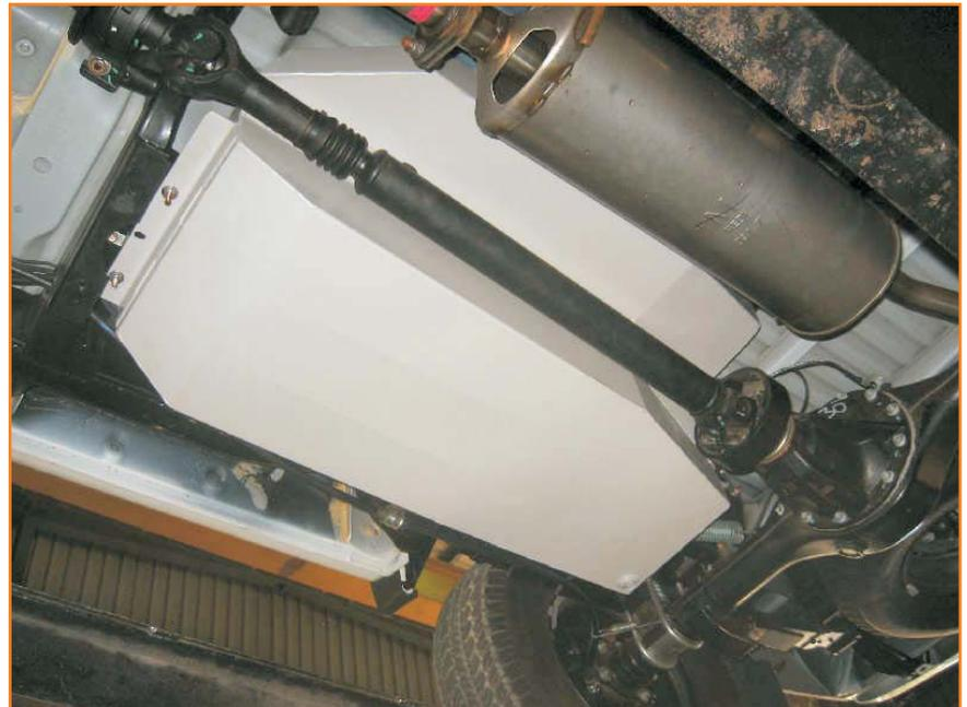
Stop when you want, not where your vehicle needs to. This replacement tank provides the user with a much needed boost in driving range thanks to an 80% increase over the standard 70lt tank. Ground clearance is actually improved, helping with the all important ramp over angle.
